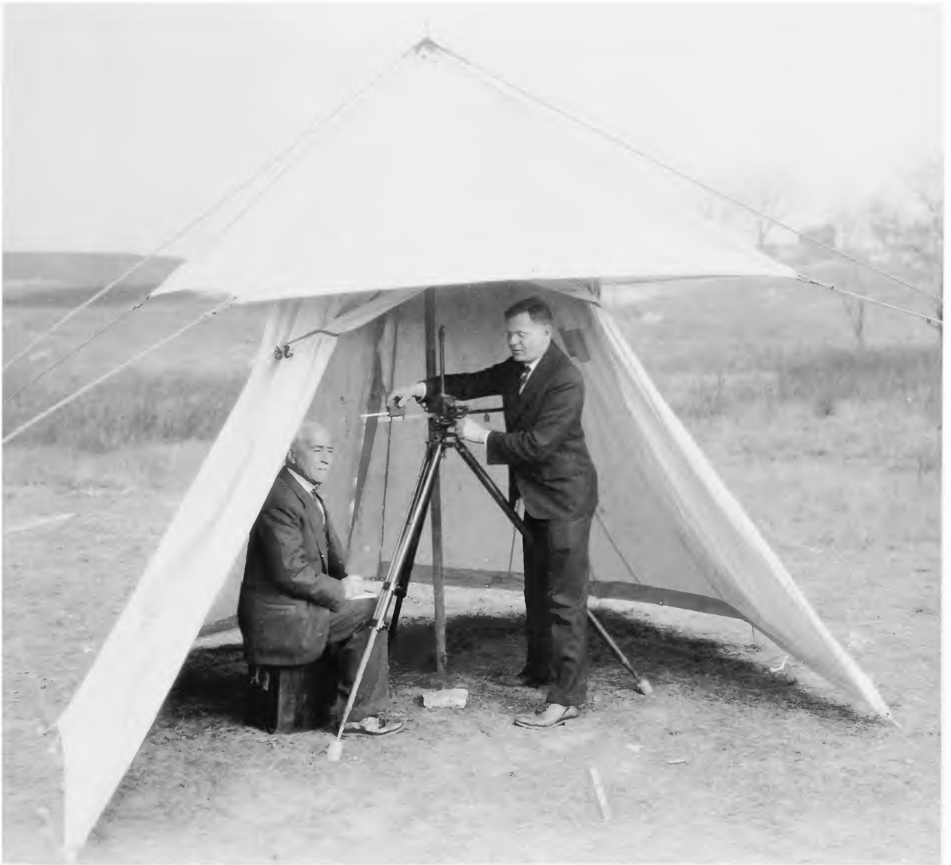
FIGURE 49.—Observation of horizontal intensity, with a magnetometer that is similar to No. 19 (Figure 48), November 1930. R.R. Bodle, standing; W.M. Hill, recording.
