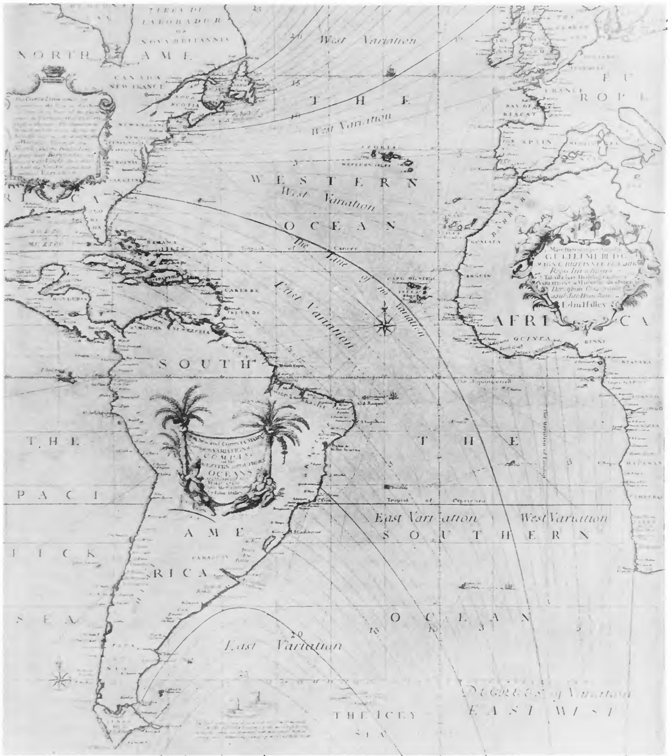
FIGURE 5.—“Chart of the lines of equal magnetic variation,” by Edmund Halley, 1701. (Reprinted from TM, 1 (1896).)
