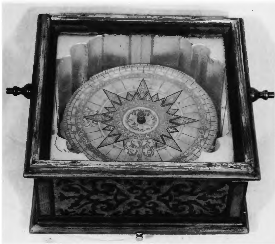
FIGURE 1.—Navigational compass, 15th century, Portuguese, a typical instrument in which a magnetized needle is fixed to the underside of a circular card on which the directions are laid out. (Copy, in the Smithsonian Institution, of an original in the Museum of the History of Science, Cambridge University.)
