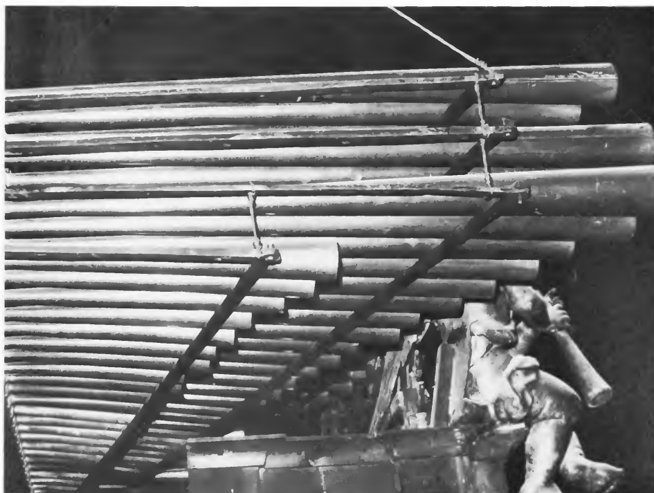
FIGURES 12, 13.—Epistle organ, Chamade reed registers: 12 (above), before the restoration of 1975–1978, showing extensive fire damage; 13 (below), after the restoration of 1975–1978. Ranks (top to bottom) are Trompa Magna (treble), Orlo (bass), Bajoncillo (bass), and Clarin en Quincena (bass).
