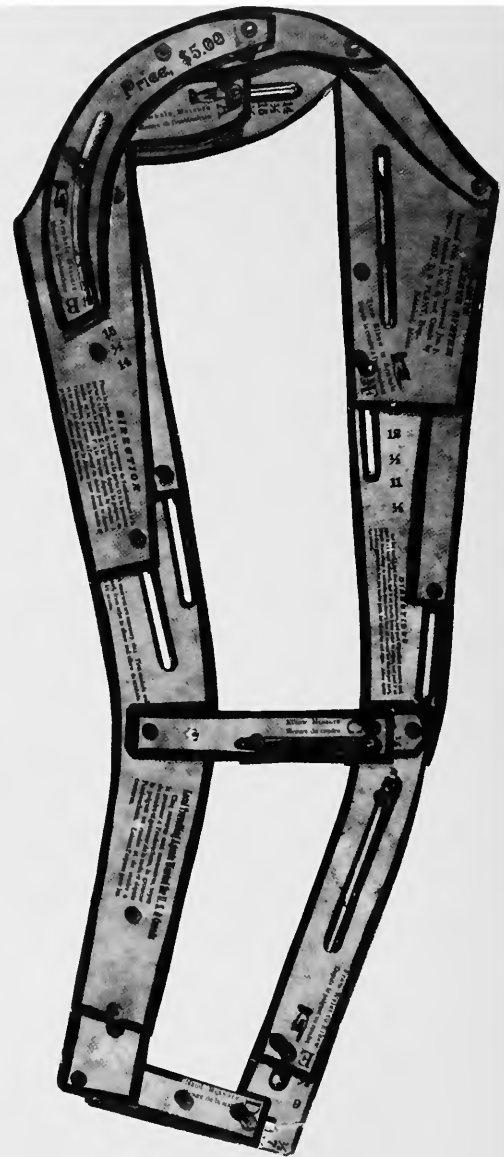
FIGURE 26. Adjustable cardboard tool for Plant's direct-measure system of drafting sleeves, which could be added to the dress cutting system for an additional $5. (Smithsonian Institution.)
