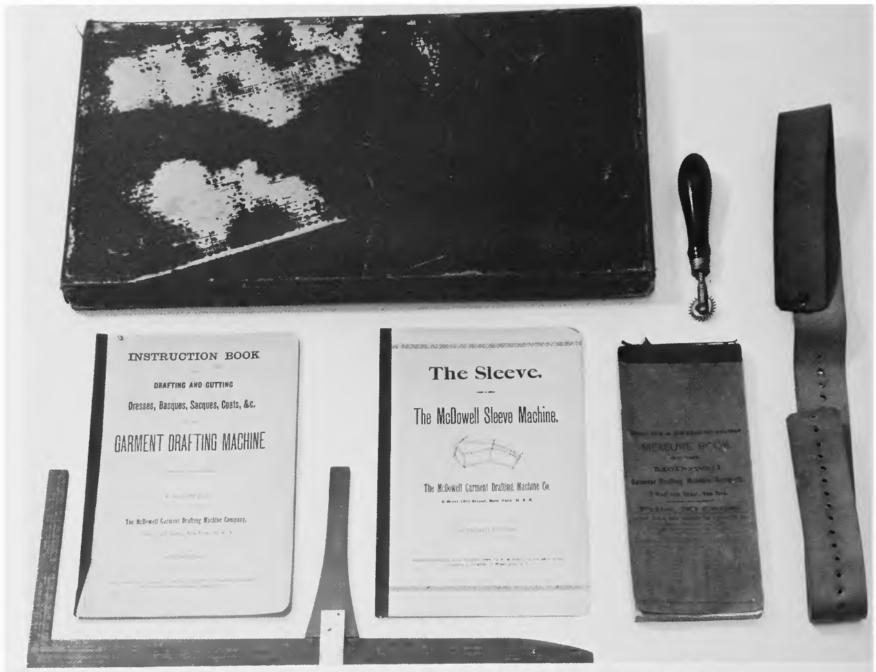
FIGURE 43d. Accessories for the McDowell machines: cardboard box, tracing wheel, instruction books for the two machines, measure book, leather belt used as a guide for taking measurements, and obsolete "McDowell Garment Drafting Square" with sliding arm or gauge used to take some measurements. The majority of individuals listed in the measure book were Duncans living in Brooklyn, New York.
