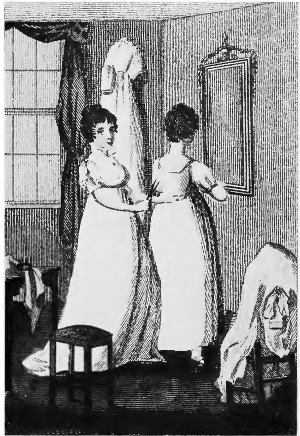
FIGURE 11. Cutting a dress according to the pin-to-the-form technique, from Tabart & Co., The Book of Trades , London, 1804. (Library of Congress.)
