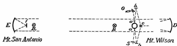
FIGURE 1.—Arrangement of Michelson apparatus. (From A. A. Michelson, "Measurement of the Velocity of Light between Mount Wilson and Mount San Antonio," The Astrophysical Journal , volume 65 (1927), page 4.)
