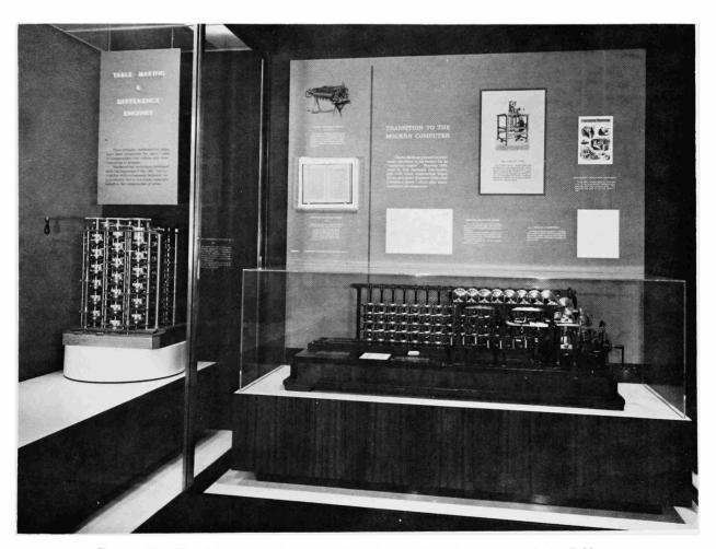
FIGURE 27.—The Scheutz calculator (right) and a replica of a portion of the Babbage difference machine (left) in the National Museum of History and Technology, Smithsonian Institution. (SI photo X4723)
