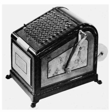
FIGURE 25.—Burroughs full keyboard adding machine of the 1890s. (SI photo 58996G; NMHT 292398)
