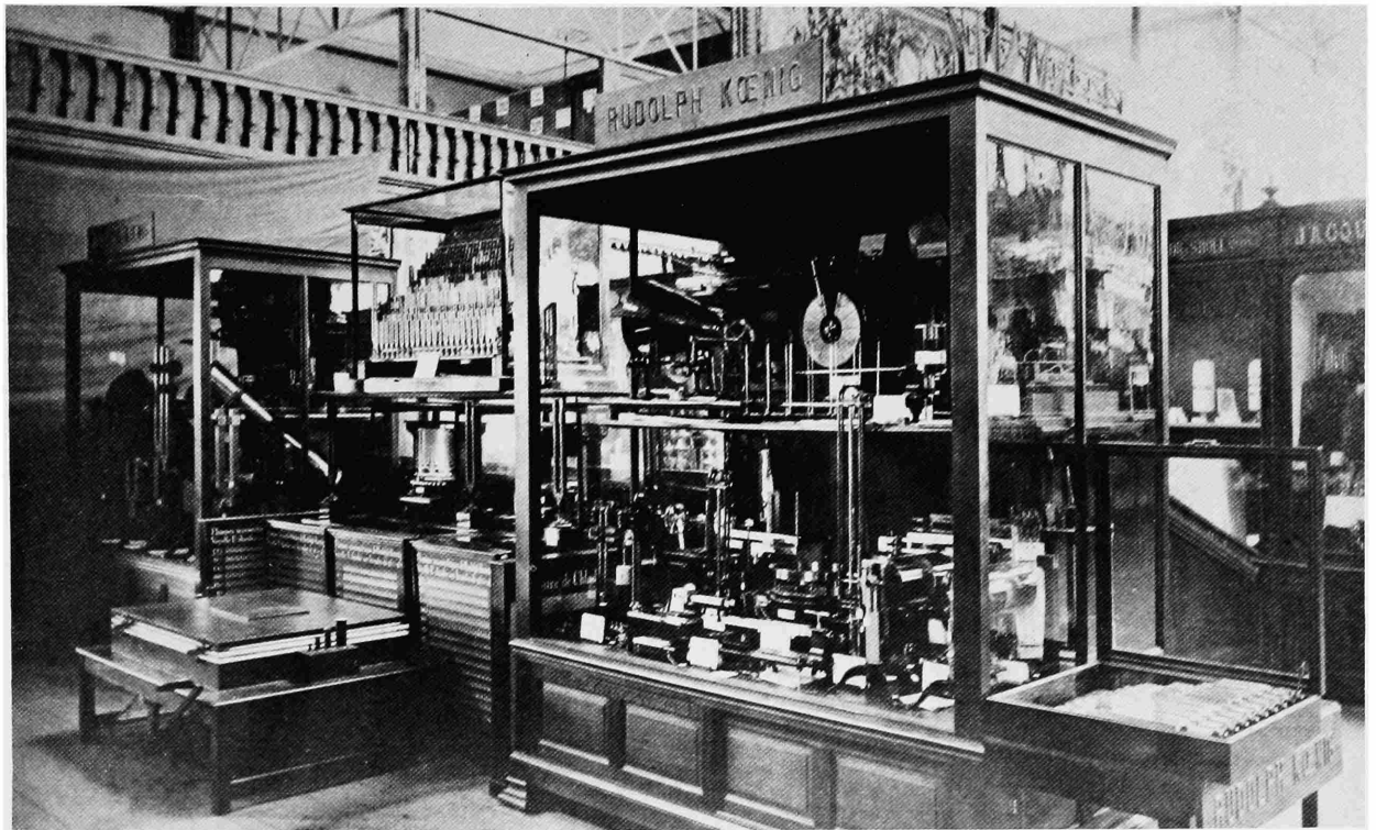
FIGURE 2.—R. Koenig's acoustic apparatus at the International "Centennial" Exhibition in Philadelphia in 1876. Note the large forks in the case on the left, the tonometer and the siren "telephone" in the center case. (SI photo 74-3810-10)
