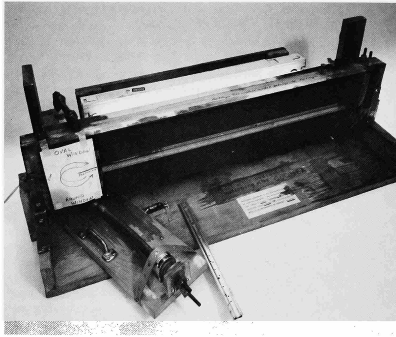
FIGURE 28.—Hydraulic model of the cochlea constructed by Max Meyer in 1964, after one built in 1928. Wooden frame 863 \times 165 \times 63 mm. (SI photo 72-11336; USNMHT 259279.01)
