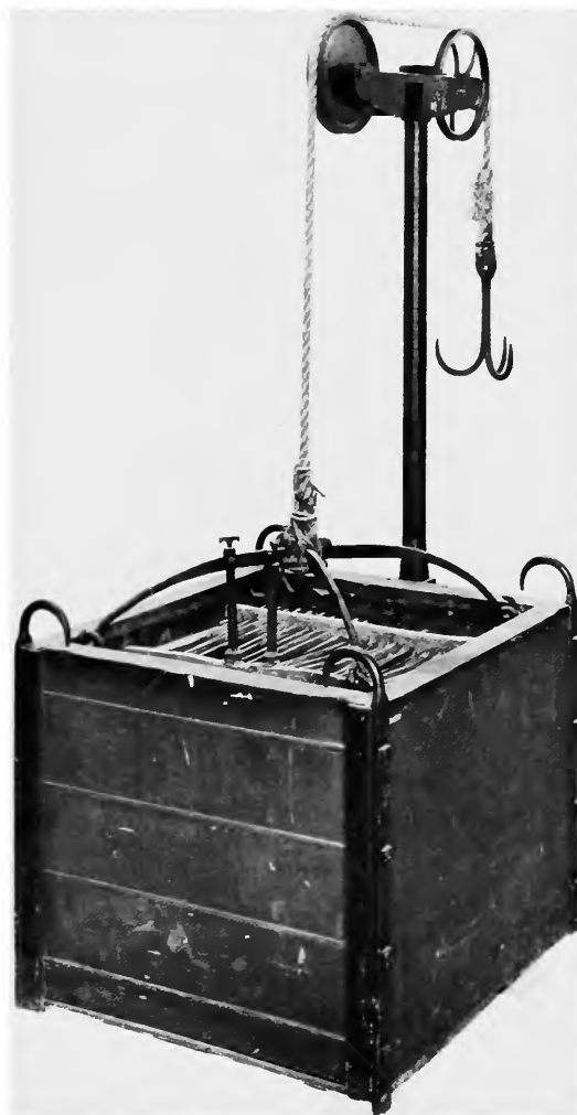
Figure 12. —ROBERT HARE'S CALORIMOTOR. This plunge-type galvanic battery, part of a collection deposited by Hare in the nascent Smithsonian Institution in 1847 following his retirement, was among the earliest specimens of "philosophical apparatus" secured by Joseph Henry for that national institution. Substantially similar to the calorimotor that Hare had described in the American Journal of Science and Arts in 1819, this galvanic device was notable in that all copper plates were connected and all zinc plates were similarly connected, thus in effect creating one large pair of electrodes, "instead of multiplying the pairs of galvanic plates." Like earlier plunge-type batteries devised by William Pepsy, C.H. Wilkinson, and Humphry Davy in England, Hare's calorimotor had the advantage of limiting corrosion of the plates to the period of actual immersion in the electrolyte. Its subsequent employment by Hare for rock blasting during 1831-33 received substantial attention in American scientific circles.
