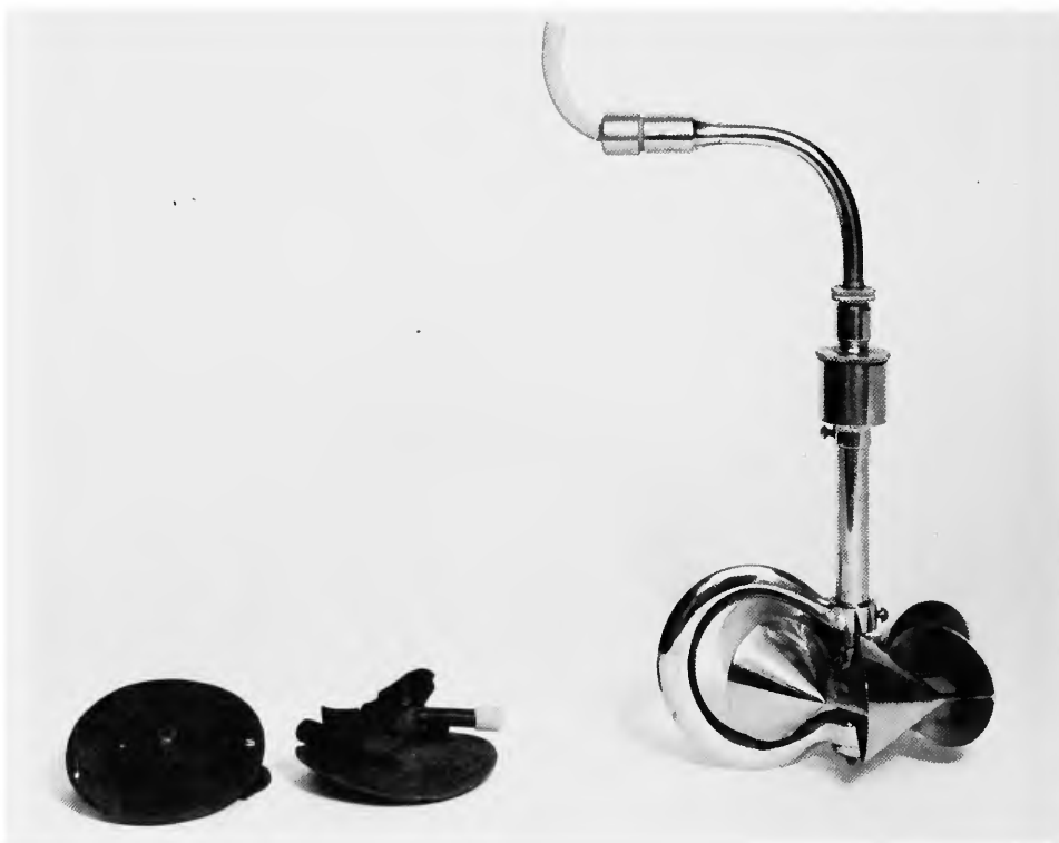
FIGURE 89.—Price's "acoustic current meter," ca. 1895, without brass suspension rods. (NMHT 316594, Smithsonian photo 72243.)
