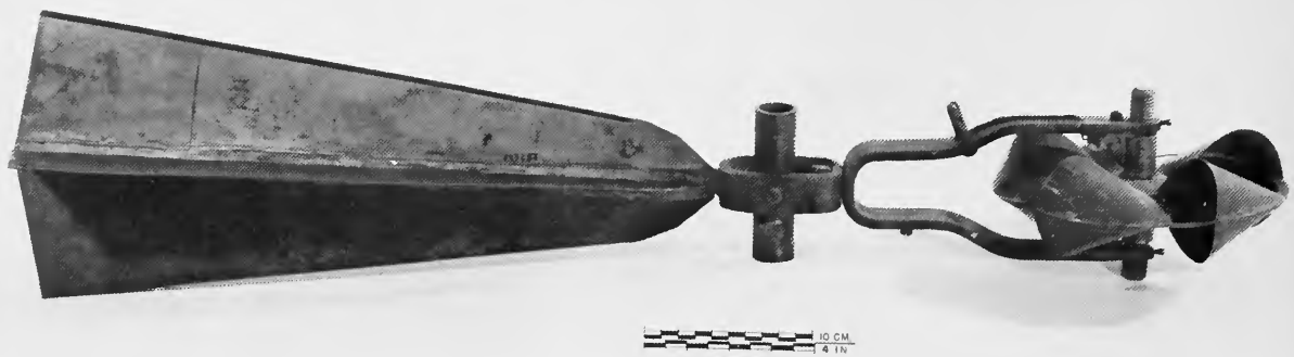
FIGURE 85.—The original Price current meter, built by him and four mechanics at Paducah, Kentucky, in 1882. (NMHT 289638, Smithsonian photo 44538-H.)
