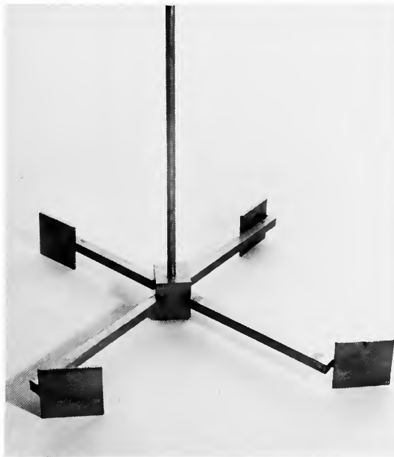
FIGURE 42.—Replica of De Saumarez' rotor, which was used on his vertical-axis ships' log, ca. 1715. (NMHT 321481, Smithsonian photo 75593.)
