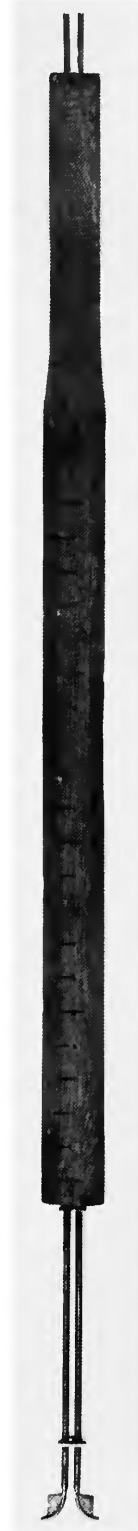
FIGURE 34.—A Pitot tube intended for use in hydraulic laboratories. This model was originally owned by the Proprietors of Locks and Canals of Lowell, Massachusetts. (NMHT 314776, Smithsonian photo 74335.)
