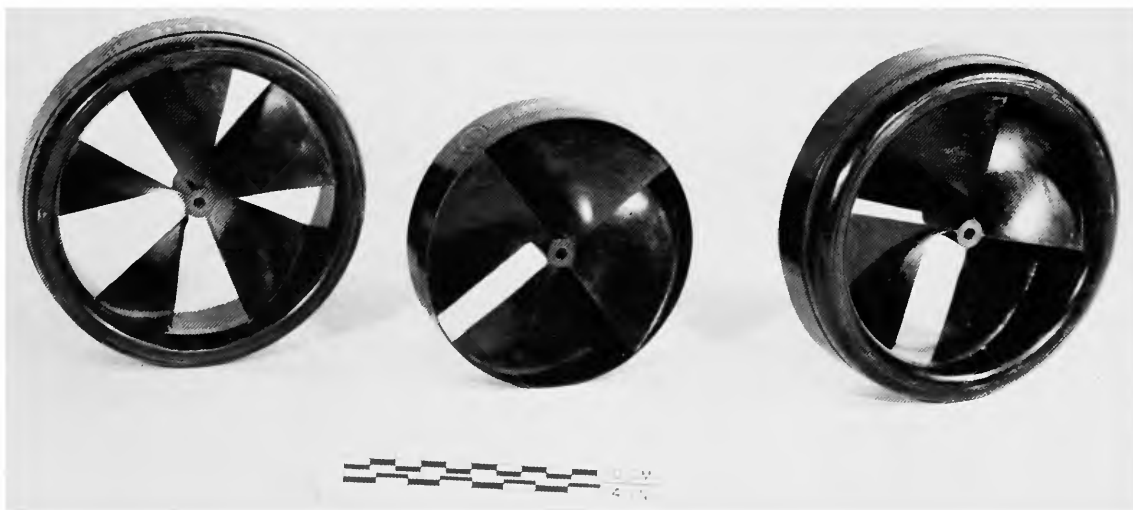
FIGURE 62.—Three experimental rotors manufactured by Buff and Berger, Boston, ca. 1876, for trial on the new "Herschel" meter, an American version of the Baumgarten meter (NMHT 314766, 314767, 314768; Smithsonian photo 44536-B.)
