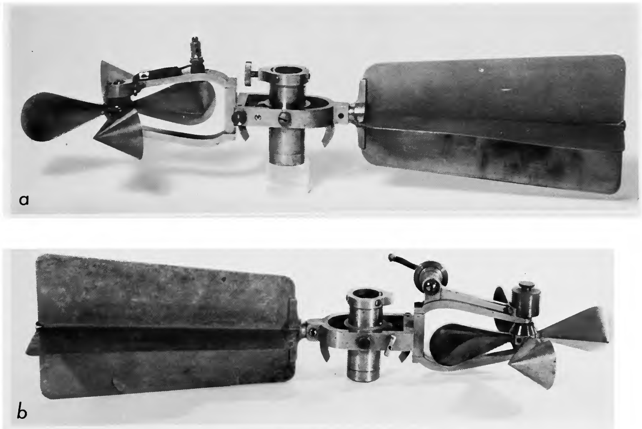
FIGURE 80.—Early Ellis current meters: a , as originally designed (NMHT 317669, Smithsonian photo 72257); b , with first improvement (NMHT 289637, Smithsonian photo 44538).
