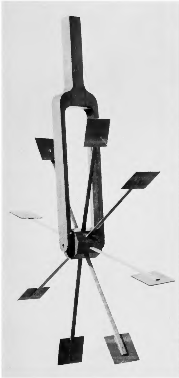
FIGURE 26.—Replica of Dubuat's "moulinet" for measuring the surface velocities of water in rivers and canals, ca. 1780. (NMHT 317672, photo by A. H. Frazier.)
