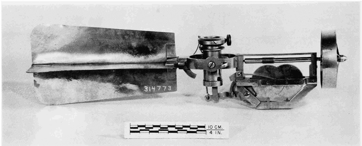
FIGURE 57.—Baumgarten's current meter, manufactured by Secretan of Paris, ca. 1846. (NMHT 314773, Smithsonian photo 44536.)
