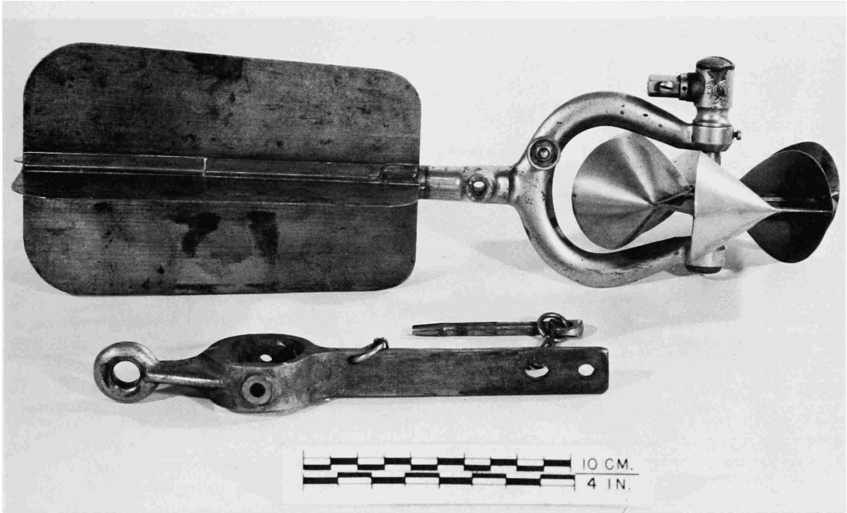
FIGURE 91.—One of the earliest Small Price current meters to be commercially manufactured, ca. 1897, by W. & L. E. Gurley. (NMHT 289644, Smithsonian photo 44538-F.)
