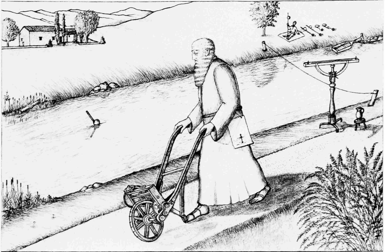
FIGURE 7.—Leonardo conducting experiments on the velocity-distribution in streams. (Drawn by A. H. Frazier.)
