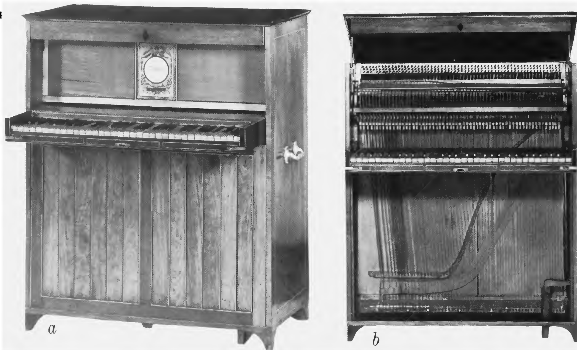
FIGURE 11. Upright piano (called portable grand) by John Isaac Hawkins, Philadelphia, 1801. Compass FF to f 3 . a , Full view. Two pedals or levers, which move from side to side—one to open and close the Venetian swell, the other a buff stop. The keyboard folds up, making a neat little portable cabinet. b , Plan view. (Catalog number 313,619; Hugo Worch Collection.)
