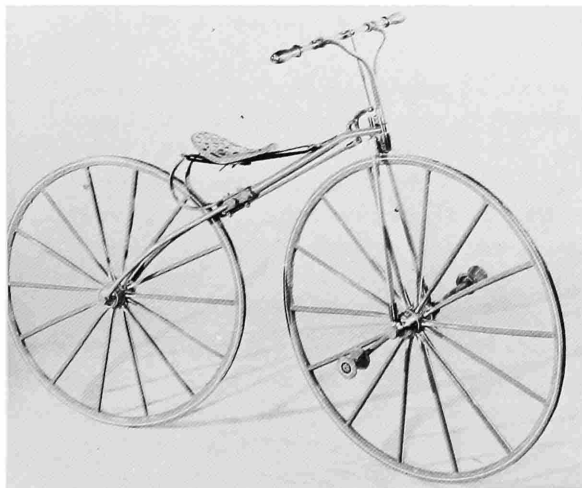
The Van Anden velocipede of 1869 has a free-wheeling device in the front hub that permits the rider to coast, as with a coaster brake.
