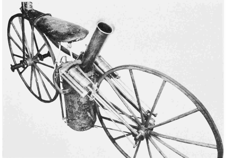
Steam velocipede built by Sylvester H. Roper about 1869. Below, arrangement of cylinders, valve chests, and the feed-water pump on the left cylinder.
