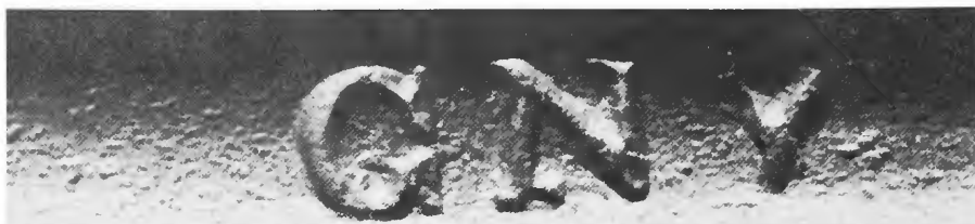
FIGURE 15.—Markings on copper bolts from contemporary ships: a, Gosport Navy Yard from Constellation ; b, Washington Navy Yard from Constellation ; c, from New Hampshire ; d, from Constitution ; e, from Constellation .
