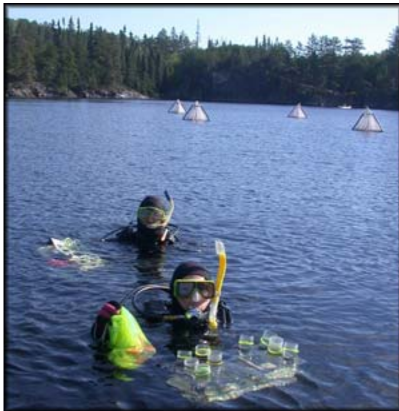
Divers sample the bottom sediments of Experimental Lake 658 to test for methylmercury produced from mercury isotopes added to lake water. An aim of the METAALICUS project is to understand how quickly mercury enters the food web.
