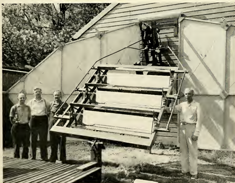
2. SOLAR BOILER FOR \frac{1}{2} HORSEPOWER ENGINE AS EXHIBITED TO INTERNATIONAL POWER CONGRESS AT WASHINGTON 1936
