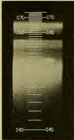
FIG. 1.—The wave length scale of the Abbe-Zeiss microspectroscope, with the absorption spectrum of "didymium" glass, the interval between the two strongest bands of which is set at 058. The several bands lie at 067.5, 062.5, 059.0, 058.2, 057.4, 053.1, 052.5, 051.2, 048.0, 044.8, and 043.3. Transmitted light; source, Welsbach burner; exposure 1 hour; Wratten and Wainwright Panchromatic plate.
