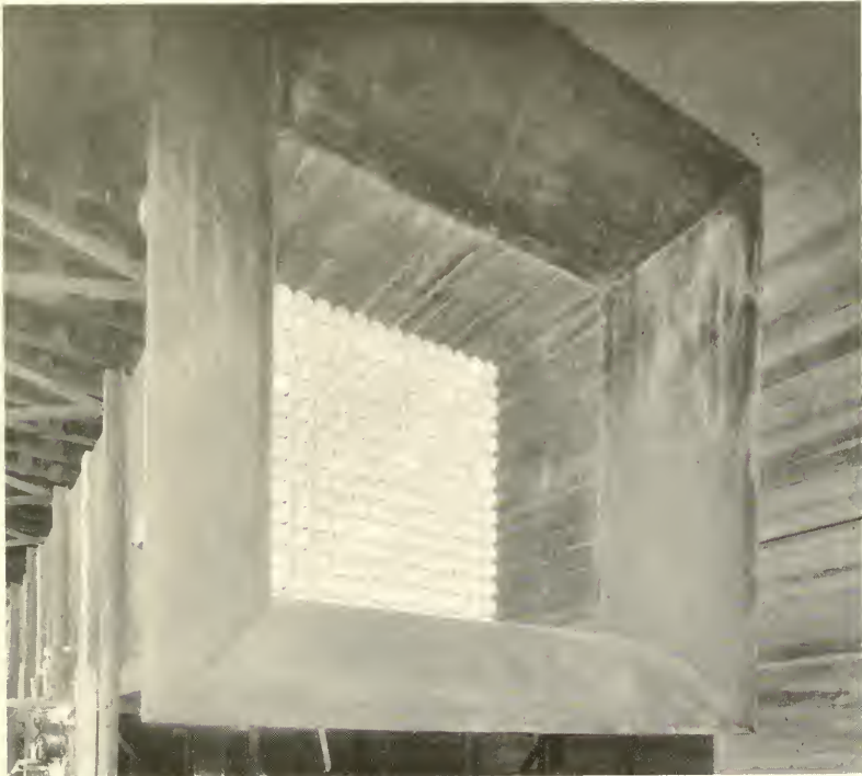
Fig. 2. ENTRANCE NOZZLE, SHOWING END OF HONEYCOMB
