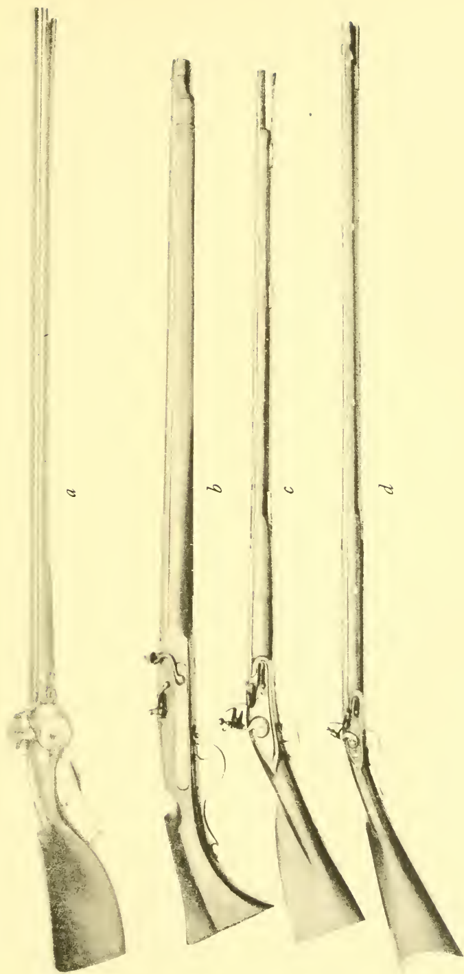
Plate 9. —EARLY TYPES OF SHOULDER WEAPONS USED IN AMERICA: a , Wheel-lock musket, caliber 0.60, Colonial period; b , match-lock musket, caliber 0.80, Colonial; c , French musket, about 1700, used in French and Indian and Revolutionary Wars; d , flintlock, caliber 0.50, formerly rifled, now smooth-bore, 1780-1800.
