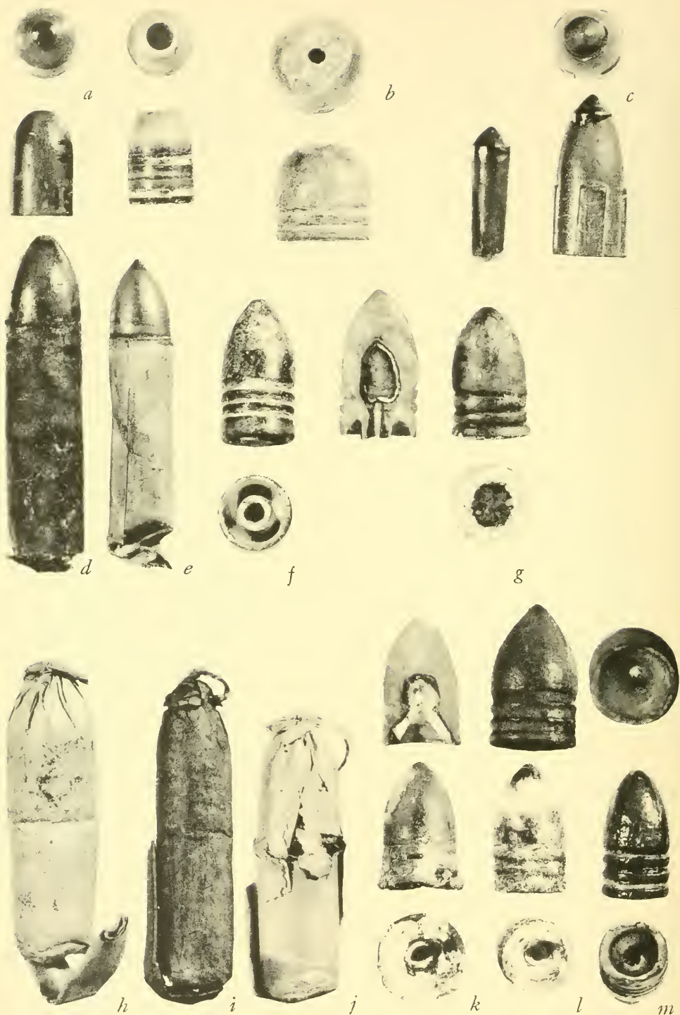
Plate 29.—EXPLOSIVE-BULLET CARTRIDGES FOR RIFLES: a , Experimental bullets with copper nose insert; b , explosive bullet for foreign musket; c , Jacobs explosive bullet; d , Gardiner explosive, caliber 0.58; e , Gardiner, caliber 0.50; f , Gardiner; g , variant Gardiner; h , explosive shell (CSA?), caliber 0.69; i , CSA explosive, caliber 0.577; j , same, damaged by deteriorating bullet; k , bullet from j ; l , bullets from h and i ; m , explosive bullet, CSA, caliber 0.54, and base of l .
