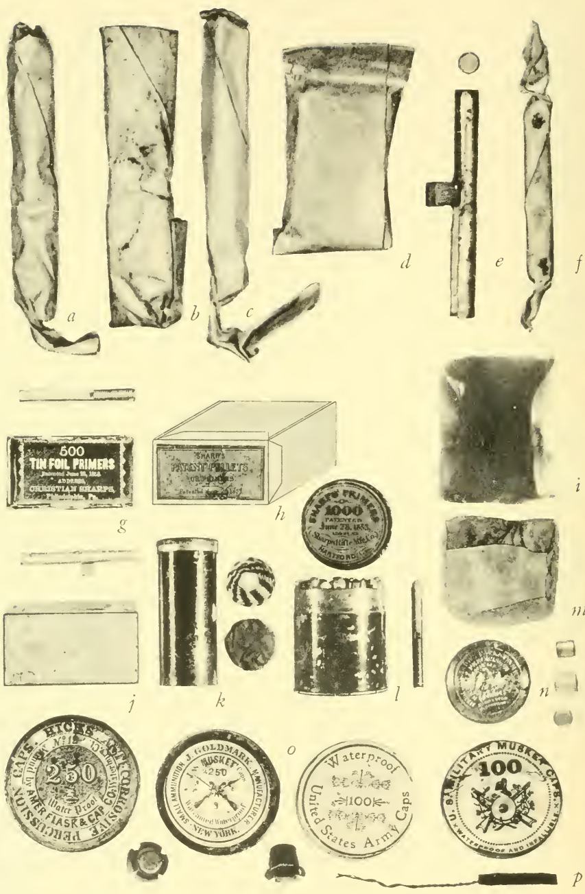
Plate 44.—IGNITION (full size except g, h, j, k, l, n, o , \frac{1}{2} size): a , Packet of 10 caps for Maynard carbine; b , packet of 12 caps for caliber 0.58 rifle; c , packet of 12 caps for caliber 0.69 rifled musket; d , packet of tape primers, M1855; e , tube, pellets for Sharps carbine; f , packet of 8 caps for revolver; g , can of Sharps primers; h , same, foil-lined; i , musket flint; j , can of Sharps primers, C. W. carbine; k , can of Maynard primers for M1855 arms; l , can of Sharps primers; m , pistol flint; n , can of 100 revolver caps; o , cans of musket caps; p , tube primer for Austrian Consol musket.
