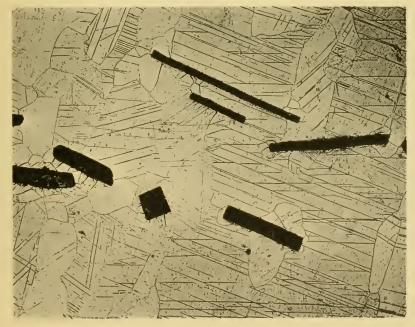
UPPER, AN AREA OF KAMACITE SHOWING FINE GRAINS OF VARYING SIZE AND SHAPE WITH NEUMANN LINES DIVERSELY ORIENTED. SOME AREAS SHOW SUCH GRAINS; IN OTHERS THE KAMACITE IS HOMOGENEOUS. LIGHT PICRAL, X 150.
