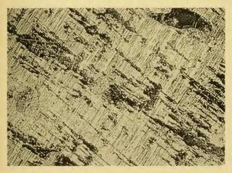
UPPER, SLICE, LIGHT MICRO-ETCH, X 4/5. ONE SET OF NEUMANN LINES IS APPARENT, RUNNING CROSSWISE OF THE SURFACE. IRREGULAR DARK BANDS, RUNNING LENGTHWISE.
