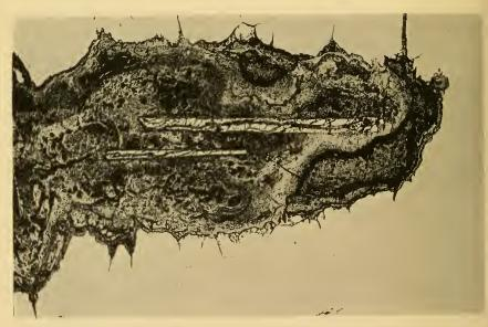
UPPER, SCHREIBERSITE LAMELLA. AS THE FE-FE3P SOLUTION COOLED, THE EXCESS OF IRON (KAMACITE) WAS REJECTED CHIEFLY IN THE FORM OF A CENTRAL LAMELLA INSTEAD OF THE MORE COMMON FORM OF DROPLETS. THIS APPARENTLY IS A PRIMARY STRUCTURE AND NOT THE RESULT OF REHEATING. X 666.
