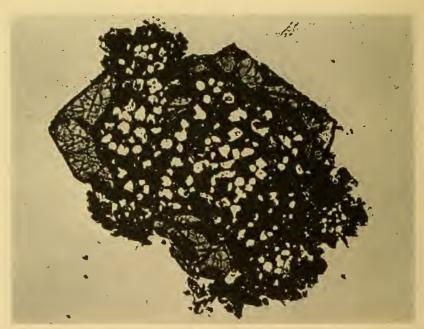
UPPER, AN AREA SHOWING ELONGATED GRAINS; LIGHT PICRAL, X 100. DIVERSE ORIENTATION OF CRYSTALLOGRAPHIC PLANES IN THE ELONGATED GRAINS GIVE THEM A DIFFERENT SHEEN FROM THAT OF ADJACENT GRAINS.
