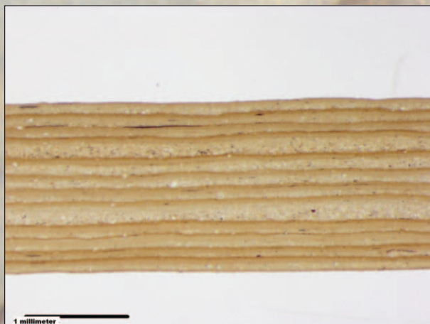
Figure 3. A cross-section of a 1.8-mm-thick piece of oil shale from the Coal Creek Member of the Kishenehn Formation reveals twelve varves with thicknesses from 75 to 250 microns. Scale bar = 1 mm.
