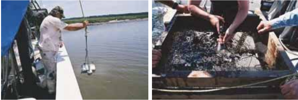
Figure 7. 2013 studies of C 41 site, Jekyll Creek. Left, sediment grab deployed; right, washing a sample grab through wire mesh screens (note algae seen in Fig. 5).
