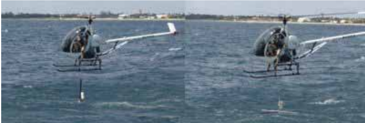
Figure 1. Sensor deployment via helicopter.
