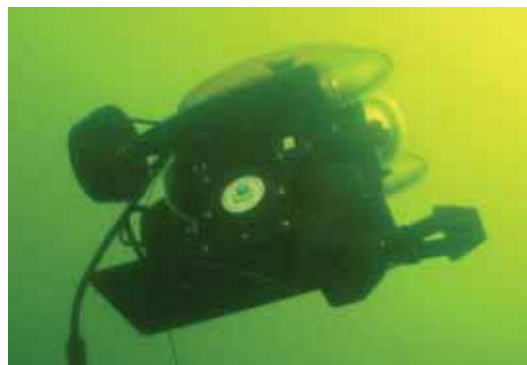
Figure 14. EPA Region 10’s ROV being used to survey a manufactured gas plant site. Photo by S. Sheldrake.
