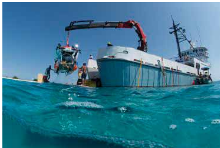
Figure 3. Deploying the Curasub at Klein Curaçao from the R/V Chapman . Photo by Barry Brown.
