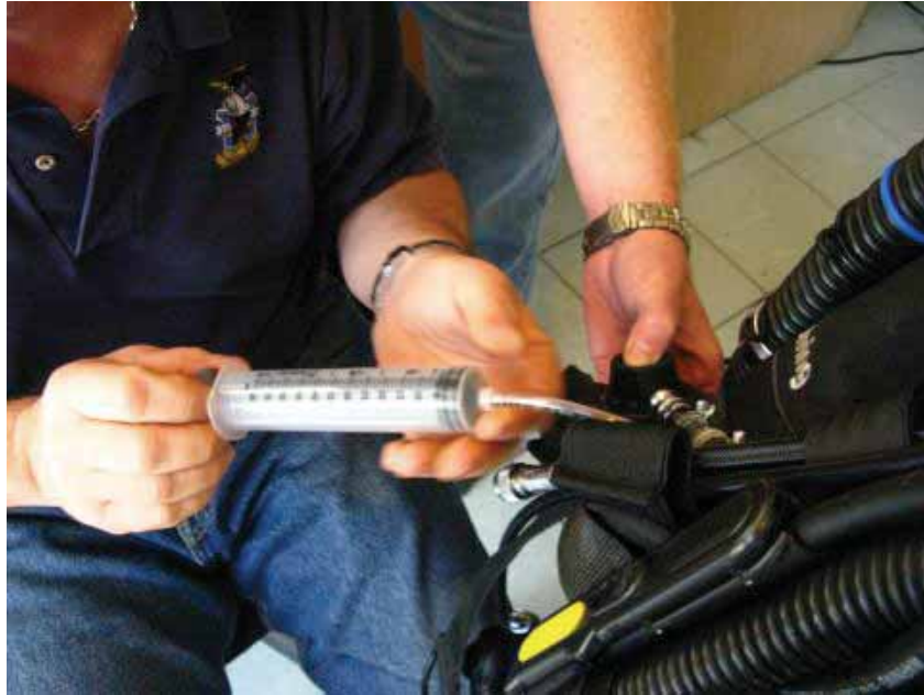
Figure 1. Gas samples pulled from a counter lung for content analysis.
