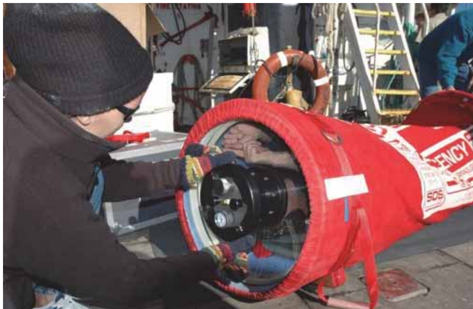
Figure 5. SOS Hyperlite TM Treatment System (Photo credit: Jitka Hyniova - NOAA Collection)
