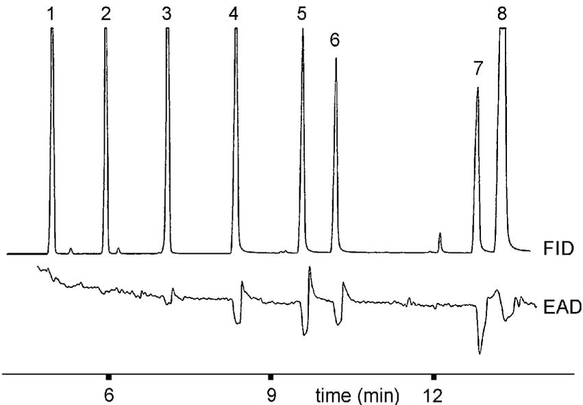
FIG. 1. Gas chromatographic analysis of a mixture of synthetic compounds with flame ionization detector (FID) and electroantennographic detection (EAD) recorded simultaneously using an antenna of a *Euglossa cybelia* male. For names of compounds see Table 1.
