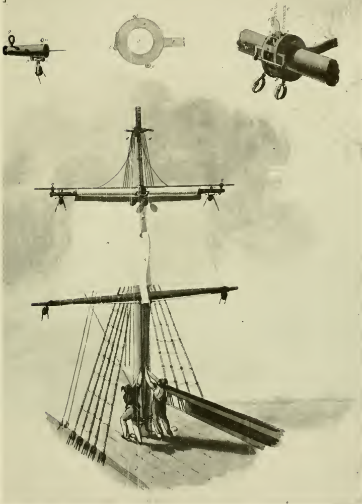
Figure 9.—APPARATUS FOR MAKING AND TAKING IN SAIL invented by John Wade. Patent 101, December 6, 1836.
