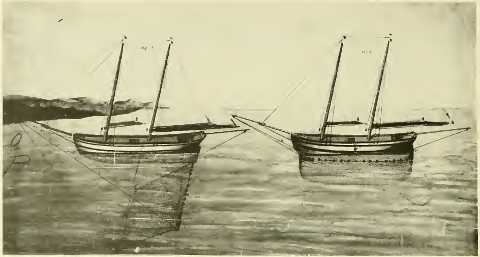
Figure 57.—FISHING NET FOR DEEP WATER designed by B. W. Hale. Patent 763, June 4, 1838.
