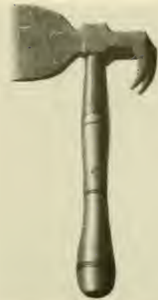
Figure 27.—HAMMER HATCHET patented by Joel Howe on July 8, 1834 (restored patent 8291X).
