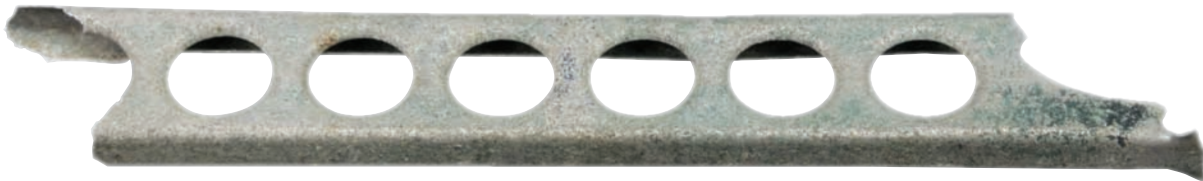
Hindenburg salvaged girder relic, 1937. Duralumin rings and girders formed a framework to hold the gas cells. The holes in the girders reduced the ship's weight. Hindenburg used hydrogen for lift because the U.S. government banned exportation of its helium reserves. Courtesy Navy Lakehurst Historical Society
