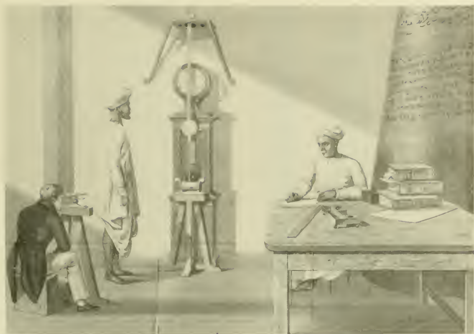
Figure 13. THIS DRAWING ACCOMPANIED John Goldingham's report on the work done in India with Kater's invariable pendulum. The value of gravity obtained, directly or indirectly, in terms of the simple pendulum, is called "absolute." Once absolute values of gravity were established at a number of stations, it became possible to use the much simpler "relative" method for the measurement of gravity at new stations. Because it has only one knife edge, and does not involve the adjustments of the convertible pendulum, this one is called "invariable." In use, it is first swung at a station where the absolute value of gravity has been established, and this period is then compared with its period at one or more new stations. Kater developed an invariable pendulum in 1816, which was used in England and in Madras, India, in 1821.
