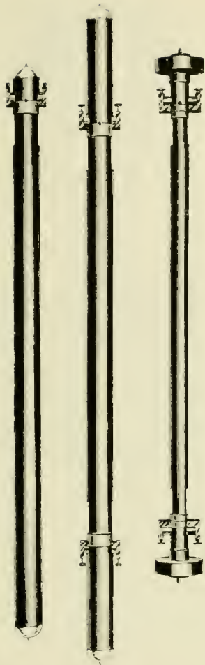
Figure 19.—THREE PENDULUMS USED IN EARLY WORK at the U.S. Coast and Geodetic Survey. Shown on the left is the Peirce invariable; center, the Peirce reversible; and, right, the Repsold reversible. Peirce designed the cylindrical pendulum in 1881-1882 to study the effect of air resistance according to the theory of G. G. Stokes on the motion of a pendulum in a viscous field. Three examples of the Peirce pendulums are in the U.S. National Museum.
