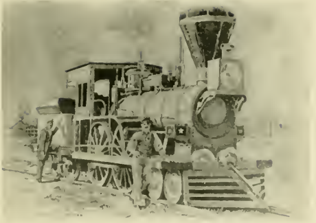
Figure 14.—THE "FURY," BUILT FOR THE Boston and Worcester Railroad in 1849 by Wilmarth. It was known as a "Shanghai" because of its great height. (Smithsonian Chaney photo 6443.)
