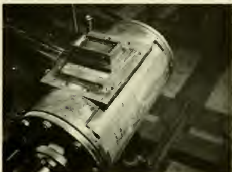
Figures 25 and 26.—CYLINDER with valve box removed, showing valve face.
