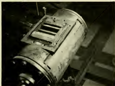
Figures 25 and 26.—CYLINDER with valve box removed, showing valve face.
