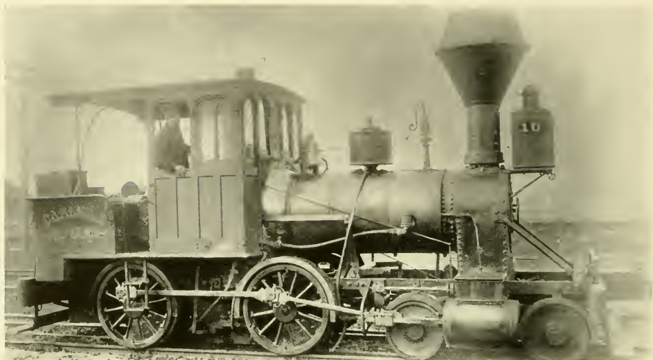
Figure 6.—THE "UTILITY" AS REBUILT TO AN 8-WHEEL ENGINE, about 1863 or 1864. It was purchased by the Carlisle Manufacturing Co. in 1882 and was last used in 1896. (Smithsonian photo 36716F.)
