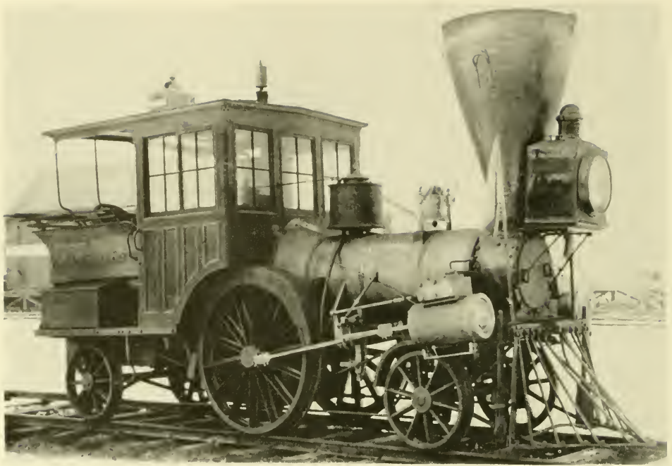
Figure 3.—“PIONEER,” ABOUT 1901, showing the sandbox and large headlamp. Note the lamp on the cab roof, now used as the headlight. (Smithsonian photo 49272.)
