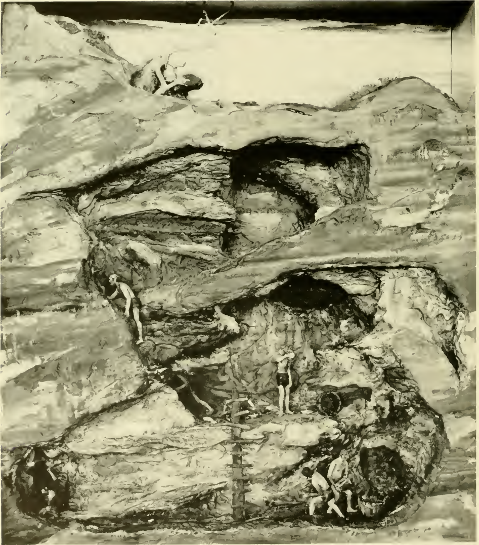
Figure 1.—MINING BY EARLY EUROPEAN CIVILIZATIONS, using fire setting and hand chiseling to break out ore and rock. MIT model— \frac{3}{4} " scale. (Smithsonian photo 49260-H.)
