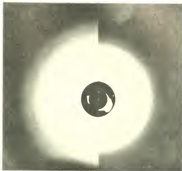
Fig. 140.—X-RAY-BACK-REFLECTION patterns of two gold coins, serving to distinguish between a genuine struck coin (left) and a counterfeit cast piece (right).
