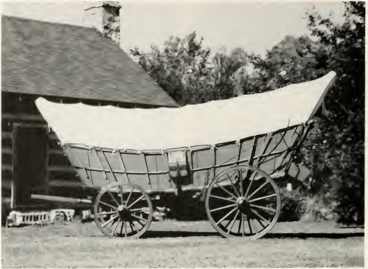
Figure 6.— RESTORED FREIGHT-CARRYING CONESTOGA WAGON, about 1830, in the collection of the author. The tongue is not full length. (Photo by the author.)
