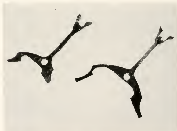
Figure 15. VERGE AND LEVER for an Auburndale timer. The one on the left beats eighths of a second; that on the right beats quarters. (In author's collection.)
