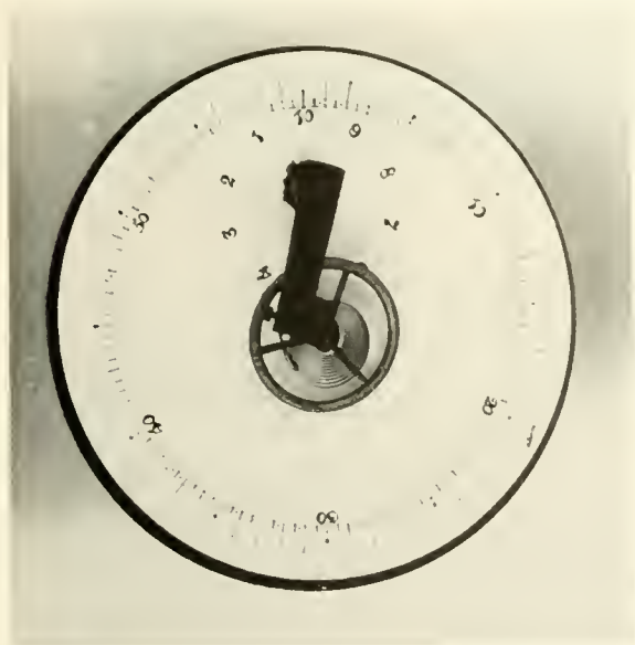
Figure 17. A TIMER DIAL that is probably either experimental or very early. Note that the fractions of a second (quarters) are shown on the outside dial instead of on a separate dial. This dial was converted at the factory for use as the base of a hairspring vibrating stand. A dial different from this but having the same arrangement of circles is known. (In author's collection.)
