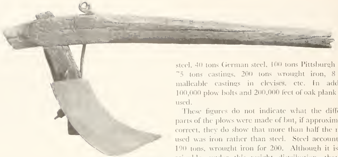
Figure 7. JOHN DEERE'S 1838 PLOW, RIGHT SIDE, showing large iron staple used to fasten end of right handle to the standard. Note remains of wooden pin near rear end of plow beam. (Cat. no. F1111; Smithsonian photo 42639-1.)
