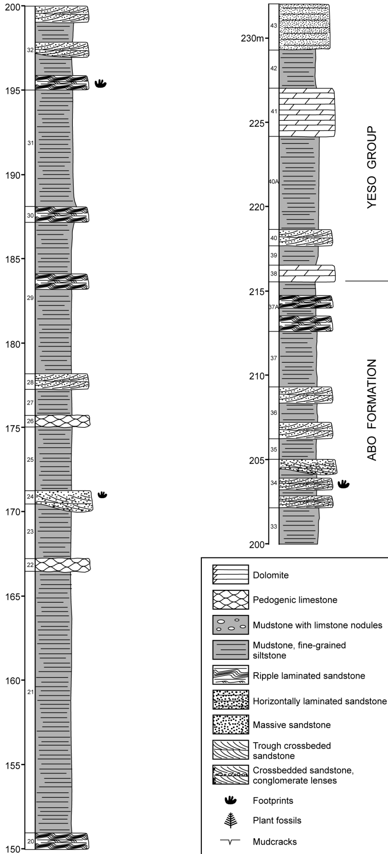
FIGURE 8. Continued. Measured stratigraphic section of the uppermost Bursum Formation, entire Abo Formation and lower part of the Yeso Group (lower part of Arroyo de Alamillo Formation) at Stop 2.
