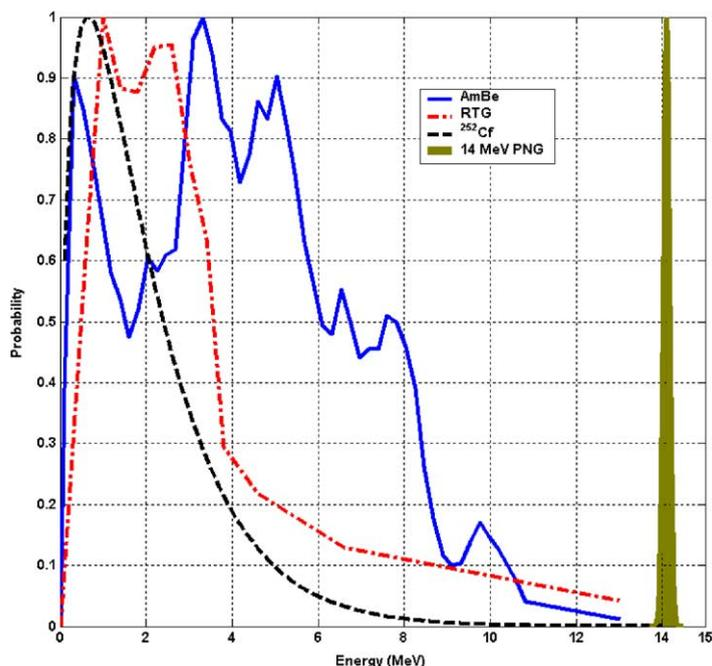
Fig. 1. The source spectra for AmBe [4], RTG [5] and  $^{252}\text{Cf}$  [6] isotopic neutron sources are shown. Note that the spectra for  $(\alpha, n)$  sources can vary significantly in details especially below 2 MeV, depending on the homogeneity of the target and  $\alpha$  emitter mixture and the thickness of the capsule. The emitted neutron energy from D–T reaction is almost mono-energetic with average neutron energy of 14.4 MeV.
