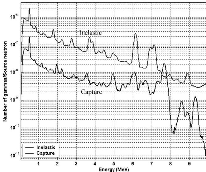
Fig. 4. The CsI gamma-ray detector response for a soil sample with the APXS instrument composition [3] + 3% water. The capability of turning the source on and off for a given pulse width allows recording inelastic and capture spectra separately. The resolution of the CsI detector was 8.5%.
