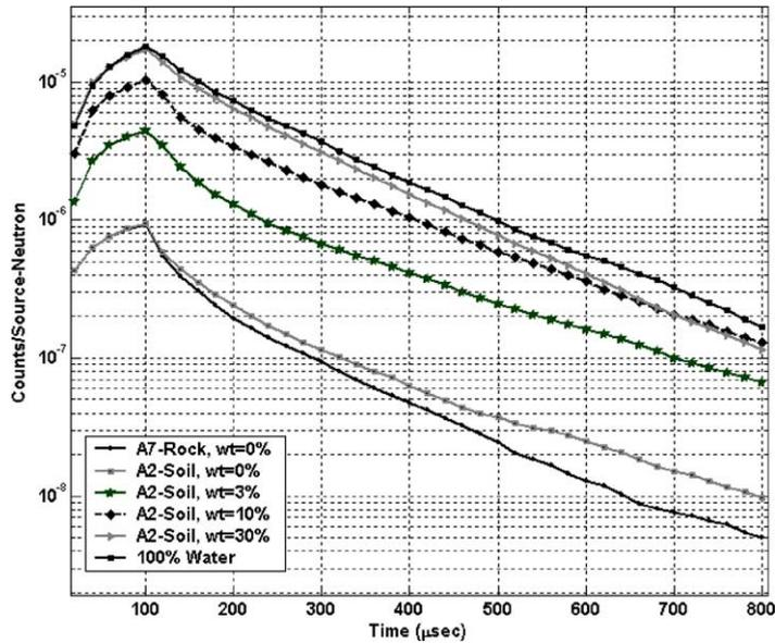
Fig. 3. Thermal neutron detector time detector response for varying water content in soil [3]. The count rate per acquisition time interval is obtained by multiplying by the neutron source output.
