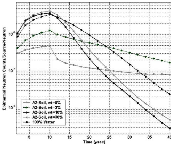
Fig. 2. Epithermal neutron detector time dependent response for varying water content in soil [3]. The count rate per acquisition time interval is obtained by multiplying by the neutron source output.
