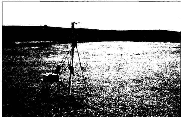
Figure 6. Ash deposit surface at Kilauea. The tripod supports a laser micro-topography mapper (sub-cm accuracy).
