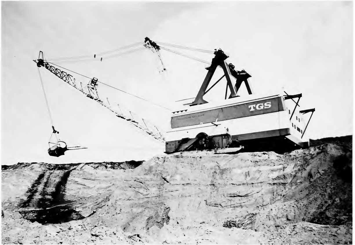
FIGURE 2.—Dragline on working bench after chopdown, lifting 72-cubic-yard ( 55\text{-m}^3 ) bucket containing 100 tons of phosphate ore (dark colored) to be stacked in background at surface for slurring and piping to mill. Spoil windrow in foreground. Courtesy of Texasgulf Inc.
