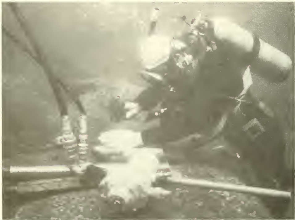
A Smithsonian Tropical Research Institute biologist is shown preparing to drill into a coral reef. The cores obtained from this work will help determine whether the extraordinary die-offs of coral reefs have occurred previously during the last 1000 years.
