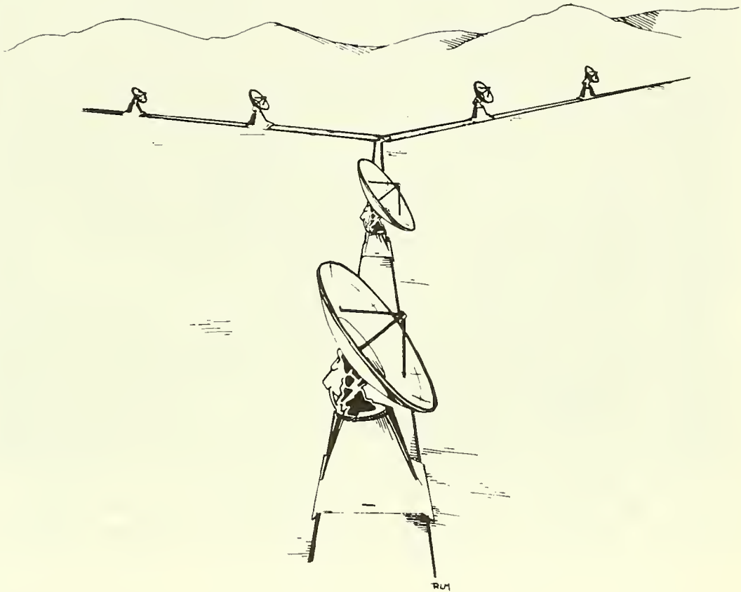
The SUBMILLIMETER TELESCOPE ARRAY, shows artist's conception of the six-element array of radio telescopes proposed for observations in the submillimeter wavelength band of the electromagnetic spectrum. The movable antennas would be mounted on a Y-shaped track.
