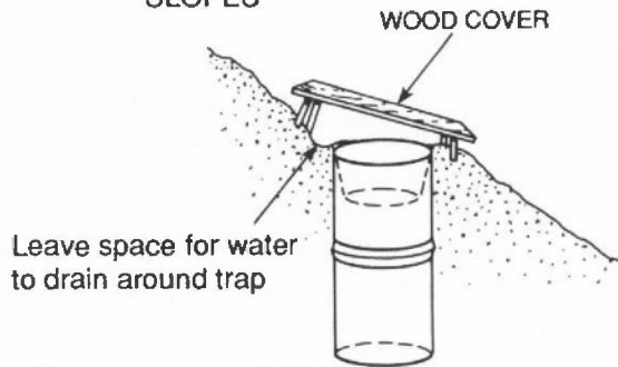
Figure 12. Construction of pitfall traps from two number-10 tin cans (reprinted with permission from Corn and Bury 1990).
