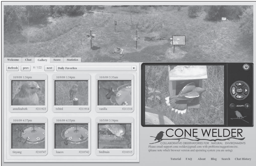
FIG. 2. Interface of the website ( http://cone.berkeley.edu ) for the collaborative telerobotic wildlife camera system, CONE Welder. The top panorama illustrates the camera field of view, which allows users to draw rectangles to control the camera. The camera window on the right side of the frame shows the live view. Each user can capture a picture by clicking on the camera button to the right of the live view. The image is then stored and displayed in the list at the left side of the live view, where users can enter their comments to annotate the image or comment on photos taken. Each user logs on to the system to draw rectangles on the panorama to indicate where they want the camera to observe. Details regarding camera operation can be found in Song (2009).
