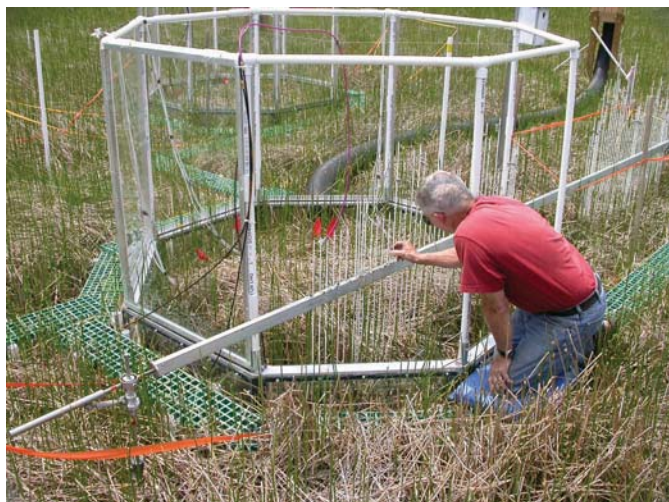
FIGURE 4. Photograph of SET measurements being made in summer 2006. Each pin is gently lowered to the soil surface, while applying minimal pressure so that the pin does not depress the soil surface. (Photograph by M. V. Sigrist.)
