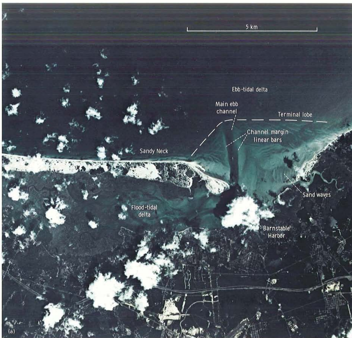
FIGURE 8.—Barnstable Harbor. (a) High-altitude aerial photograph showing components of the ebb-tidal delta. (b) Bathymetric chart of the area (ref. 5). Contour interval is 5 m.
