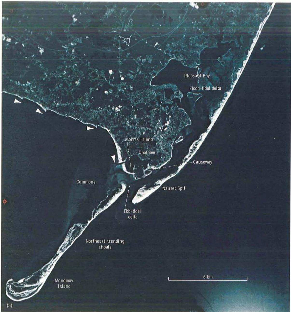
FIGURE 7.—Nauset Beach and Monomoy Island. (a) High-altitude aerial photograph showing areas of change on Nauset Spit and Monomoy Island. Triangles indicate direction of longshore drift. (b) 1967 bathymetric chart (ref. 6) showing changes in Nauset Spit and Monomoy Island. Dashed lines indicate positions on 1975 photographs. Contour interval is 1 fathom (1.8 m).
