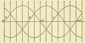
FIG. 14. Three-phase alternating current diagram
