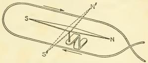
FIG. 2. Zweigger's improved galvanometer
