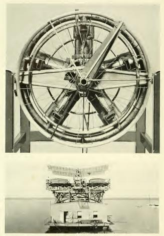
Upper: Manly 52-h.p. radial gasoline engine, built for Langley's full scale airplane. Weight 120 pounds. Lower: Langley's full-scale airplane poised for flight
