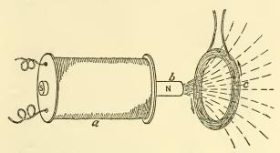
FIG. 11. The electric repulsion principle. Diagram to illustrate Dr. Elihu Thomson's invention of the electric repulsion motor
