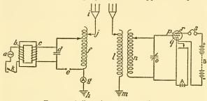
FIG. 30. A discontinuous-wave radio set
