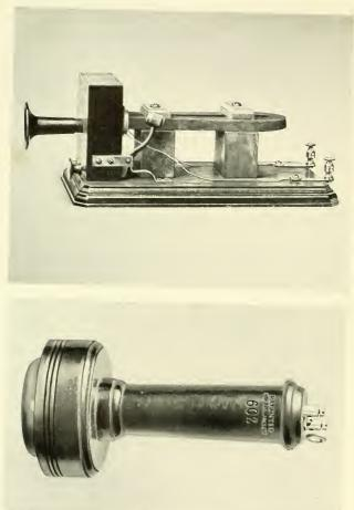
Upper: Bell's box telephone of 1877 with hammer called "Watson's thumper" used to attract the listener. Lower: Hand telephone receiver of 1877
