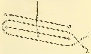
FIG. 3. Faraday's galvanometer
