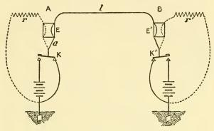
FIG. 23. Duplex telegraph diagram
