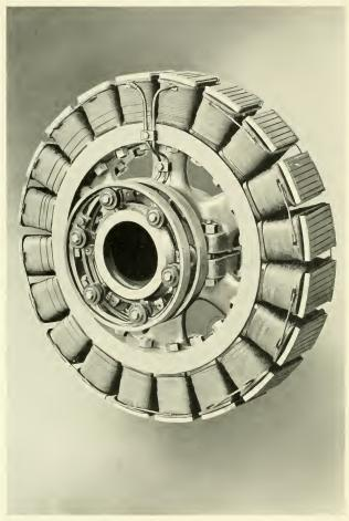
Rotating field of alternator. Approximate diameter 4½ feet. Courtesy of the General Electric Company
