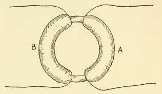
F10. 5. Faraday's iron ring experiment, whereby he first produced electricity by magnetism
