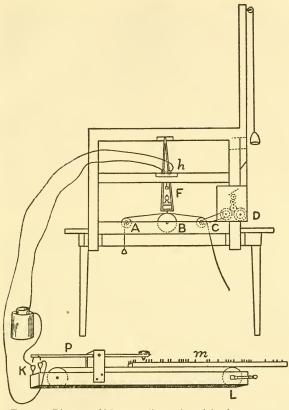
F10. 22. Diagram of Morse sending and receiving instruments. The "port rule" for sending, shown below, produces intermittent currents in the line. These operate a magnet, which draws over a pendulum carrying a point that embosses the paper record fed along by clockwork. A relay may be interposed to strengthen the action
