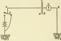
FIG. 25. Cable operation through electric condenser
