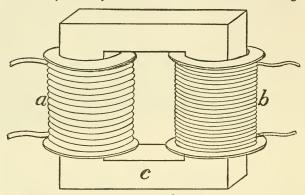
FIG. 13. A step-up transformer, to convert alternating current of moderate voltage to alternating current of higher voltage
