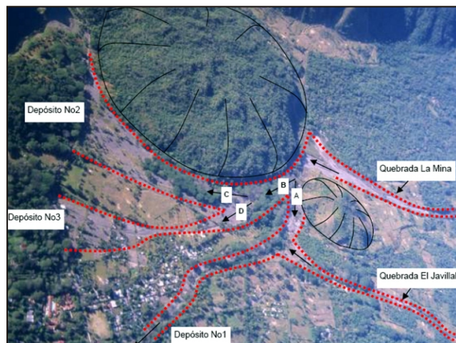
Figure 17. Annotated aerial photo at unknown date showing part of Coatepeque’s Planes de Laguna, W of Santa Ana, taken looking roughly S. The view illustrates lahars in and around El Javillal. The lahars entered the area along two drainages (Quebradas La Mina and El Javillal), both flowing from right to left (arrows). Adjacent to the domes and settlements, the flow patterns become quite complex (as indicated by flow directions A, B, C, and D). Lake Coatepeque appears at the upper left. The steep caldera wall lies along the photo’s margin from the upper center to right corner. The large circular dome is Cerro Pacho; the smaller dome to the right is Cerro Guacamayero. Photo from SNET (2006).
