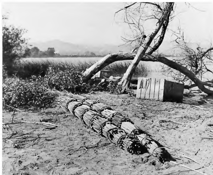
Figure 75. Bundles for Pomo tule balsa boat, including keel bundle and one side bundle, on the shore of Clear Lake, California. Note the method of joining the tules before tying, suggesting that the boat definitely had a forward end. Photograph probably by S.A. Barrett, ca. 1915. Courtesy of Lowie Museum of Anthropology (Cat. No. 15-17287), University of California, Berkeley.
