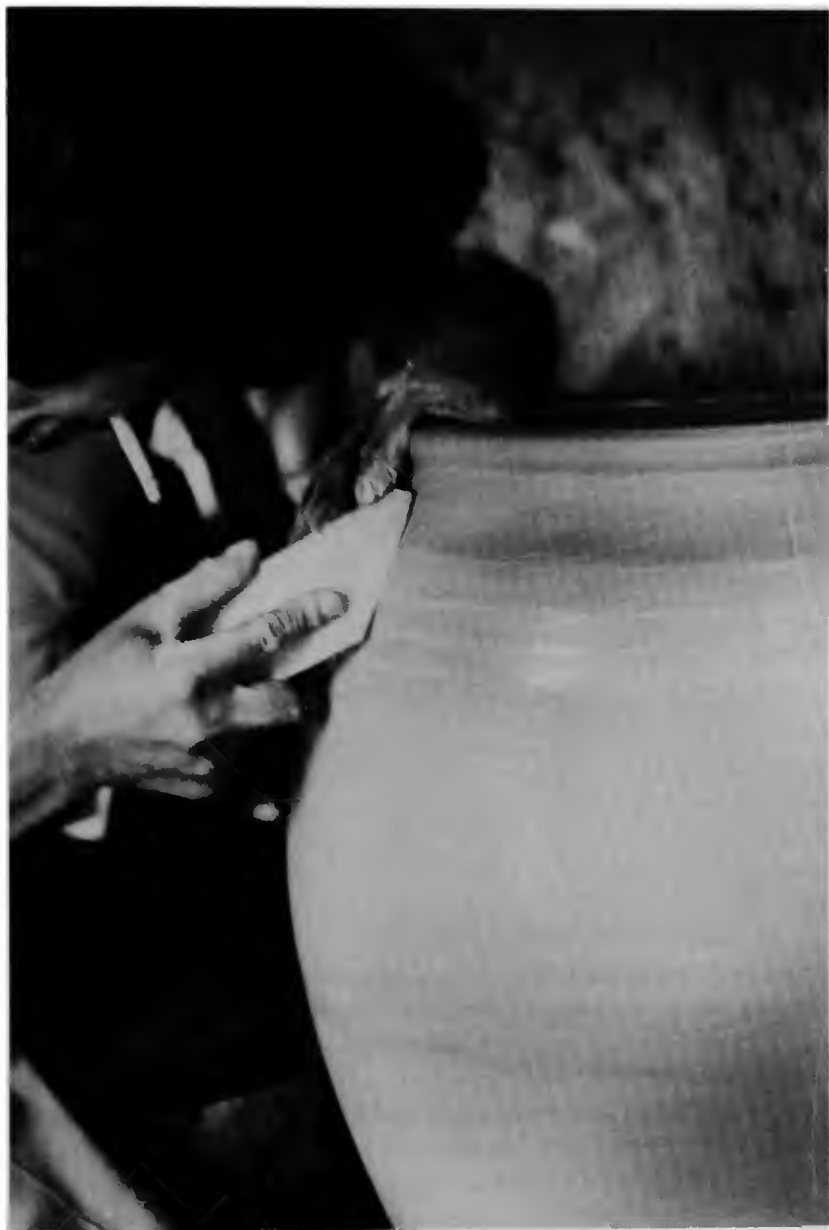
Figure 921. Cylinder wall finished with trapezoid (kūn'gi).
