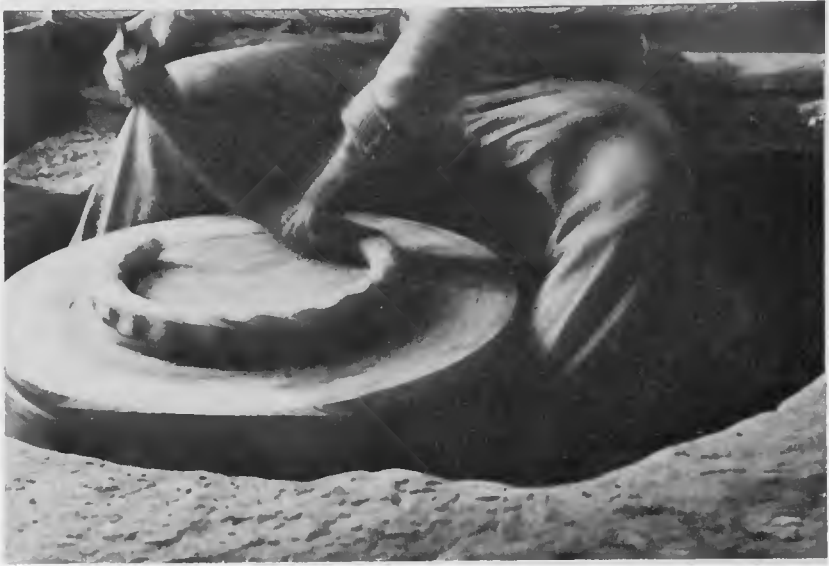
Figure 60b. Coil added around perimeter of disk.
