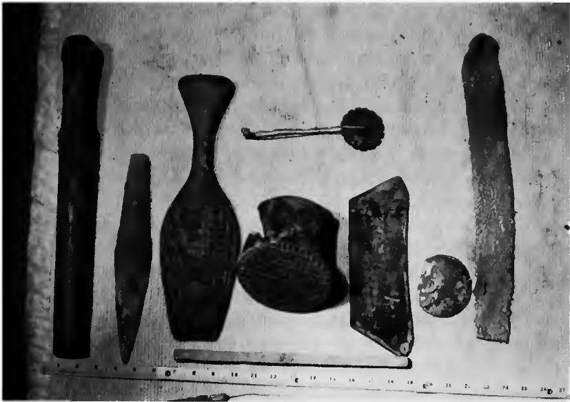
Figure 45. Potters' tools at Sönggwang Factory (left to right): bottom flattener (pangmangi), incising awl (mitkasae), paddle (surae), anvil (t'oge), outside shaper (pakkat kün'gae), inside shaper (an kün'gae), cloth finishing strip (mulgajuk), (top) roller stamp (torürae), and (bottom) stick gauge (padak chönggüm). (Scale in inches.) (Photo by Ralph Rinzler, 1971.)
