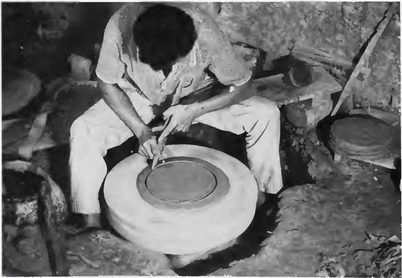
Figure 34c. Bottom disk inscribed with awl (mitkasae). This procedure centers the base while trimming it to its proper diameter.
