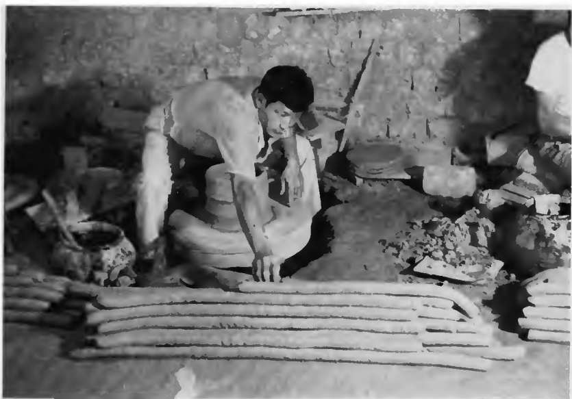
Figure 34e. Initial coils added in slow clockwise direction.
