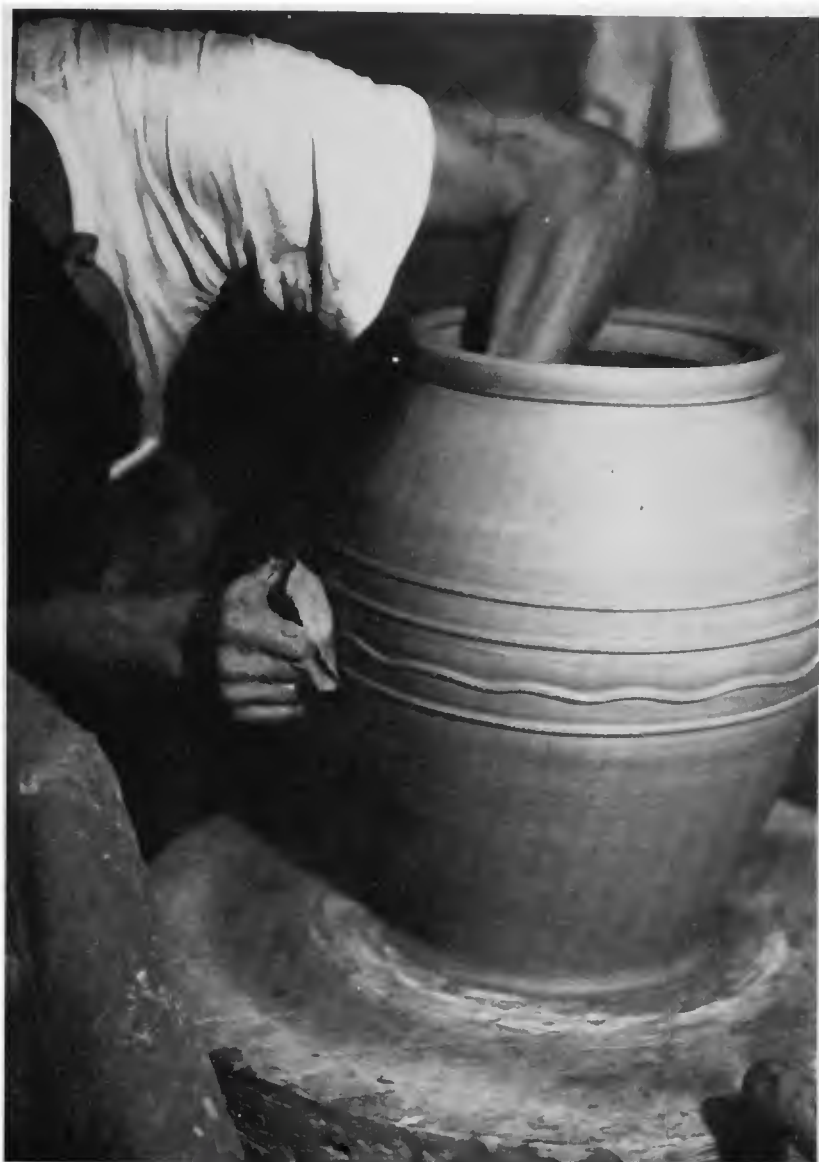
Figure 34i. Wavy dragon line (yong tti) added around midpoint of vessel with leather strip.
