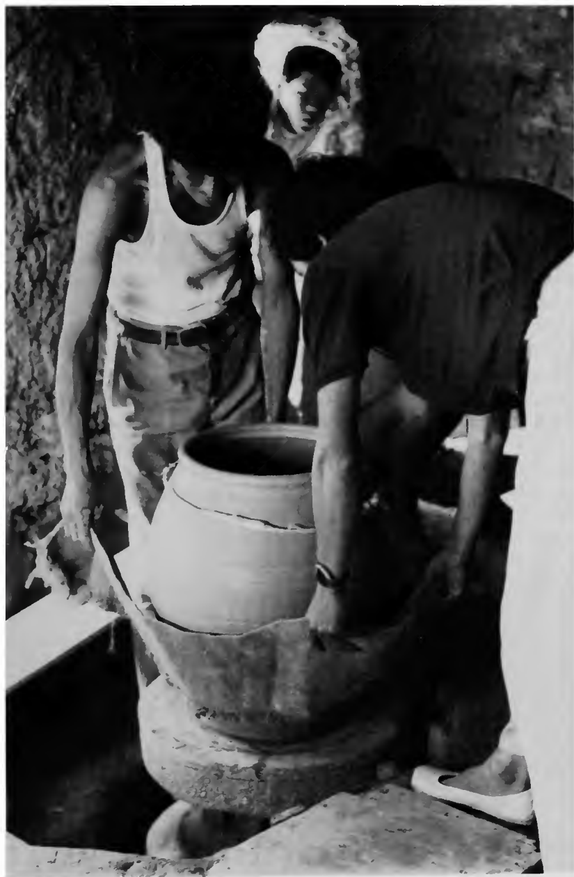
Figure 92p. Pot removed from wheel in burlap sling (ttökpatchi). Plastic-covered ring (teduri) encircles vessel to prevent distortion of wall. Factory owner Yi Hae-man called the Chölla slab method noböng t'aeryöm and the coil method used elsewhere chwoigi t'aeryöm. Potters in Kyönggi Province gave taegi t'aerim and ch'etpaggu t'aerim.
