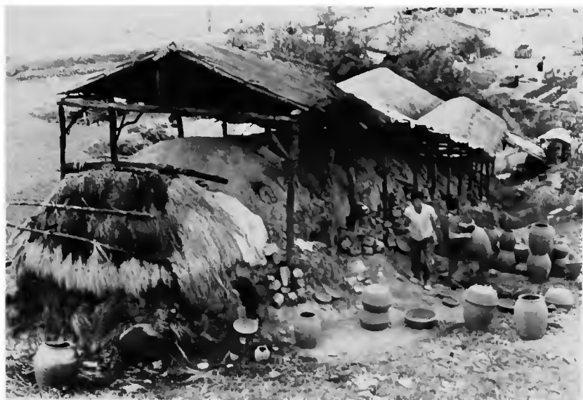
Figure 102. Chamber kiln (called kaeryanggul in the Kyōngsang provinces) at Turyang village factory. The workers had just opened the chamber doors after seven or eight days of firing (note insulating thatch piled over structure's upper end) and were carrying 4500–5000 jars down a steep walkway adjacent to the kiln. Broken vessels and sherds were used to line drying beds at a local salt-processing plant. (Photo by Ralph Rinzler, 1972.)
