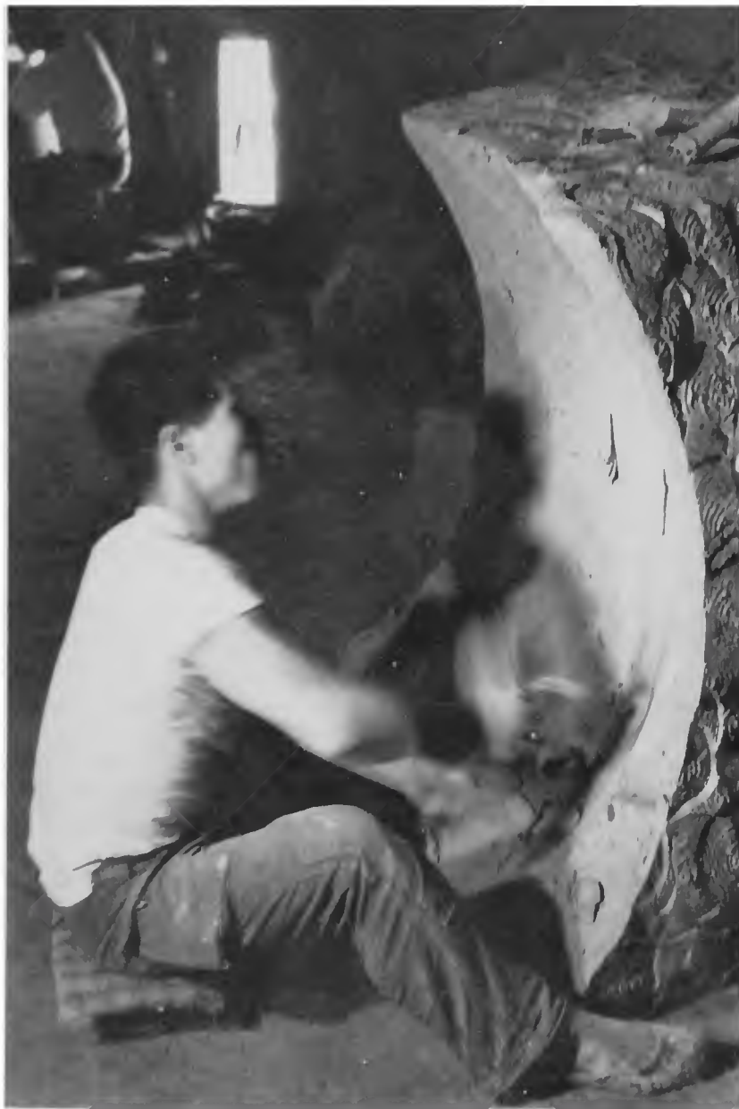
Figure 44. Potter's assistant using metal blade to shave clay ribbons from large mound. (Photo by Ralph Rinzler, 1971.)
