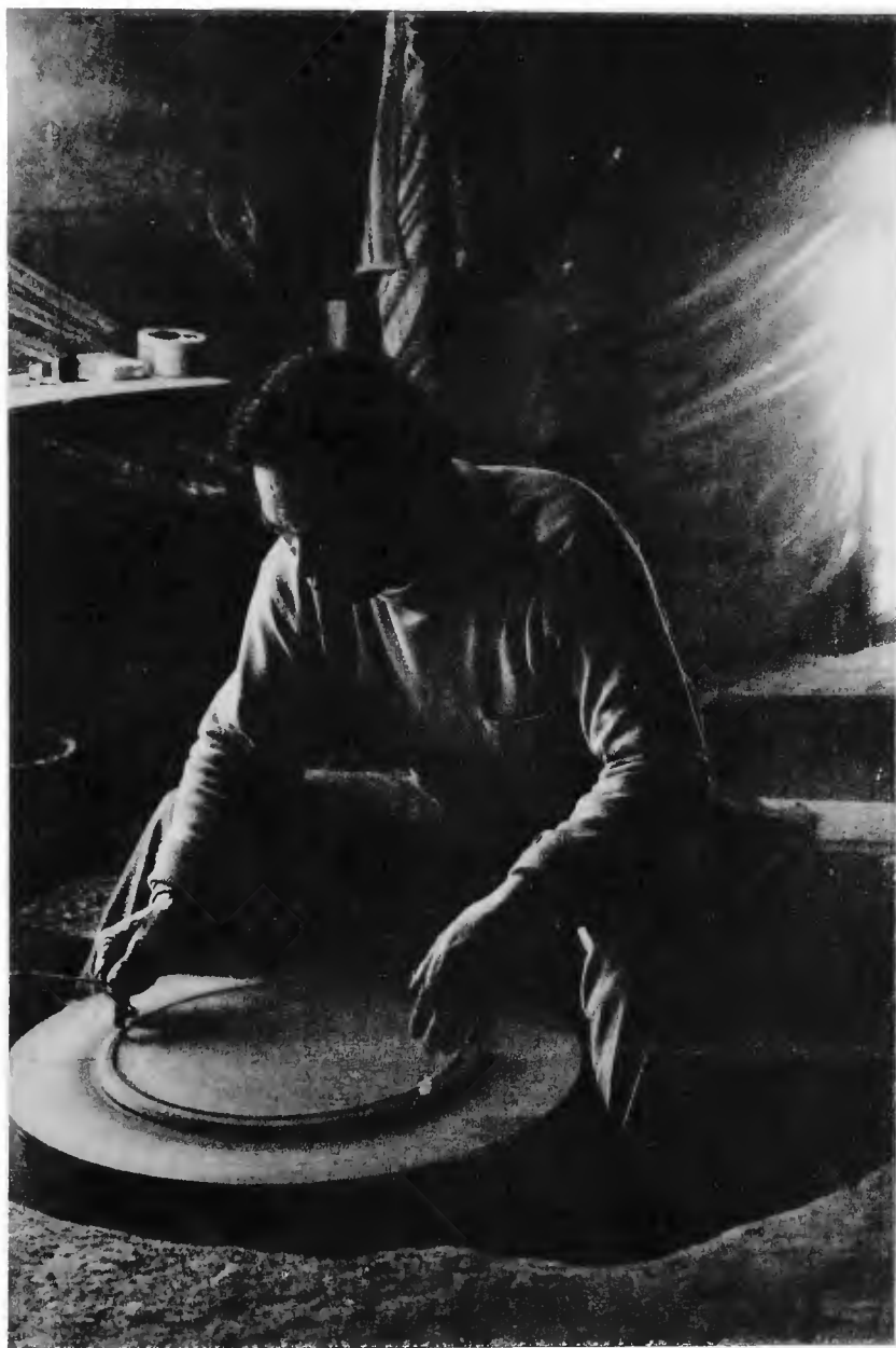
Figures 60a–d. Manufacturing storage jar lid. (Photos by Ralph Rinzler, 1982.)
