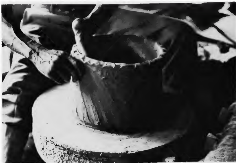
Figure 92d. Cylinder wall thinned with knuckle and side of right forefinger.
