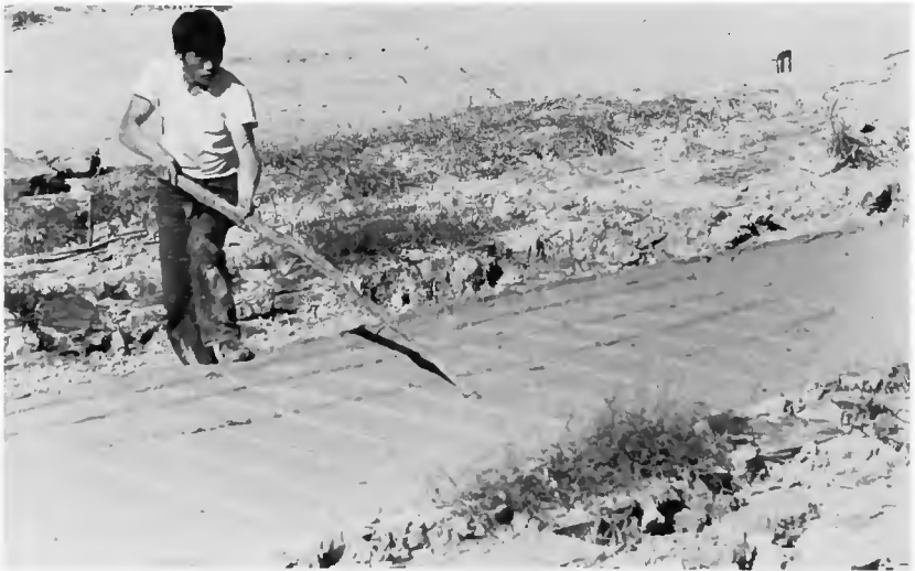
Figure 72. Worker inscribing clay beds to hasten drying and to facilitate later handling of material. (Photo by Ralph Rinzler, 1972.)
