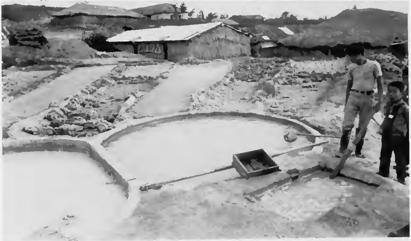
Figure 71. Clay washing tanks and drying beds at Kaya village. The clay is passed through the strainer in foreground enroute from the square mixing box into the circular settling tank. (Photo by Ralph Rinzler, 1972.)
