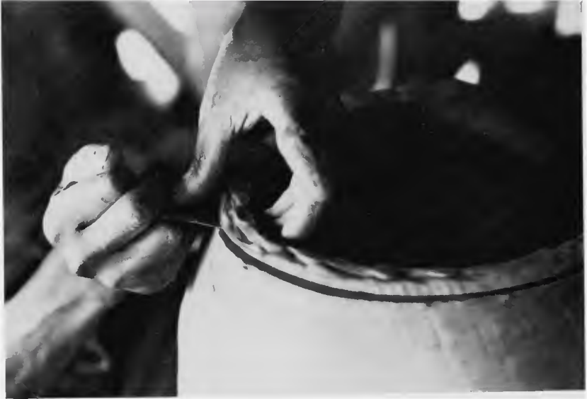
Figure 92j. Rim evened with small metal awl (mokkasae).
