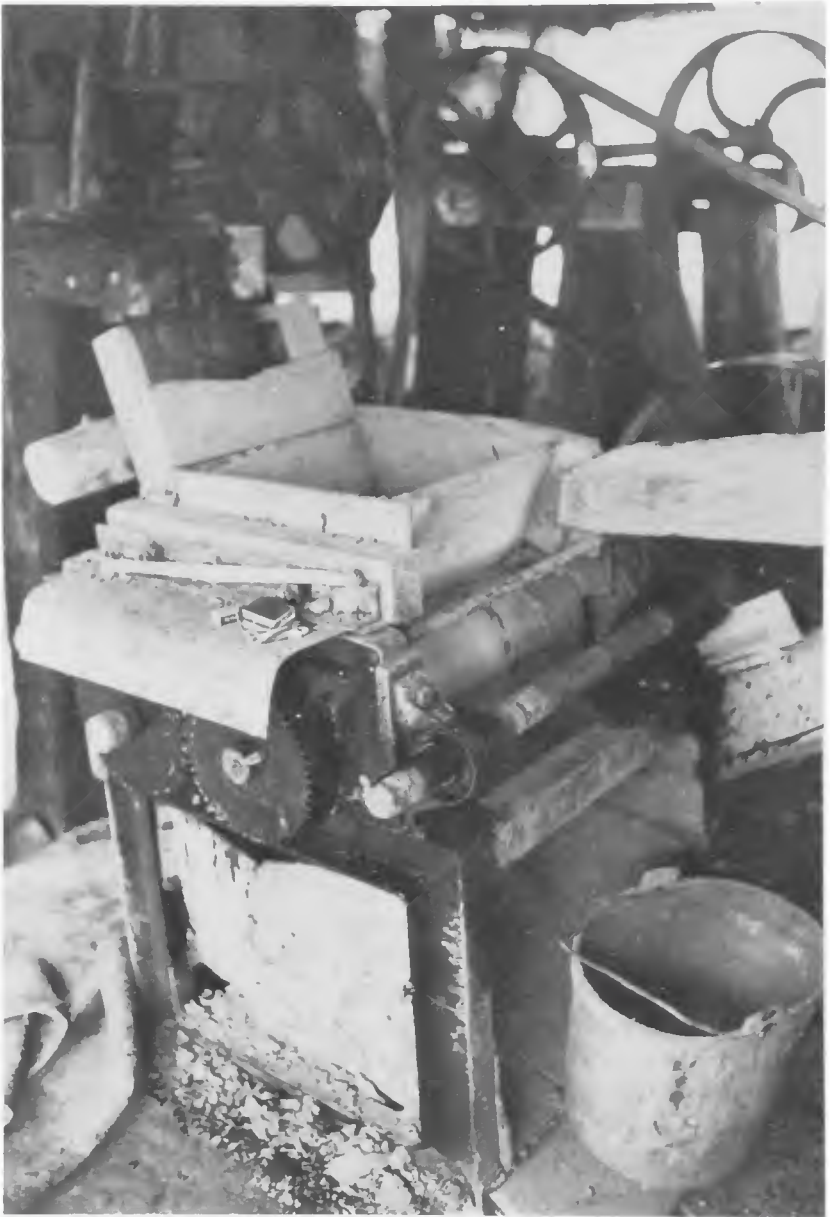
Figure 48. Rolling mill (rora) at Songgwang Factory. This machine and a clay extruder are connected by belts and pulleys to a diesel engine. (Photo by Robert Sayers, 1981.)
