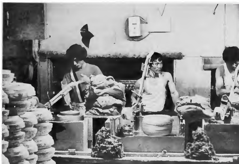
Figure 37. Workers at Künjin Factory manufacturing ware with jiggling knives and templates. (Photo by Ralph Rinzler, 1981.)
