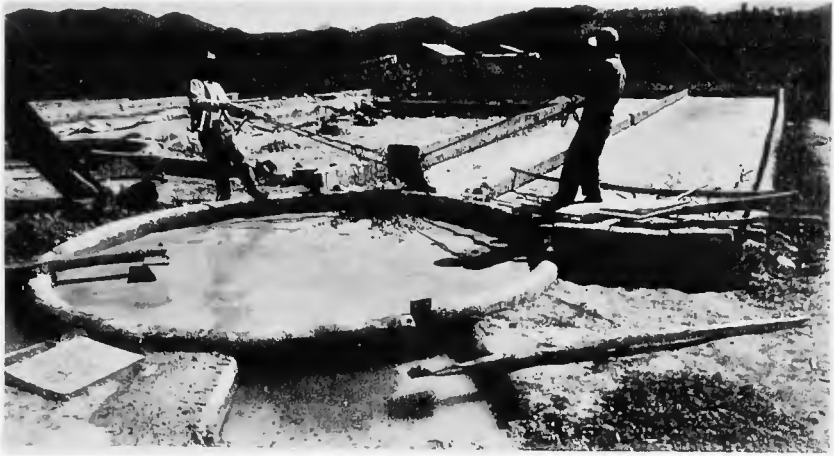
Figure 57. Men using swinging conveyance ( pagaji ) to transport clay slurry from settling tank to drying beds. Clay is initially mixed in the rectangular box (foreground), then is strained into the round settling tank. Sim Sang-un in 1981 still processed his clays in this manner before cycling them through a rolling mill and an extruder. (Photo by Ralph Rinzler, 1971.)
