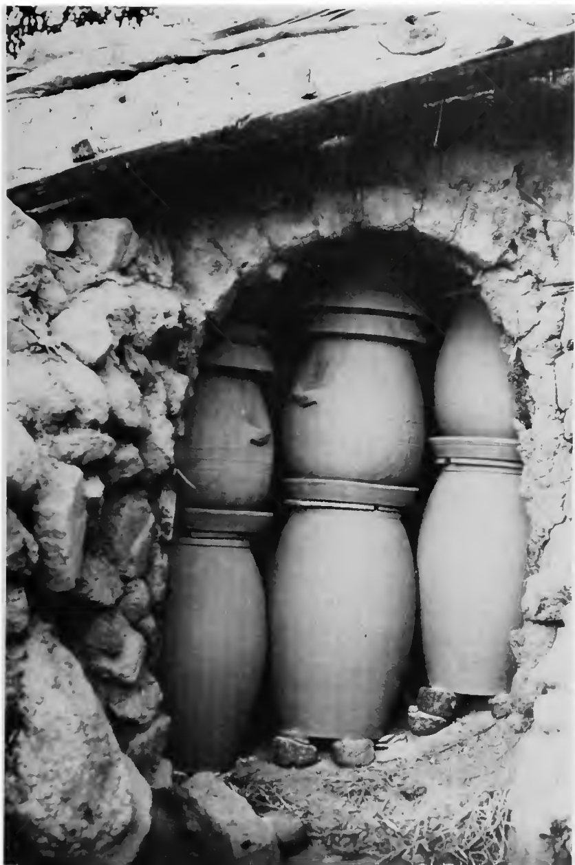
Figure 75. After nesting, the ware is stacked inside the kiln on clay or stone pads with ceramic disks separating the layers. (Photo by Ralph Rinzler, 1972.)
