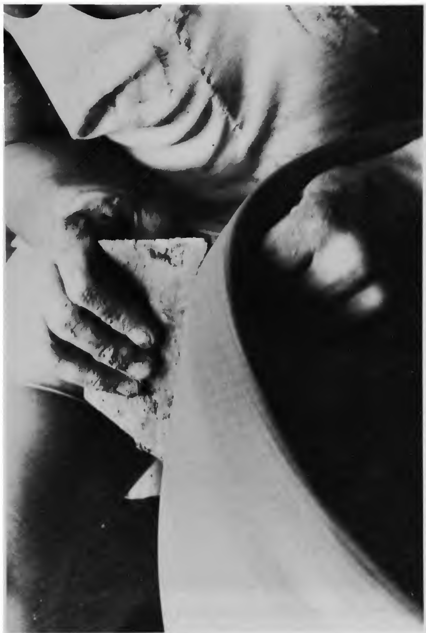
Figure 34g. Sides of jar thinned with metal trapezoid (kūn'gae) and clamshell (an kūn'gae) in fast counter-clockwise direction.
