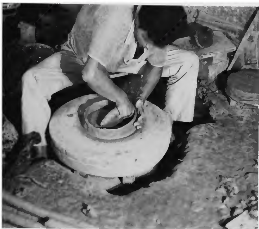
Figure 34d. Clay ring mounted on centered base.
