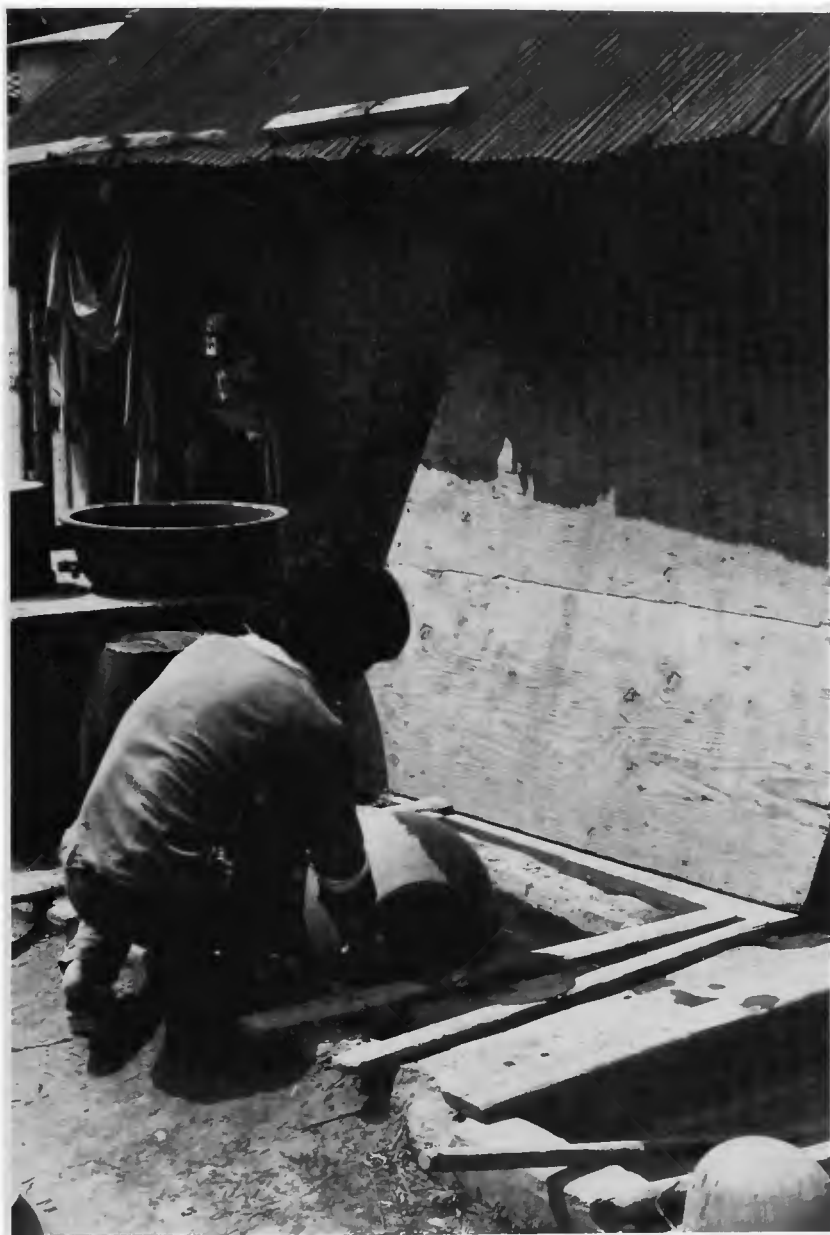
Figure 115. Rolling jar in glaze solution. (Photo by Ralph Rinzler, 1981.)
