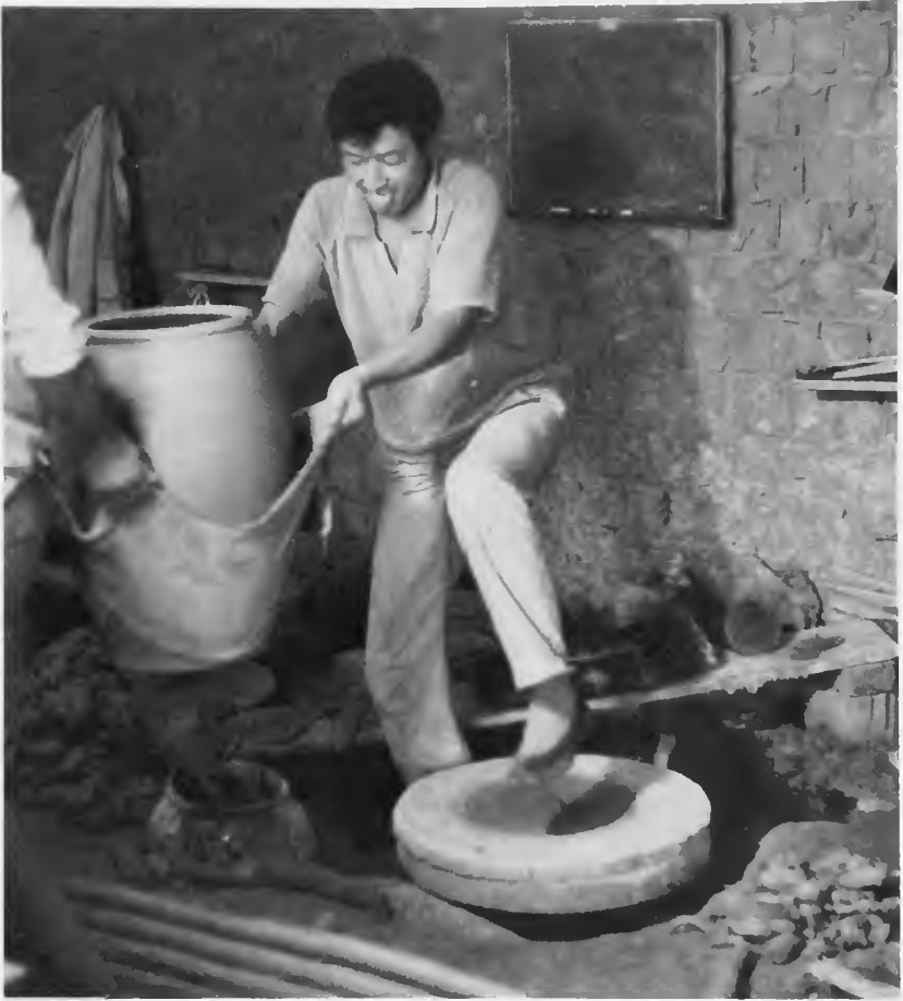
Figure 34m. Finished jar lifted from wheelhead in cloth sling.
