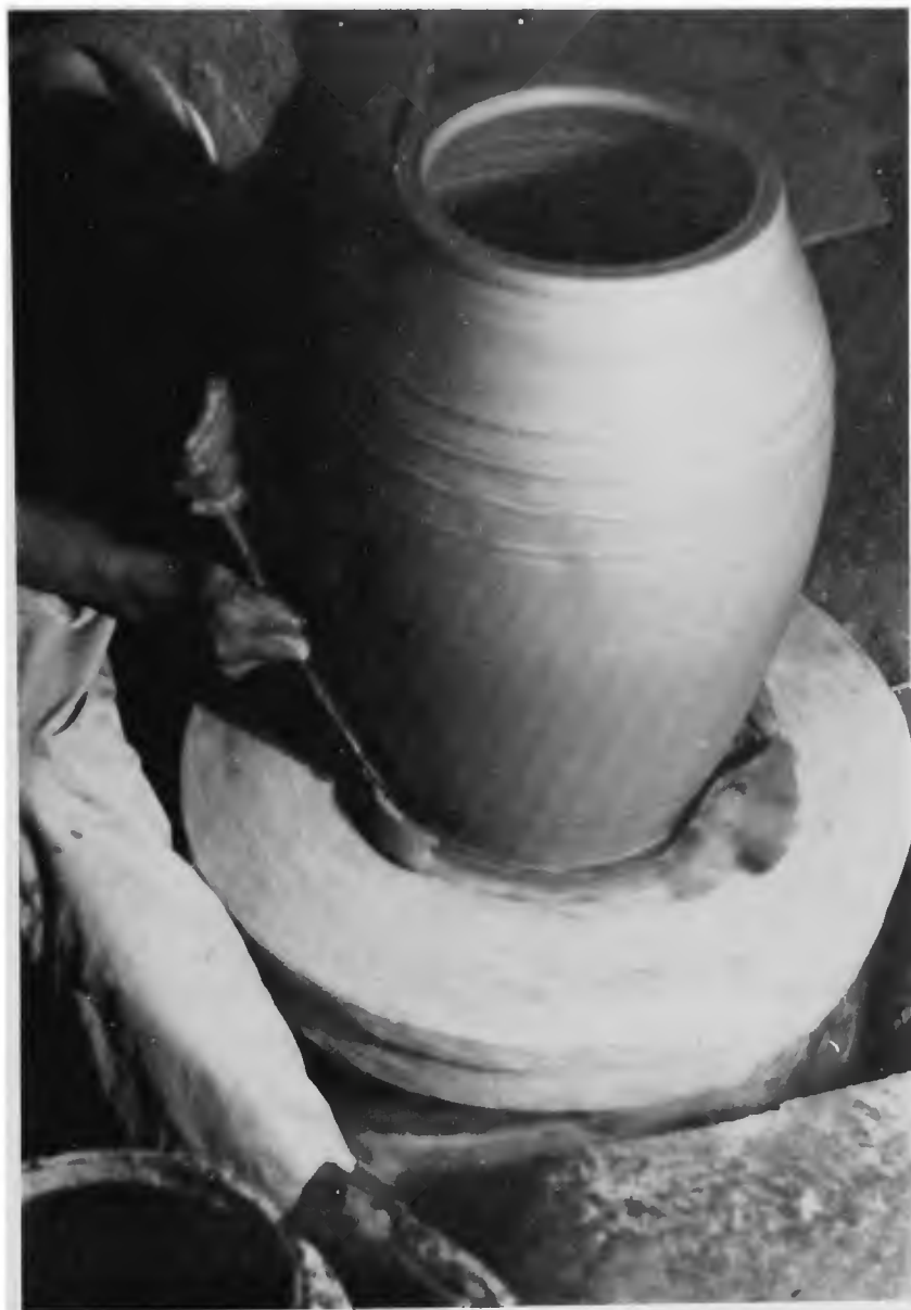
Figure 34l. Vessel bottom trimmed with awl.
