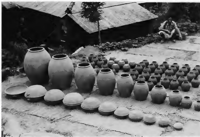
Figure 101. Turyang village factory owner Kang Kil-bu with unfired storage jars (in descending order of size): tae tchari, ch'ilbu, tchak tanji, set tchebi, chul sa tan, chul o tan, al sa tan, al o tan, yuk tan, and sip tan. These jars will shrink in size by approximately 30 percent during firing. (Photo by Ralph Rinzler, 1981.)
