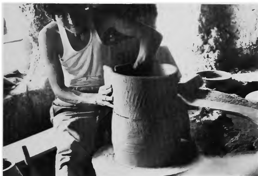
Figure 92g. Adding second slab.
