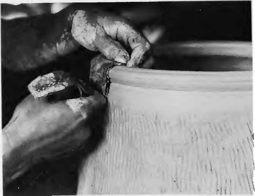
Figure 92k. Vessel lip formed with leather strip (mulgajuk).
