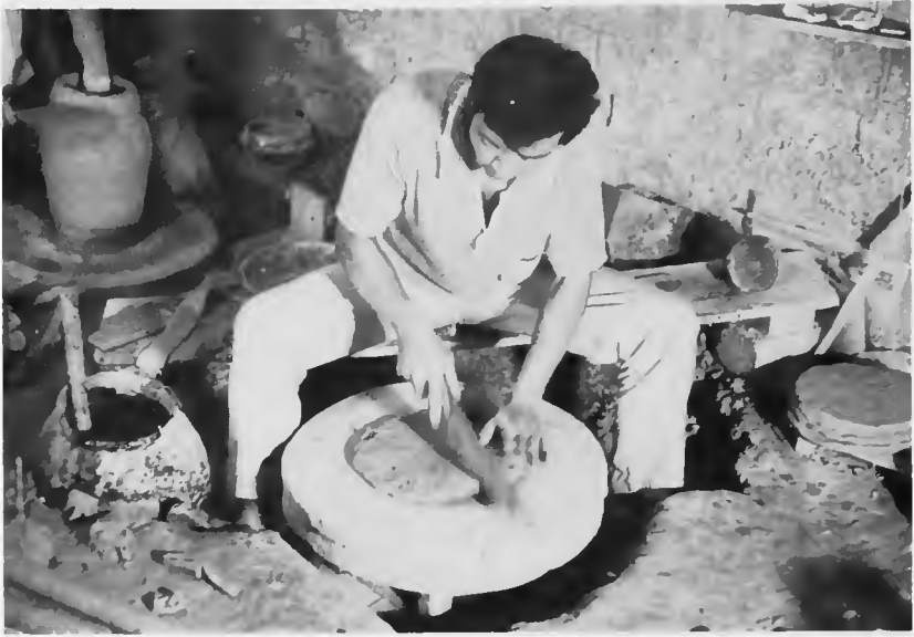
Figure 34b. Bottom disk flattened with wooden beater (pangmangi).
