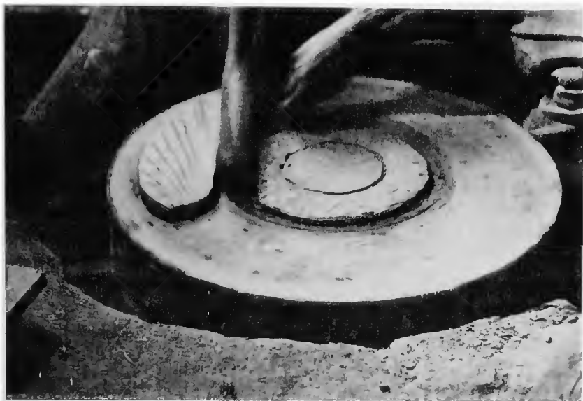
Figure 61b. Coil flattened before being mounted on base.
