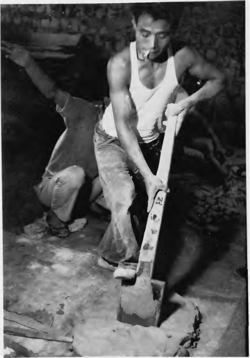
Figure 32. Worker cutting clay block with wooden shovel. (Photo by Ralph Rinzler, 1971.)
