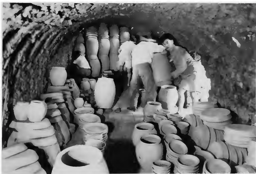
Figure 41. Men stacking interior of cannon kiln at Talsông Factory. (Photo by Ralph Rinzler, 1971.)
