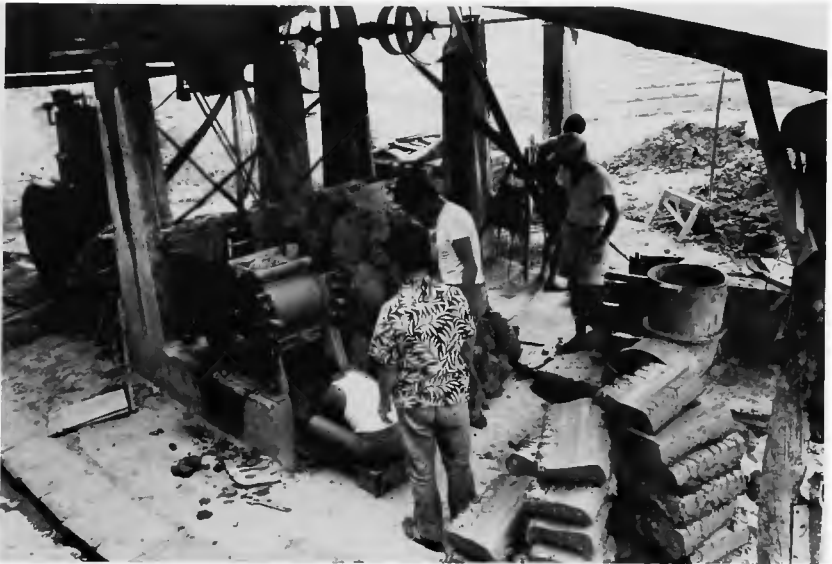
Figure 84. Rolling mill and clay extruder (right foreground) in equipment shed are connected to diesel engine (rear). Clays are washed before being processed through machines. (Photo by Ralph Rinzler, 1981.)
