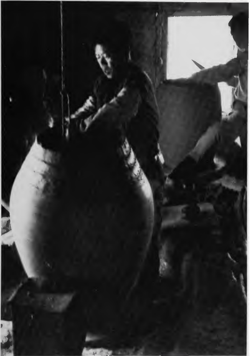
Figure 68. Potters manufacturing large rice or wine jars. Charcoal-filled heaters (foreground and suspended in vessel) stiffen cylinder wall as artisan works. (Photo by Ralph Rinzler, 1972.)
