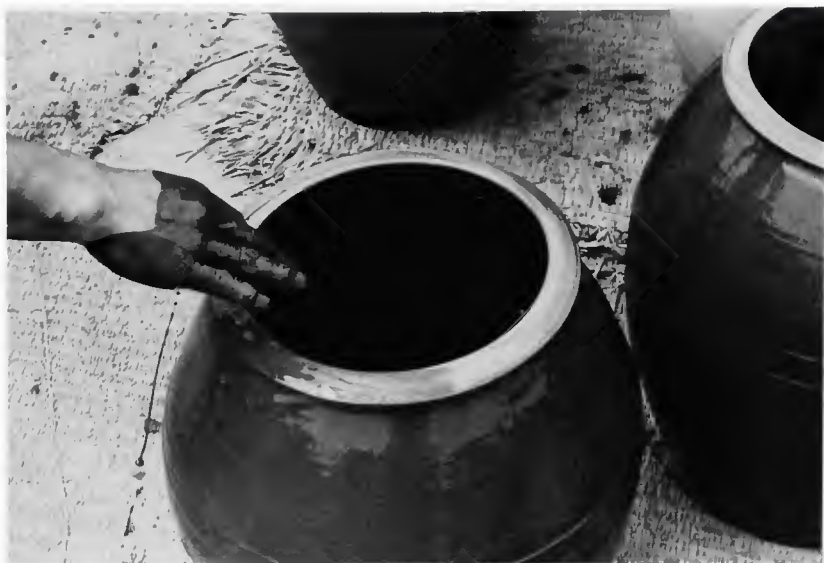
Figure 116. Wiping glaze from rim to prevent stacked jars from adhering during firing. (Photo by Ralph Rinzler, 1981.)
