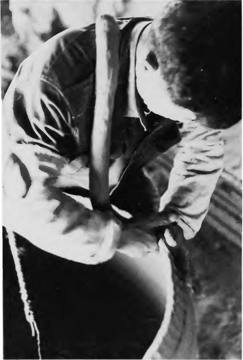
Figure 69. Curved stick extends potter's reach during making of large vessels. (Photo by Ralph Rinzler, 1972.)
