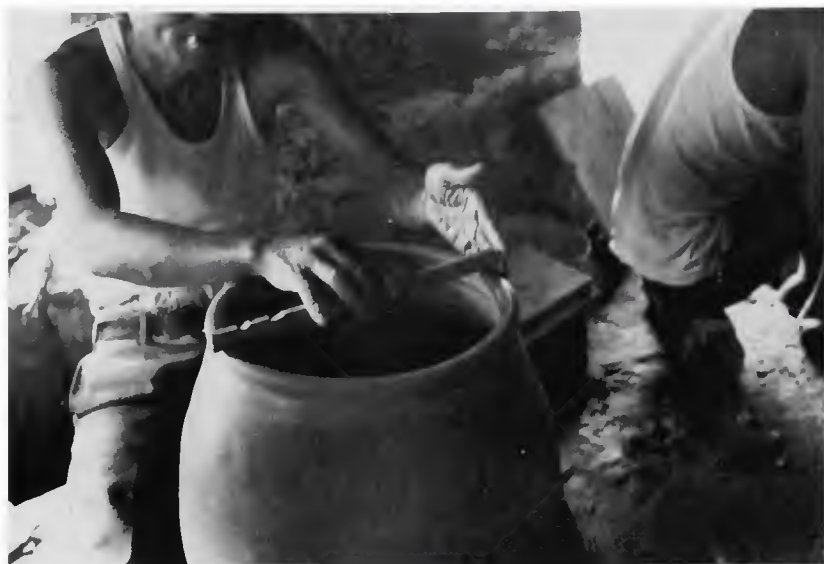
Figure 92m. Use of stick gauge ( chönjimdae ) ensures that mouth and bottom diameters are the same.
