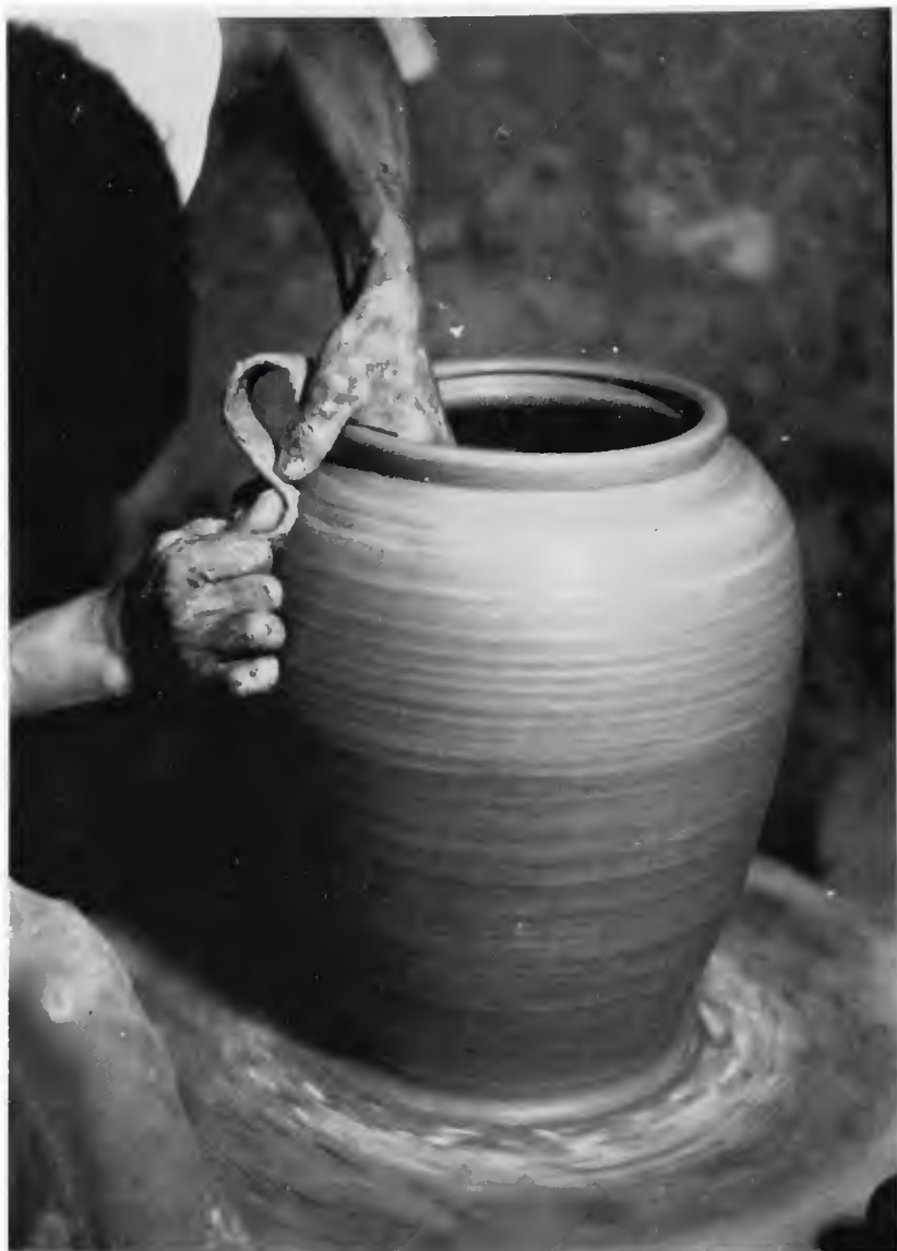
Figure 34h. Rim and shoulder of vessel formed with quilted cloth strip.
