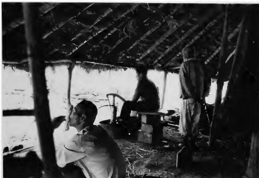
Figure 40. Supplemental oil is pumped through two pipes into mouth of kiln in Figure 38. (Photo by Ralph Rinzler, 1971.)
