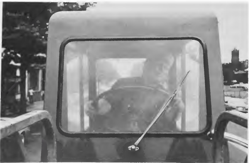
Figure 17. The tillerman steering the rear axle of the truck as he sits in the tillerman's cage.
