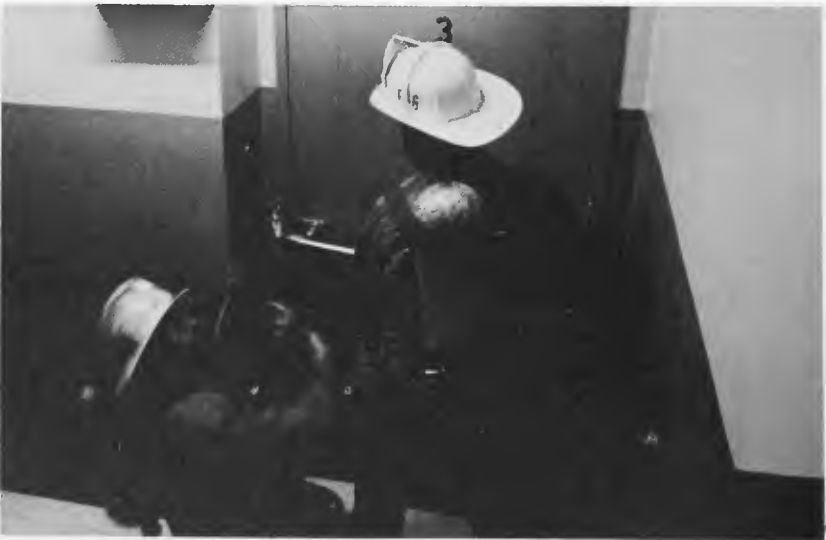
Figure 18. A halligan bar man and a member of the engine company gain forcible entry with the bar.
