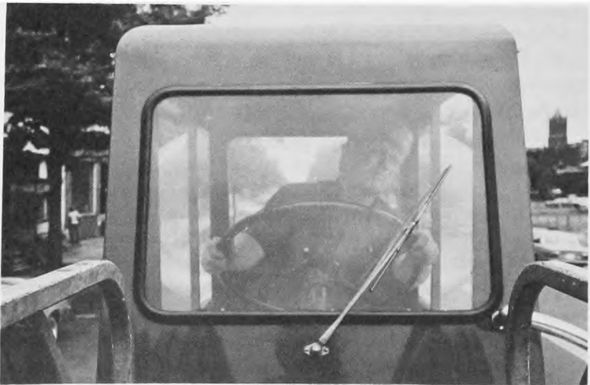
Figure 17. The tillerman steering the rear axle of the truck as he sits in the tillerman's cage.
