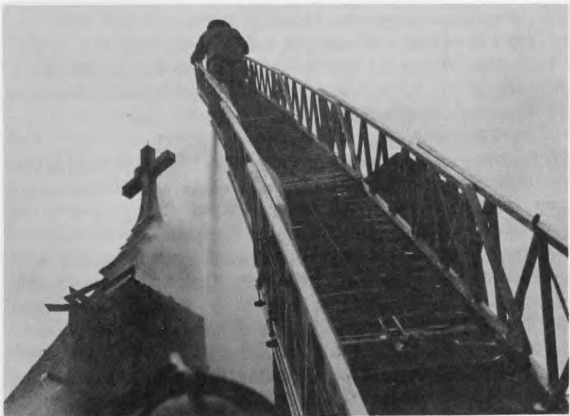
Figure 33. A member of the truck company operates the ladder hose pipe at the tip of the aerial ladder.
