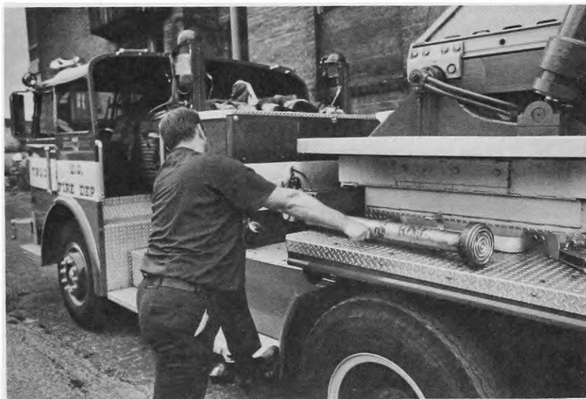
Figure 16. The truck driver begins to extend the aerial ladder by pulling the jacks* or outrigger supports that keep the turntable* stable while the ladder is extended.
