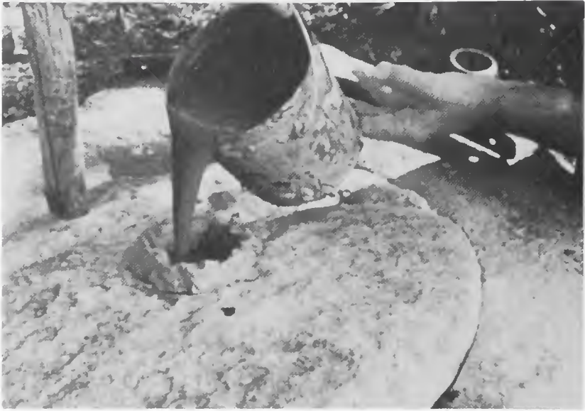
Figure 30. Pouring glaze through the center of the runner. (From the film, The Meaders Family: North Georgia Potters. )
