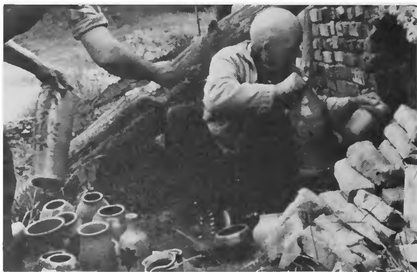
Figure 36b. Q, relaying the ware from the mouth of the kiln to an assistant.
