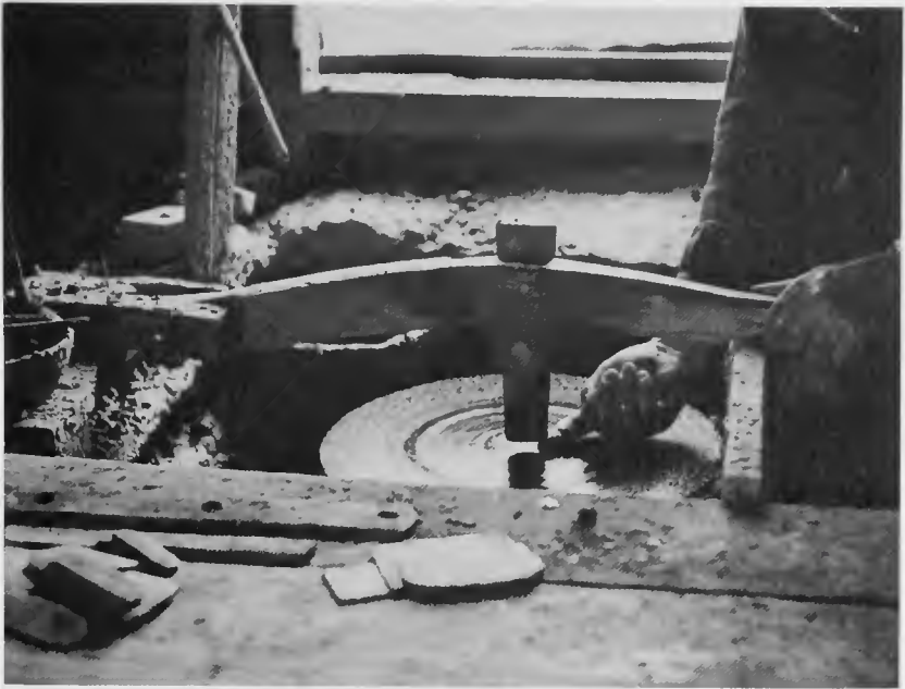
Figure 17. Crib assembly, showing ball opener/bottom gauge and height gauge. (Photo by Ralph Rinzler, 1978.)
