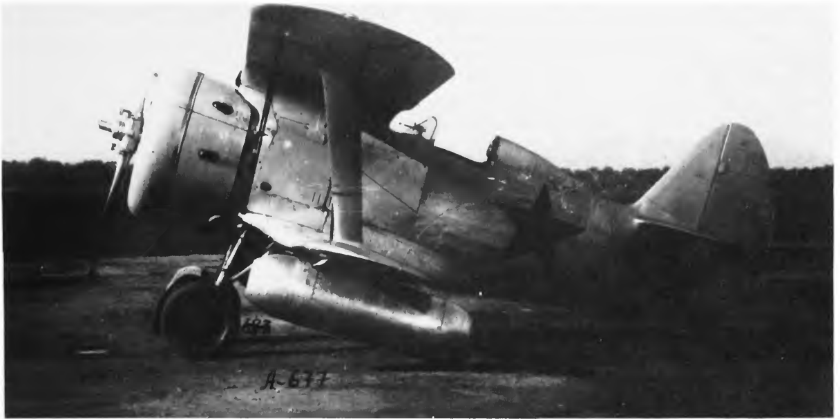
FIGURE 3.—DM-2 ramjet engines suspended beneath wings of N. N. Polikarpov aircraft I-15-bis (I-152), No. 5942.
