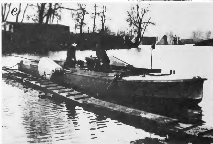
FIGURE 7.— a , Očenášek's water-jet propelled boat No. 1, showing exhaust nozzles; b , rear of boat No. 1; c , water-jet propelled boat No. 2; d , boat No. 3 during demonstration test; e , water exhaust ducts of boat No. 3.
