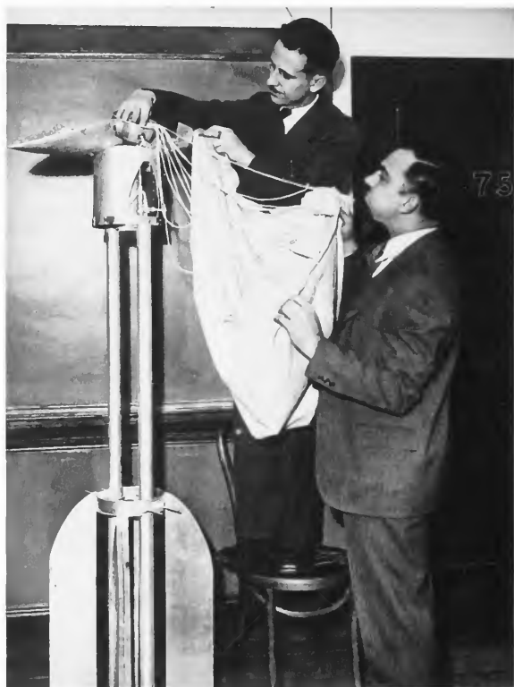
FIGURE 2.—ARS No. 1, during a demonstration and lecture at New York University (Washington Square Campus), in spring 1932. Hugh F. Pierce, who constructed the rocket, is packing the parachute in its container (made from a ten-cent-store saucepan) as G. Edward Pendray, co-designer of the rocket, holds the parachute. The cone-shaped nose was designed to open up at the height of the flight and eject the parachute. The parachute itself, made by Mrs. Leatrice M. Pendray from a scaled-down design for a professional aviation parachute, was of silk pongee. Photo from Pendray Collection, Princeton University Library.
