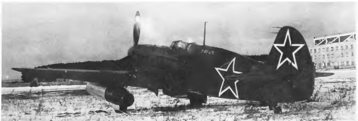
FIGURE 4.—DM-4 ramjet engines mounted beneath wings of A. S. Yanovlev aircraft Yak-7b to supplement performance.
