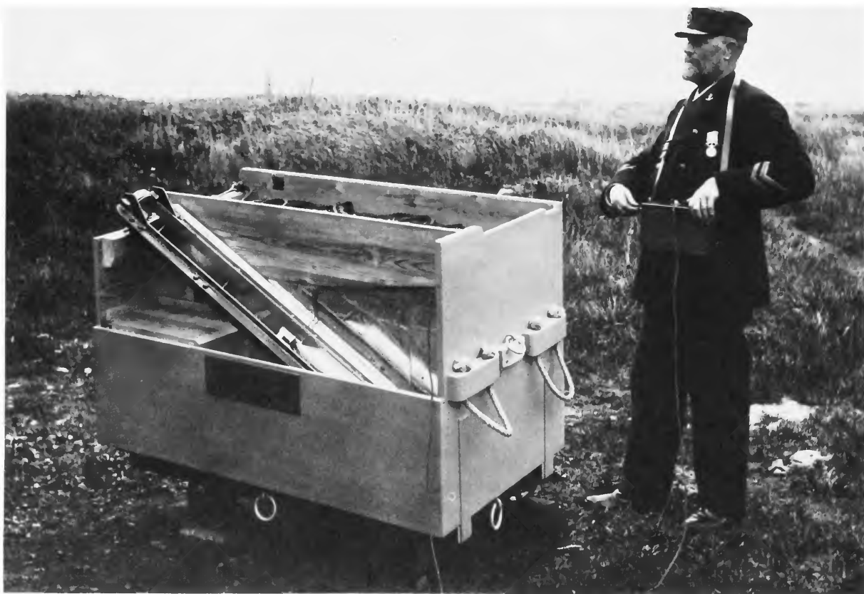
FIGURE 10.—Complete lifesaving rocket system, manufactured by the Mars Company. Photo from Armémuseum Archives, Sweden.
