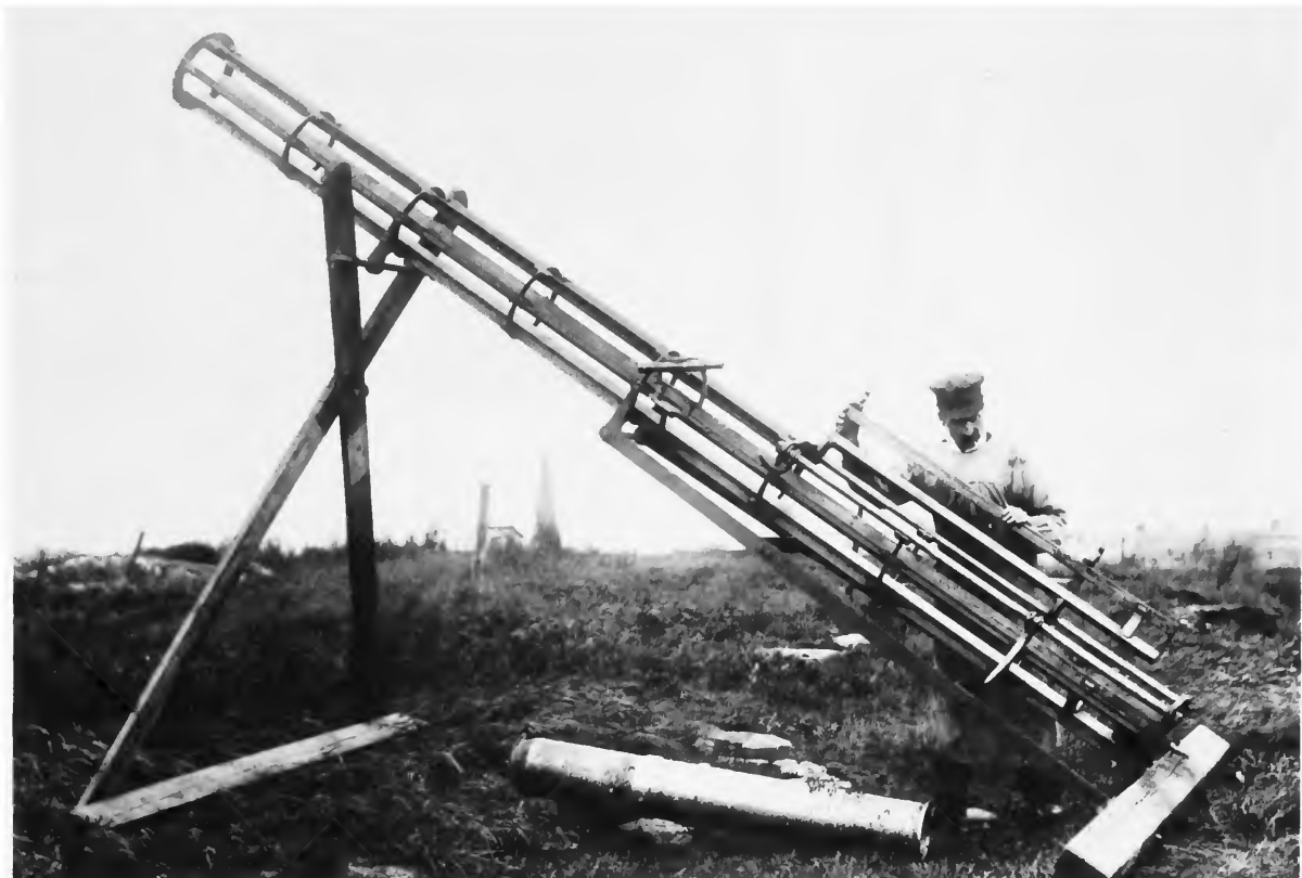
FIGURE 4.—The lightweight launching barrel consisting of cylindrically arranged guides. Photo from Armémuseum Archives, Sweden.
