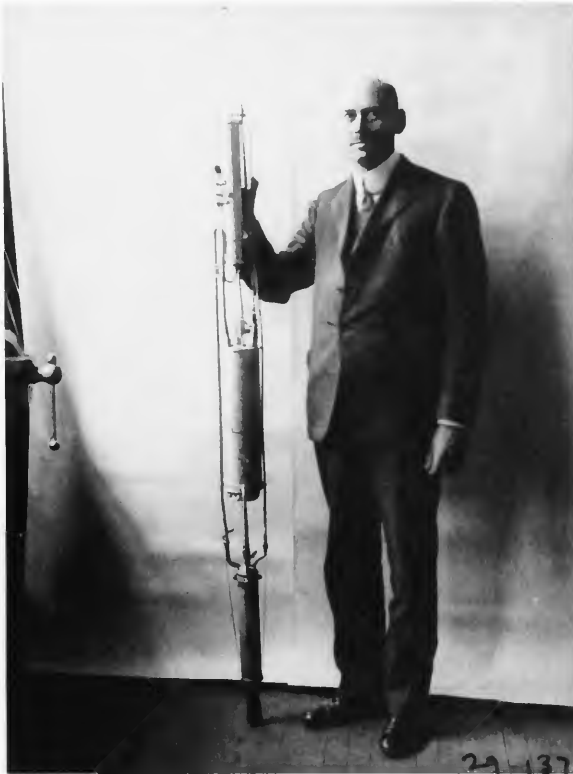
FIGURE 5.—Modification of rocket design in, now classic, configuration: motor at rear, surmounted by liquid oxygen and gasoline propellant tanks. Rocket is on exhibit at Smithsonian Institution.
