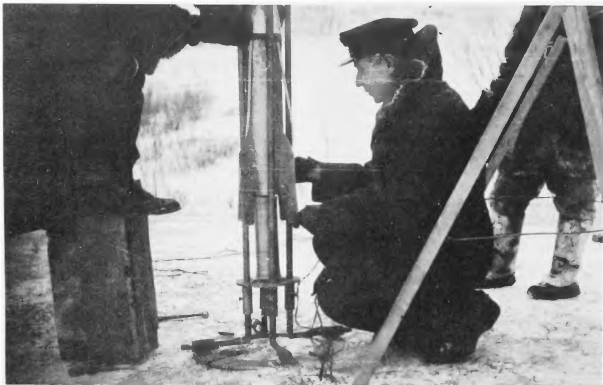
FIGURE 1.—Two-stage ramjet rocket being prepared on launching rack, showing first-stage solid propellant rocket below fins.
