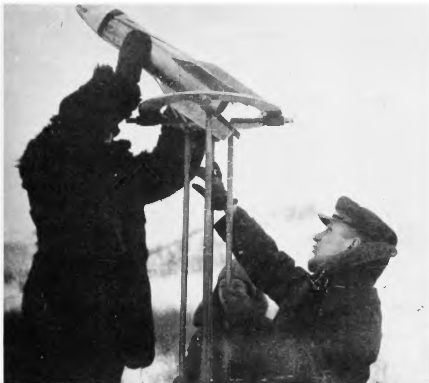
FIGURE 2.—Second stage of ramjet-rocket vehicle being lowered onto launching rack.
