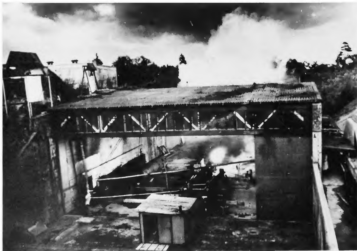
FIGURE 3.—Overall view of a 1000-kg, high-pressure combustion chamber experiment using cooling by evaporation. Propellant tanks are above the roof, to the left. The propellant pumps are directly underneath. Combustion chamber is in operation in center. Note the cloud of condensed cooling agent. The observation stand is above on the right.
