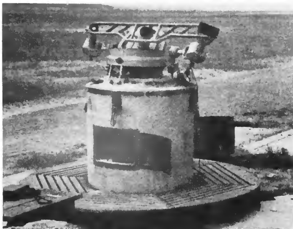
FIGURE 4.—First Askania cinetheodolite, used at the DFS-Darmstadt, Germany, 1935–39 for flight performance measurements. Photo courtesy R. Opitz.
