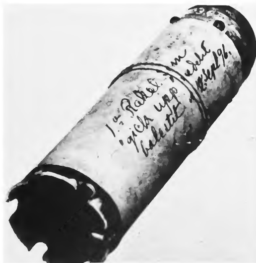
FIGURE 5.—The first known ballistite rocket, fired 12 September 1896 in Stockholm. In Tekniska Museet, Stockholm.
