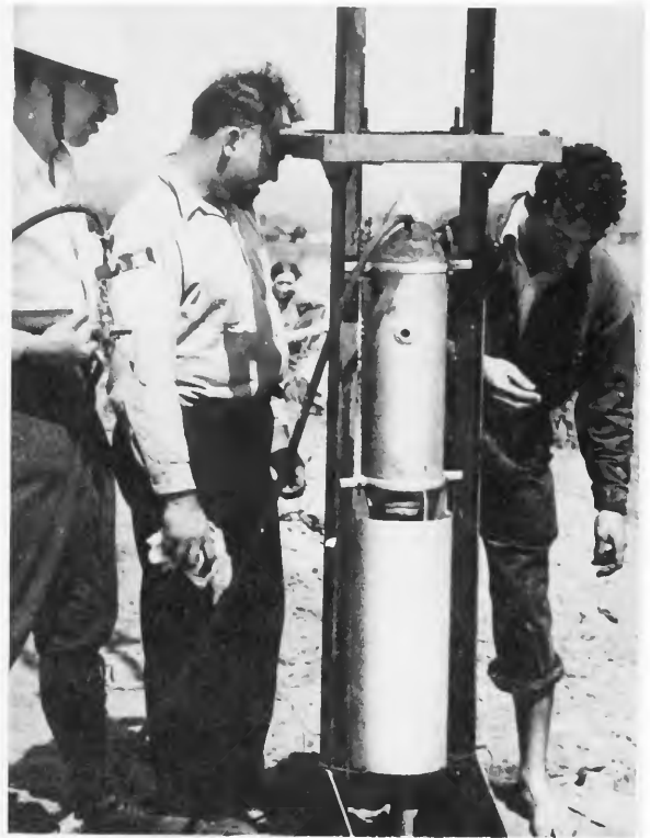
FIGURE 9.—ARS Rocket No. 3, at Marine Park for launch attempt in September 1934. From left, Shesta, Pendray, and Smith. The gasoline tank is being pressurized with nitrogen through a valve in the cone. The oxygen fill-hole is visible just below the pressure inlet. Photo from Pendray Collection, Princeton University Library.
