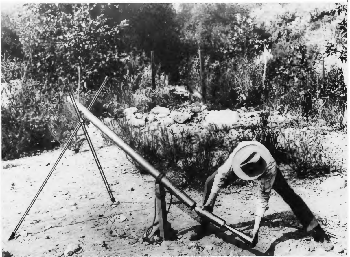
FIGURE 2.—Goddard inserts 3-inch rocket in lightweight tube launcher. Demonstration tests were made at Aberdeen Proving Grounds, 6–7 November 1918.
