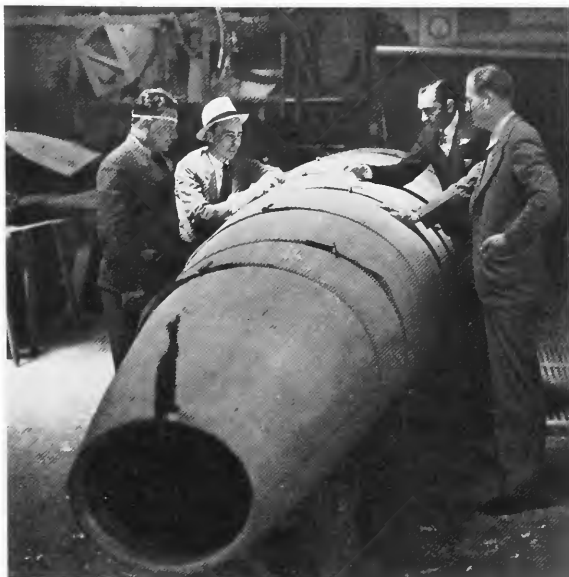
FIGURE 40.—Wiley Post, left, at the Lockheed factory in Burbank, studies the fuselage-construction method used for Vega fuselages. The two half shells of the wooden fuselage were glued together as shown. Second from left is Bill Parker, third is Carl B. Squier, general manager, and on the far left is Richard Von Hake, works manager. (Courtesy Lockheed Aircraft Company.)
