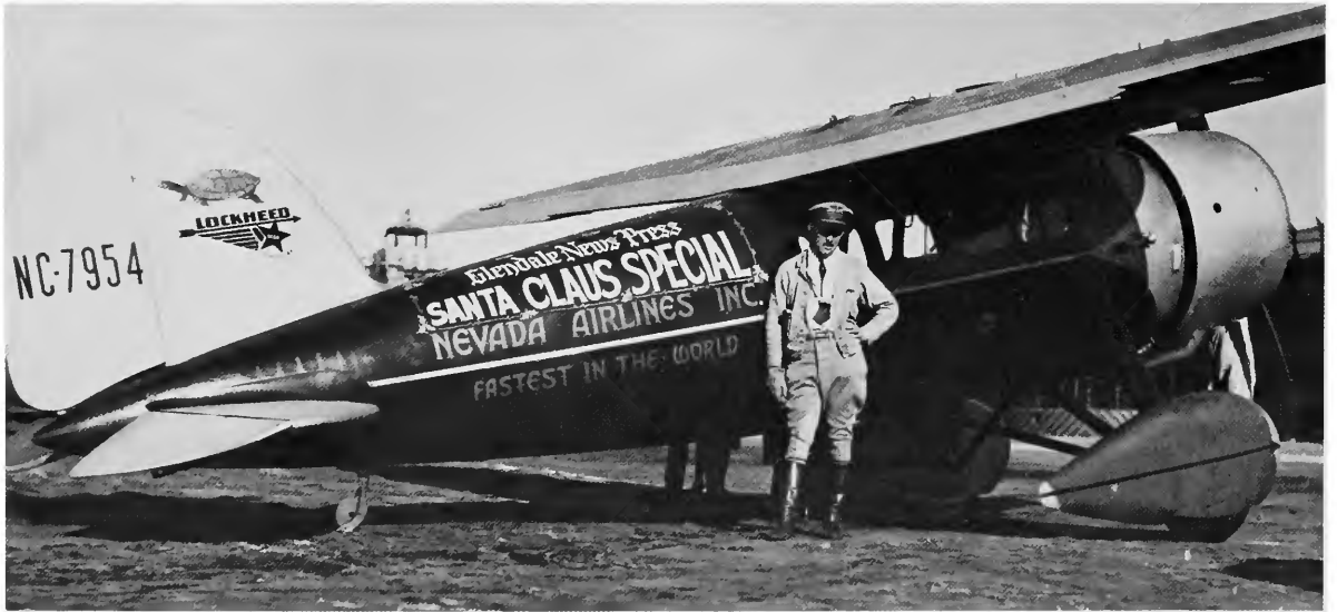
FIGURE 14.—In 1929 F. C. Hall sold the first Winnie Mae (NC 7954) back to Lockheed, who in turn sold the aircraft to Nevada Airlines. The Vega was equipped with a N.A.C.A. cowl and wheel pants, and was renamed “Sirius.” “Captain” Roscoe Turner (later “Colonel”) flew the aircraft in the 1929 air races, coming in third in the free-for-all speed contest, at an average speed of 163.44 miles-per-hour (mph), behind Doug Davis, first, (194.90 mph in a Travel Air) and R. G. Breen, second, (186.84 mph in a Curtiss P-3-A). (Courtesy Lockheed Aircraft Company.)
