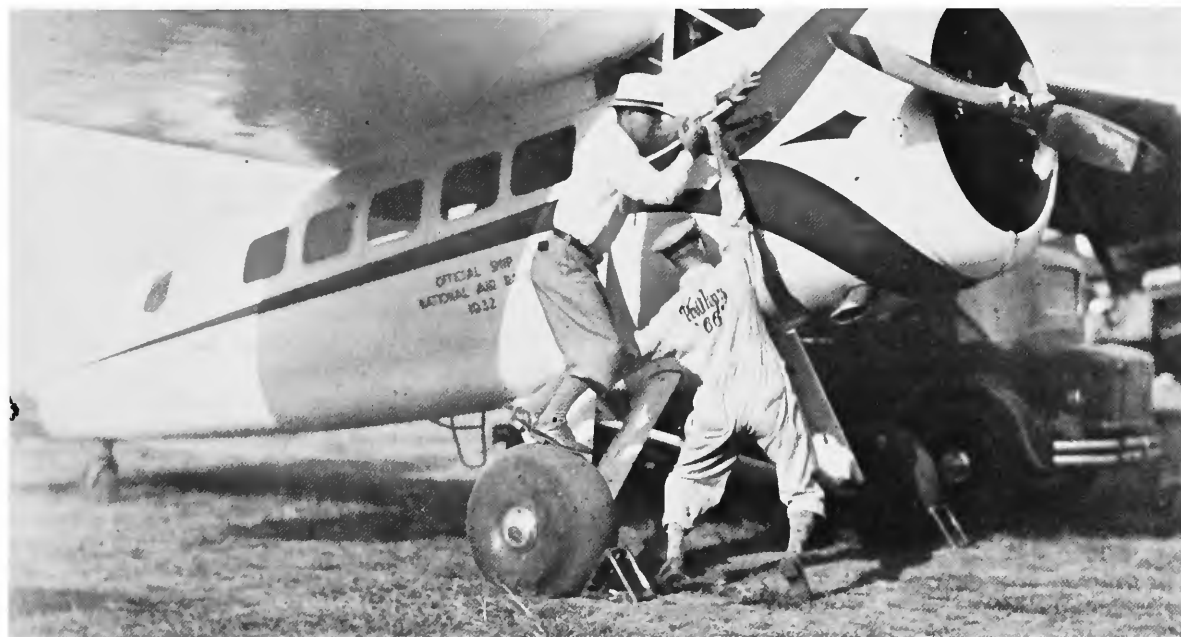
FIGURE 42. —Billy Parker’s Lockheed Vega is started by hand-cranking the inertial starter at the National Air Races, 1932. The mechanic on the right is Fidel “Pancho” Vela, who maintained Parker’s plane. (Courtesy Phillips Petroleum.)
