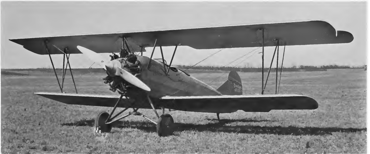
FIGURE 12.—A 1928 Travel Air Model 4000 with a Wright J-4 engine of 200 horsepower represents the type of three-place biplane purchased by F. C. Hall and Powell Briscoe, the Oklahoma oilmen who gave Wiley Post his first job as an executive pilot late in 1927. (Courtesy Beech Aircraft Co.)
