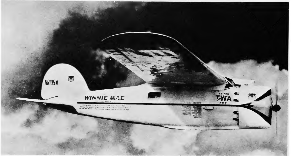
FIGURE 110.—The ultimate in Lockheed Vega beauty and advanced equipment is achieved in the 1935 supercharged version of the Winnie Mae . Post spent more flying hours in the stratosphere by June 15, 1935, than any other man. While in the jet stream during these flights, he traveled at sustained ground speeds in the vicinity of 300 miles per hour for periods longer than any other person had accomplished. Note that to reduce as many aspects of air drag as possible, not only has the landing gear been dropped, but the rudder has been decreased in size and even the tail skid has been dropped. (Courtesy Lockheed Aircraft Company.)
