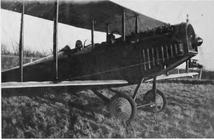
FIGURE 11.—J. Bart Scott (rear seat) and Wiley Post (front seat) prepare to take a spin in one of Scott's Canucks, 1927. Behind them, a contemporary Model T Ford proceeds along a country road. Note that the tire-inflation valves are on the inside of the wheels. (Courtesy J. Bart Scott.)
