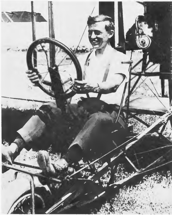
FIGURE 5.—This is the dynamic Art Smith preparing for an exhibition flight. The early Curtiss Pusher had certain novel control linkage features which differed from other aircraft of that time and from later aircraft. The shoulder straps are fastened to lateral arm supports that pivoted at the seat level. This mechanism was then connected with the ailerons (located between the wings) that were operated by leaning the torso to one side or the other for banking the aircraft. The wheel was connected to the rudder used for yaw. The fore and aft motion of the wheel worked the horizontal tail for pitch up or down. On the wheel yoke was a spark-advance and retard lever and on the wheel was an on-off ignition switch. The engine throttle worked with a foot attachment (for details see U.S. Naval Institute Proceedings , July 1971, pages 34–43, article by Thomas Ray). Smith wears corduroy trousers and high buckle shoes. (Courtesy Will D. Parker.)
