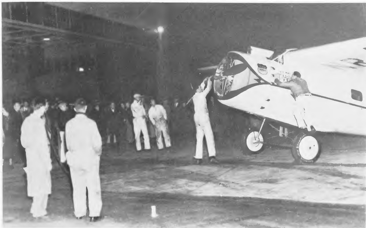
FIGURE 109.—The Winnie Mae is being hand started in the early morning hours at Burbank, California, February 22, 1935, in preparation for the start of a transcontinental stratosphere flight. Wiley Post is in his pressure suit in the cockpit. The droppable landing gear is in place, suspended by force and aft cables that Post could release after takeoff by a lever in the cockpit. This version of the Winnie Mae did not have an electrical system, hence the hand cranking (the radio compass was powered by dry cells). The man standing on the wheel is feeling the exhaust air as the propeller is rotated. The propeller tips were color coded so that, in preparation for the dead-stick landing, the propeller could be positioned horizontally with a specific blade on one side (by a special crank inside the cockpit) so that the crankshaft counterweight would be down, thus minimizing propeller rotation possibly induced by landing bumps. (Courtesy Lockheed Aircraft Company.)
