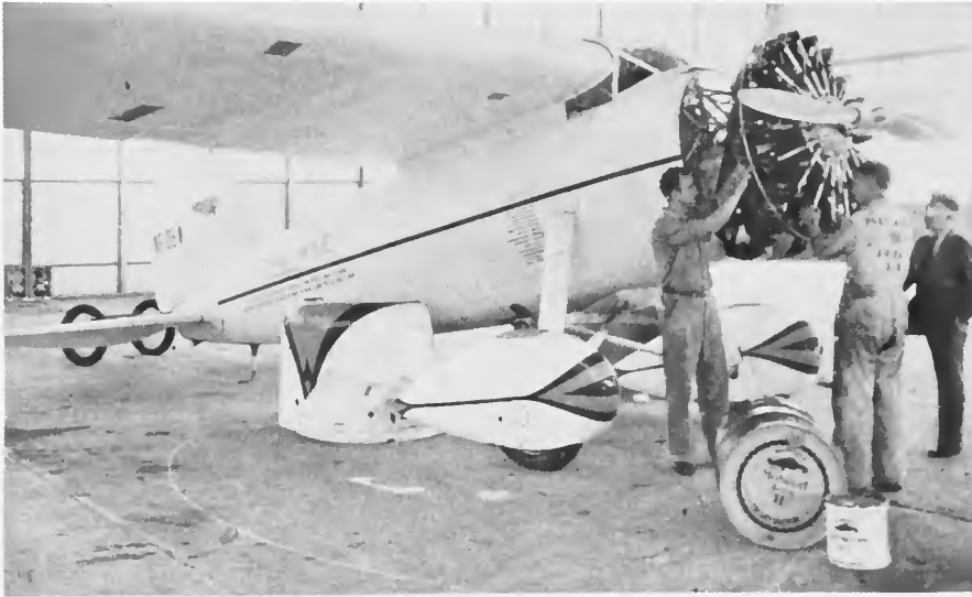
FIGURE 48.—The Wasp engine of the Winnie Mae is readied for the 1933 solo world flight by Pratt and Whitney mechanics, as Post watches. (Courtesy Pratt and Whitney Aircraft.)
