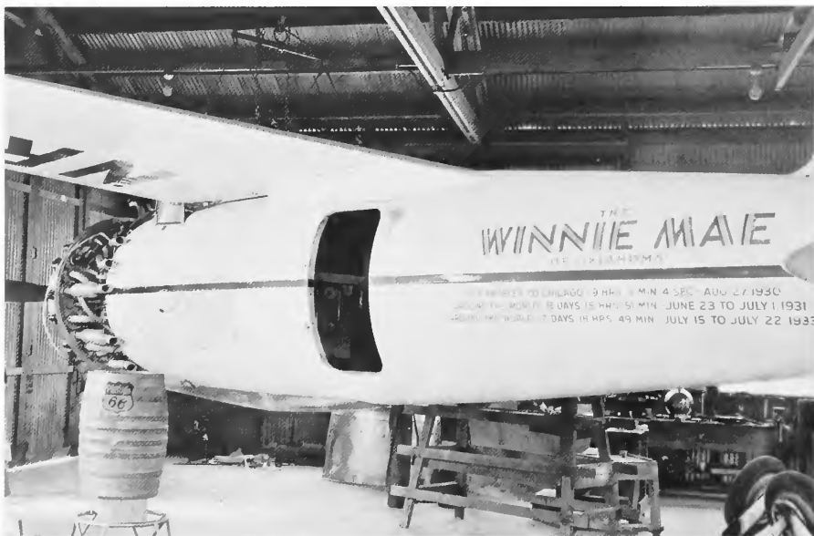
FIGURE 96.—The Winnie Mae is shown being prepared for a transcontinental stratosphere flight. This photograph was made in January 1935 at the original Lockheed hangar in Burbank. This hangar had been a "glass factory" prior to its use by Lockheed. The cowling has been removed and cleaned of paint (seen on floor behind fuselage). The aircraft is suspended by pulleys from a ceiling beam by utilizing the hoist eye hooks on the upper wing. The belly-landing skid made of spruce has been glued in place and is now metal clad. Under the rear fuselage in the background on the workbench is the spherical container for the liquid oxygen. (Courtesy Phillips Petroleum.)
