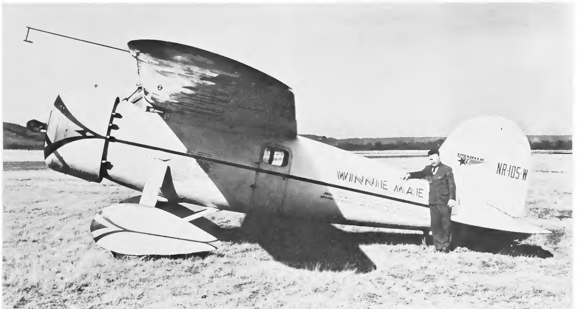
FIGURE 94.—Wiley Post and his Lockheed Vega, the Winnie Mae . Picture made at Bartlesville, Oklahoma, late in 1934. Note that Post has picked up some weight since the time of the 1933 picture at Floyd Bennett Field. Note also that he has provided the Wasp engine with a separate exhaust stack for each cylinder, a recent modification he devised at the time to facilitate cylinder purging. (Courtesy Phillips Petroleum.)
