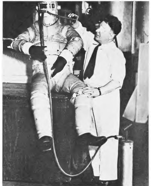
FIGURE 72.—Wiley Post's second pressure suit is shown during a static pressure test at the B. F. Goodrich Company in Akron, Ohio. This pressure suit was the first to employ flexible elbow and knee points. The suit was entered through the waist, which was sealed with two large metal plates held together with wing nuts. The oxygen was brought in just below the visor. Post had to be cut out of the suit when he became stuck in it. Photograph made in July 1934. (Courtesy Popular Mechanics Magazine.)
