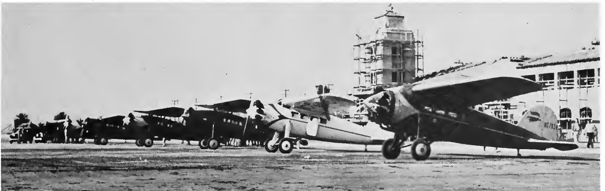
FIGURE 13.—The original Winnie Mae , Lockheed Vega NC 7954, is shown in 1928 at Grand Central Airport, Glendale, California. NC 7954, completed on August 12, 1928, is at the far right. The second aircraft to the left is another Vega, with two Lockheed Air Express Aircraft as numbers three and four. The remaining aircraft are Vegas. Note that the N.A.C.A. engine cowlings were not used at this time. Wheel pants also were not used. The construction work that was progressing on the terminal building is clearly evident. (Courtesy Lockheed Aircraft Corporation.)
