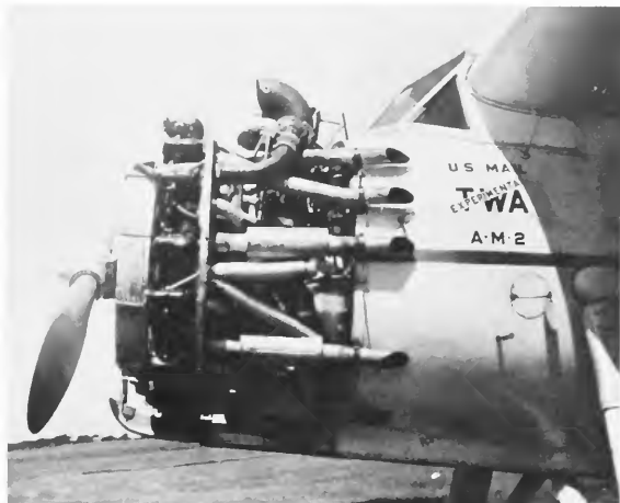
FIGURE 99.—The uncowed Wasp engine of the Winnie Mae reveals features added for stratosphere flight. The air scoop and its circular, external supercharger are shown atop the engine just forward of the windshield. The “intercooler” radiators that remove heat from the air derived from the external supercharger are between the propeller and the cylinders. Each cylinder is equipped with its own exhaust stack, some stacks surrounded with shrouds to provide heated air. The wooden, metal-clad landing skid is shown. The triangular, left cockpit window is partially open. A tag is shown on the circular cover for the special oil-tank filter opening just forward of the main landing gear fuselage attachment. The aircraft is being readied in California during January-February of 1935 for the forthcoming February transcontinental stratosphere attempt. (Courtesy Ernest Shults.)
