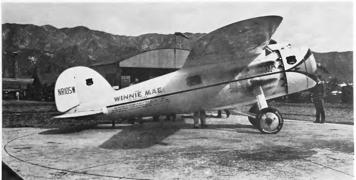
FIGURE 105.—The Winnie Mae without droppable gear (but with the belly skid in place) is shown at Burbank after a test flight. The dark exhaust marks on the fuselage were not unusual following a long flight. (Courtesy Phillips Petroleum.)
