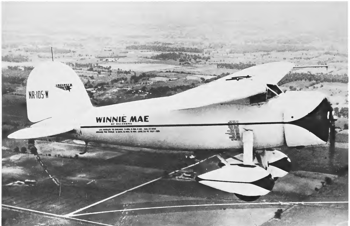
FIGURE 55.—The Winnie Mae is shown ready for the around-the-world solo record flight attempt. The “sense” antenna post on the fin is clearly evident. (Courtesy Jimmy Gerschler and Smithsonian Institution.)
