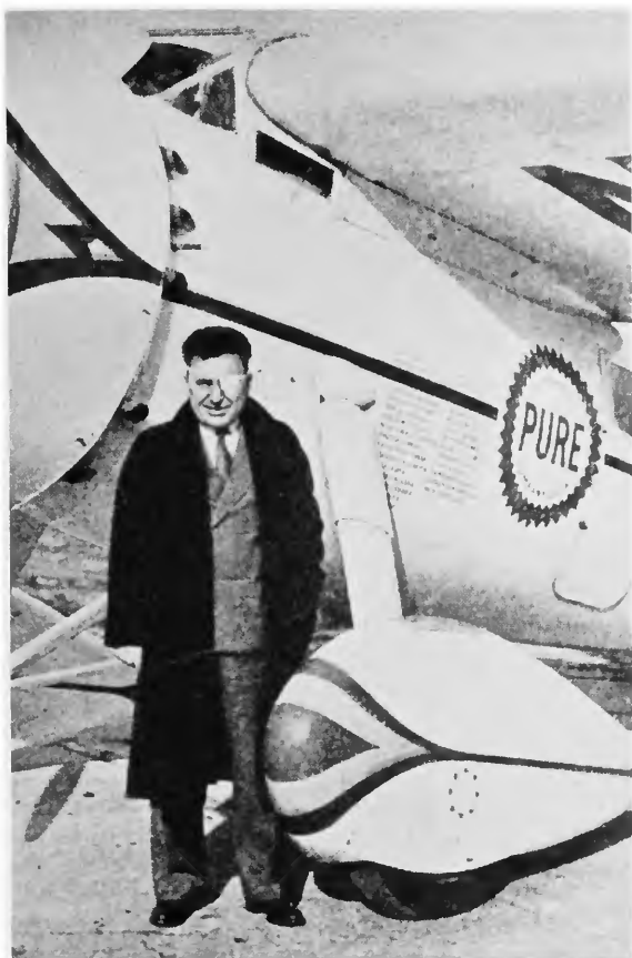
FIGURE 79.—The Winnie Mae in early September 1934, as used in the high-altitude flight-record attempts at Chicago. The sponsoring Pure Oil Company emblem is prominently displayed. The exhaust stacks are separately vented by cylinder and an “external” Bendix supercharger has been added to the top of the Pratt & Whitney Wasp engine. The separate exhaust stacks reduced back pressure, and enabled an increase in horsepower, as well as more efficient engine cooling. (Courtesy Pure Oil Company.)
