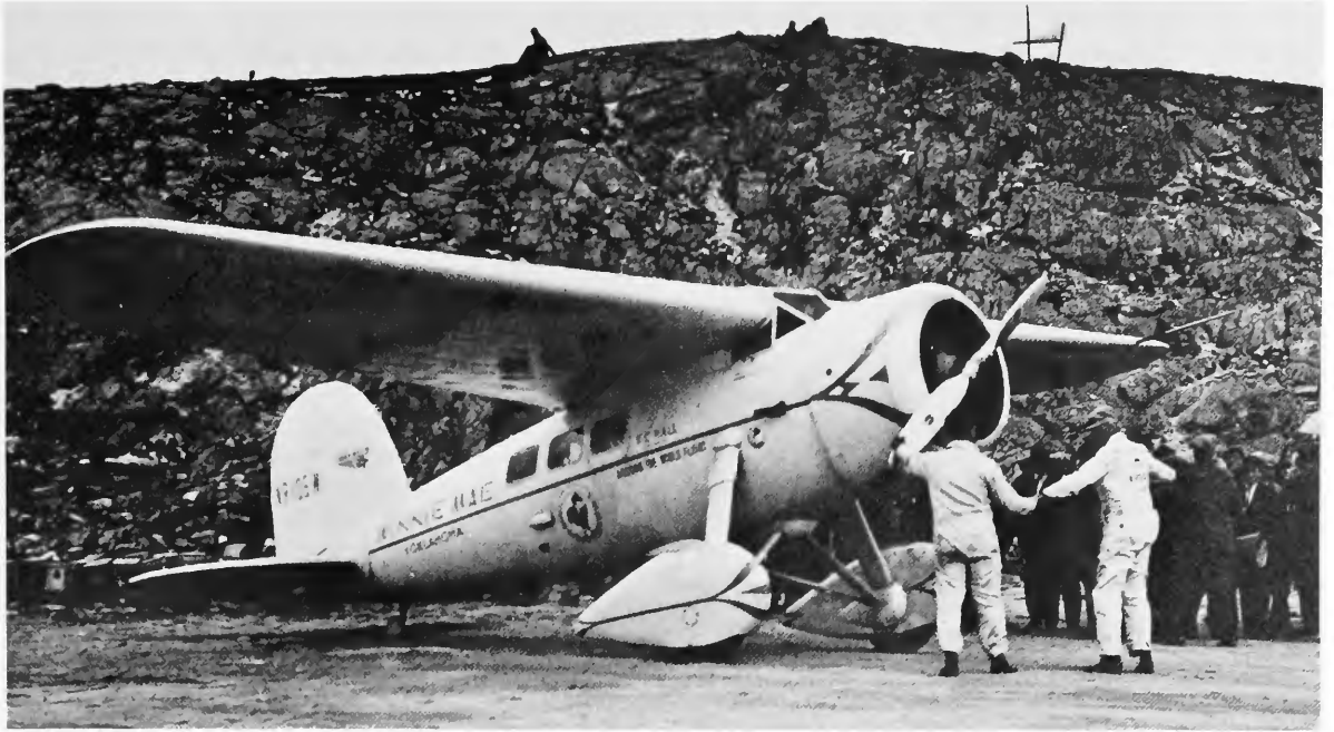
FIGURE 22.—On June 23, 1931, Post and Gatty landed at Harbour Grace, Newfoundland, after a 6-hour 47-minute flight from New York City. After refueling, they were given a hand start (one man pulled another, who held the lower propeller blade) and took off for England. The aircraft at this time did not have a starter motor. Gatty's drift and
