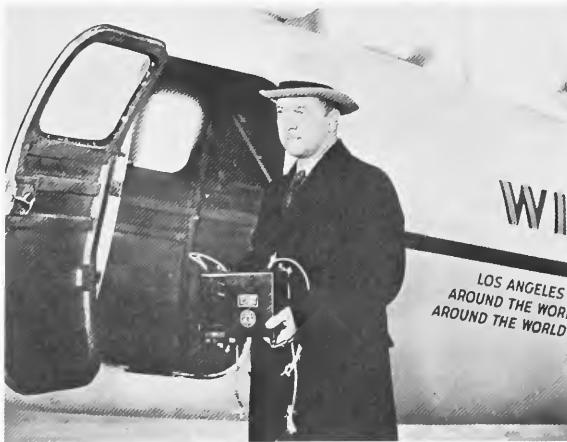
FIGURE 87.—A. M. Alcorn, Civil Aeronautics Administration inspector, prepares to install one of two sealed barographs in the fuselage of the Winnie Mae in December 1934, at Bartlesville, Oklahoma. These barographs were used in official record attempts in accordance with National Aeronautic Association procedures (note NAA initials on container). Shock cords for mounting are attached to the top of the barograph. (Courtesy Phillips Petroleum.)
