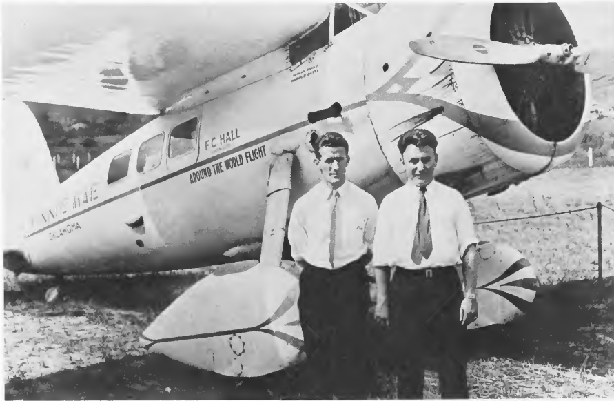
FIGURE 38.—Gatty and Post are seen after their 1931 around-the-world record flight. Note the oil-streaked cowling of the Winnie Mae . The small hole in the cowling above the trim is for the crank that spins the hand-inertial starter. The venturi tube just aft of the cowling above Gatty's head is for Gatty's duplicate set of gyroscopic flight instruments. The airscoop for cooling Post's feet is seen just above Gatty's right ear. The Pathé rooster emblem on the fuselage has been painted over but still shows slightly through. Gatty's drift and ground-speed instrument ports are shown under the rear windows. The propeller is a fixed-pitch Hamilton Standard. The right-wheel pant has a metal cover on top for a fuel-handler step. The attachment point to the wheel axel is shown with eight screws, while below this, the cover for the tire inflation valve is shown. The aircraft is roped off for protection. On this flight, Post confirmed his theory that the "variance in time" would disrupt his body biological rhythms and derogate flight performance. He was the first to publish on this phenomenon, which later became known as "circadian rhythm disruption." (Courtesy Lockheed Aircraft Company.)
