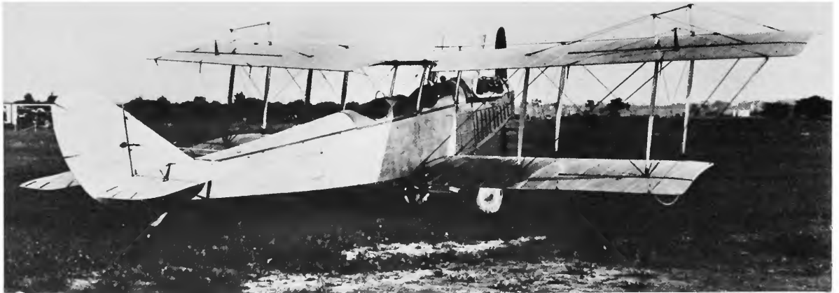
FIGURE 8.—The Curtiss “Canuck,” Canadian version of the famous Curtiss JN-4 “Jenny” military training airplane of World War I, became a popular barnstorming airplane in the 1920s. The Canuck was typically powered by a Curtiss OX-5 engine of 90 horsepower, which gave the airplane a 60-mile per hour cruising speed with a 45-mile per hour stalling speed. The Canuck had ailerons on both wings, which gave it a more rapid roll rate than the American Jenny. The OX-5 engine was a water-cooled, eight-cylinder engine that consumed nine gallons of fuel per hour. The fuel tank capacity was 20 gallons. (Courtesy Smithsonian Institution.)
