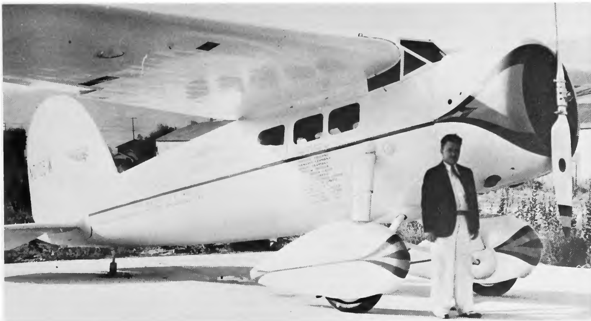
FIGURE 41. —Wiley Post stands before the beautifully reconditioned Winnie Mae , August 1932, Burbank, California. The propeller is of the fixed-pitch variety, and the lower right wing sports a retractable landing light (the light and the other, in the left wing, was extended manually or by an electric motor). The airplane is now in the “commercial” category (NC 105W). Note that the listing of the 1931 landings is lined up on the left margin, and that the exhaust is emitted at the lower side of the cowling. The Winnie Mae is on a “compass rose” at the airport. (Courtesy Lockheed Aircraft Company.)
