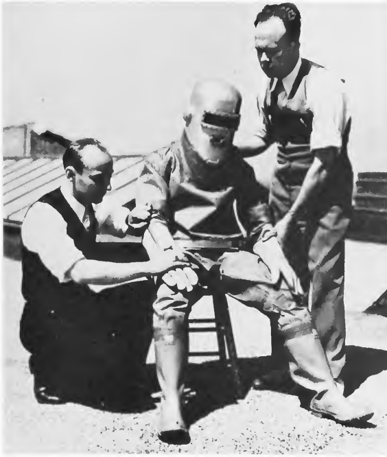
FIGURE 71.—W. R. Hucks (standing) and J. Stevens, of the B. F. Goodrich Co., in Los Angeles, scrutinize Wiley Post's first pressure suit, which they had just completed to his specifications. Photograph taken in June 1934. A laboratory assistant is in the suit and the helmet's mouth opening for food intake and speaking (during unpressurized periods) is shown with open cover. The suit was discarded when it ruptured during static tests at Dayton, Ohio. R. Colley of B. F. Goodrich kept the helmet, which is on display now at the Smithsonian Institution. (Courtesy NEA.)
