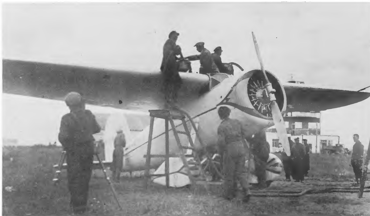
FIGURE 58.—A crew of Russians energetically and efficiently refuel the Winnie Mae at Novosibirsk on July 18, 1933. Note that the left- and right-wing tanks are being filled through chamois cloths to remove any contaminating water. A photographer in the left foreground records the event. Post stated that he got excellent service in Russia and received a very warm welcome at each stop, including Moscow, the preceding stop, where he made an unscheduled landing. The Chief of Transaviation, Mr. A. Petrov, requested the chief of the West Siberian Administration and the chief of the Far Eastern Administration to give full assistance to Fay Gillis and Wiley Post regarding the flight. (Courtesy Fay Gillis Wells.)
