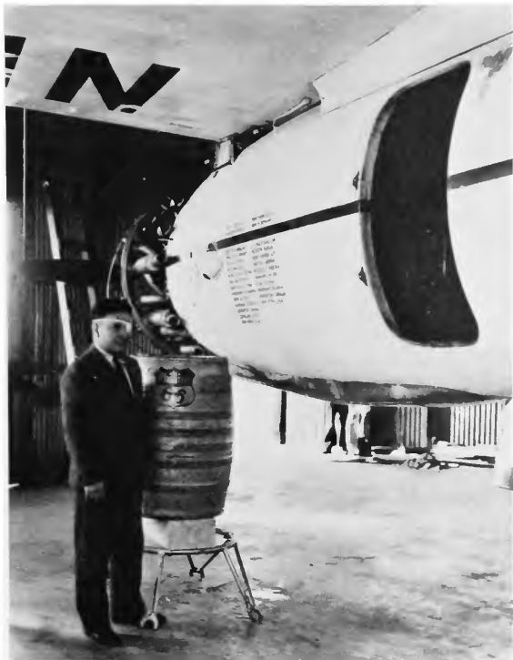
FIGURE 97.—Post poses by the evolving long-distance stratosphere modification of the Winnie Mae . The fuselage fuel tanks are seen through the door. The tubing at the wing root is a fuel line. (Courtesy Phillips Petroleum.)
