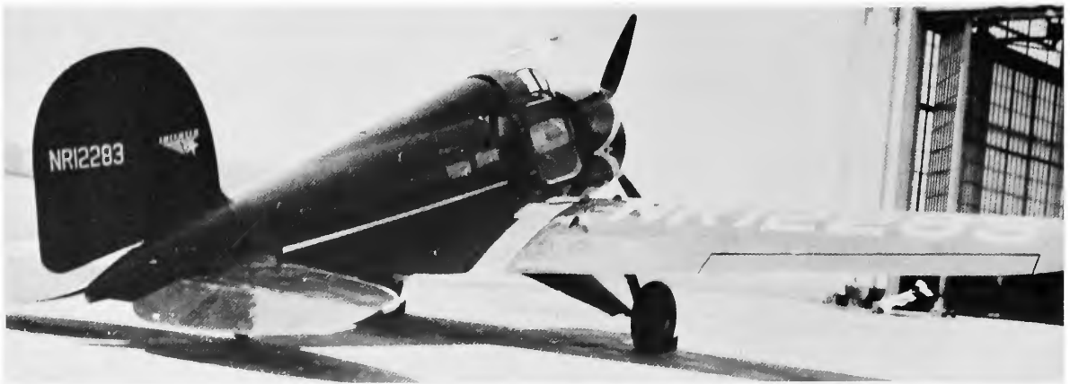
FIGURE 121.—The racy, new hybrid airplane obtained by Post in the spring of 1935 was assembled from the fuselage of a damaged second-hand Lockheed Orion, and the wings of an experimental Lockheed long-distance aircraft, an Explorer. This Explorer had cracked up in the Canal Zone and had not been tested for a type certificate by the Bureau of Aeronautics of the Department of Commerce. The combination of the Explorer wing (six feet longer than that of the Sirius or Orion) with the Orion fuselage and tail produced an uncontrollable, nose-down pitching moment at low air speeds and low power settings. The substitution of improper floats for wheels aggravated an existing nose-heaviness. The Lockheed Company did not countenance this unusual airplane. Note the fixed landing gear (Orions had retractable main wheels). (Courtesy Edwin O. Cooper.)
