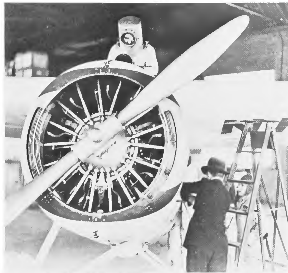
FIGURE 85.—Wiley Post eases into the cockpit with his pressure suit donned. The butterfly valve for the external supercharger is closed and may be seen just below Post's faceplate. The large grids seen in the front portions of the cowling on the left and right sides are the intercoolers that enabled the air compressed by the external supercharger to be cooled prior to entering the updraft carburetor in the lower, rear portion of the engine. The pressurized ignition harness may be seen. Billy Parker (back to view) is checking the oil filler area. (Courtesy Phillips Petroleum.)
