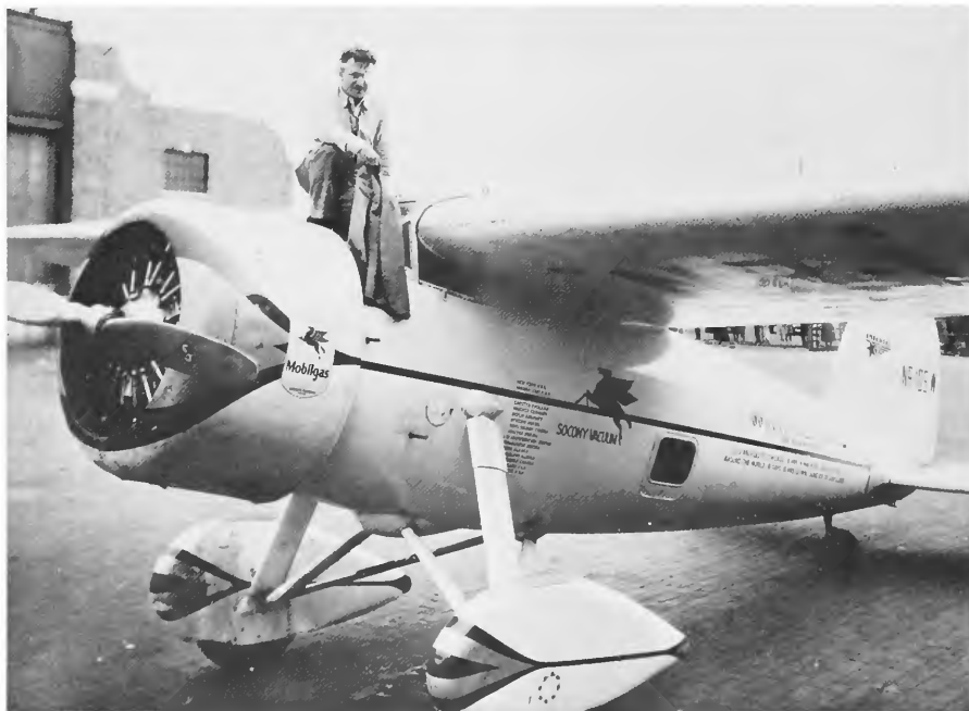
FIGURE 65.—This view shows the Winnie Mae at Floyd Bennett Field with a battered wing leading edge and dented wheel pants and cowling, illustrating the scars of the 1933 solo world flight. The two steps for mounting or climbing down from the cockpit are extended. The steps could be moved in or out from either inside the cockpit or outside the aircraft. An unusual feature is the tail wheel, which Post did not prefer. His traditional tail skid gave much more stability with respect to ground handling during landing roll-outs, especially in crosswinds at short fields. However, some "grass-strip" airport operators objected to tail skids, due to the "furling" that was produced. The top of each wheel pant is metal clad to withstand foot-pressure without damage to the finish. (Courtesy Mobil Oil Corporation.)
