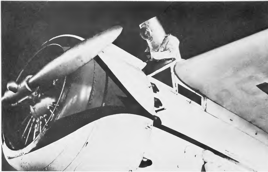
FIGURE 86.—Wiley Post, in his final pressure suit, smiles as he enters the top cockpit hatch of the Winnie Mae at Bartlesville, Oklahoma, December 1934. The Winnie Mae was placed within the Phillips Petroleum Hangar for this suit-cockpit compatibility test. The transparent faceplate is off the helmet and was not screwed on until climbing past approximately 17,000 feet. The fuselage landing skid is not in place at this time, but was added in January 1935 in California. The photograph was made by Frank Griggs of Bartlesville, Oklahoma. Note that the top retractable step is still out (just beneath the second exhaust stack) while the other lower step has been retracted. The top step could be retracted or extended from within the cockpit. The lower step was pushed in by foot. The oil filter cover is in place in front of the landing gear attachment. (Courtesy Phillips Petroleum Company.)
