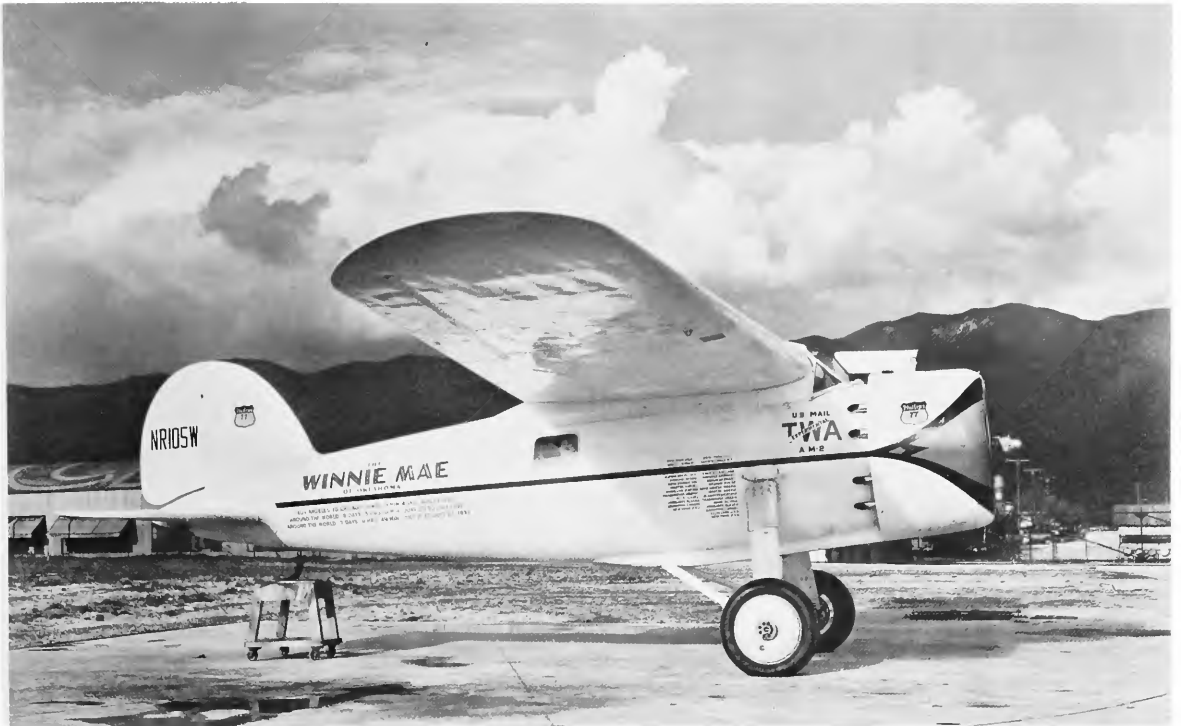
FIGURE 104.—The Winnie Mae is shown on the compass rose at Burbank. It has been placed in the cruising-flight position through the use of a dolly under the tail skid. The Trans World Airline U.S. Mail symbol is shown under the cockpit window. This references airmail contract #2. Post received sponsorship from both Phillips Petroleum and TWA for his long-distance stratosphere flight plans. (Courtesy Phillips Petroleum.)
