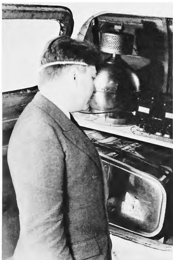
FIGURE 102.—Post views the liquid-oxygen container as stowed in the fuselage of the Winnie Mae in preparation for the long-distance stratosphere flights. Aft of the container is the Westport power supply for the radio compass. A fuselage fuel tank is mounted below the above equipment. (Courtesy Phillips Petroleum Co.)
