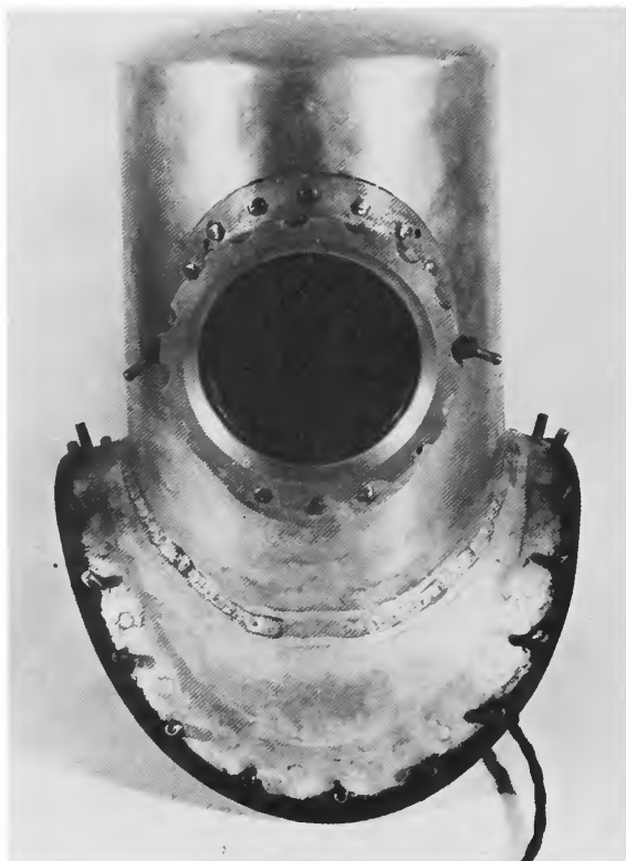
FIGURE 74.—Wiley Post's second helmet. Two inlets are located on the sides of the round faceplate. One inlet was for compressed air which originally was to be obtained from the external engine supercharger. The other inlet was for oxygen derived from a liquid-oxygen source. In practice, the oxygen source alone proved the practical approach. The faceplate could be screwed out by the gloved fingers of the pressure suit for ground- and low-altitude operations. The cord was for the headset for broadcast station tuning in relation to the radio compass. (Courtesy Phillips Petroleum Company.)
