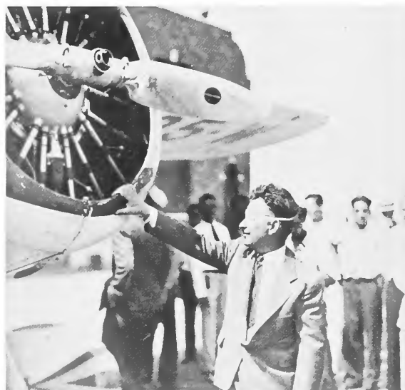
FIGURE 64.—Post examines the Winnie Mae at Floyd Bennett Airfield, New York, after completion of the 1933 solo world flight. The lower cowling reveals the dents placed there in the Flat, Alaska, nose over. The propeller is the fixed-pitch Hamilton Standard substituted at Flat for the controllable pitch propeller damaged in the nose over. (Courtesy Pratt and Whitney Aircraft.)
