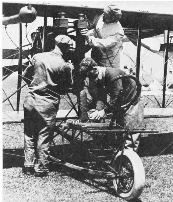
FIGURE 4.—Wiley Post's original flight inspiration, Art Smith (right top), and two assistants, prepare a Curtiss Pusher for an exhibition flight. Post saw Smith perform all types of flight aerobatics at the 1913 Lawton, Oklahoma State Fair, and was immediately enthralled. The aircraft is powered by a Kirkham water-cooled engine. The fuel tank is to the top left and the two stopcocks are in the off position. (Courtesy James R. Greenwood.)
