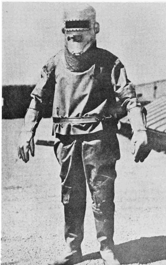
FIGURE 70.—Post’s first full pressure suit and helmet. This suit was made of rubberized parachute fabric. Earphone bulges are shown on the helmet. The rectangular plastic vision plate was replaced in the later version with a circular glass window. The metal belt sealed the top half of the suit to the bottom half, when the suit was pressurized. The suit was entered at the waist. Photograph taken on roof of B. F. Goodrich plant, Los Angeles, June 1934. (Courtesy 1935 Aircraft Year Book.)
