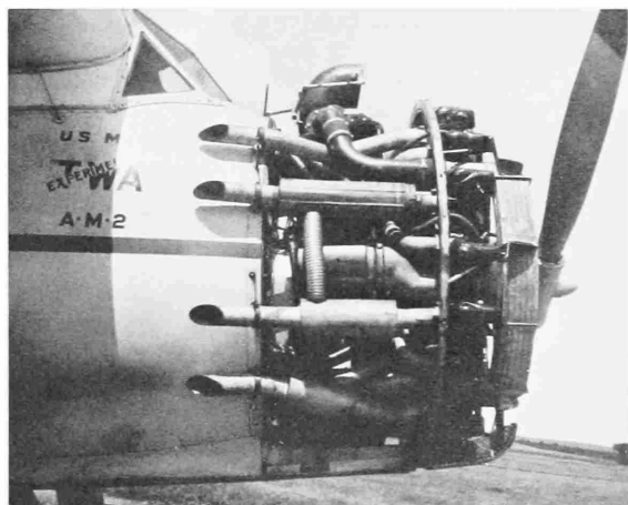
FIGURE 100.—Details are shown of the right side of the Wasp engine and the external supercharger and intercooler arrangements, plus the landing ski, as utilized for the 1935 transcontinental stratosphere flights. (Courtesy Ernest Shults.)
