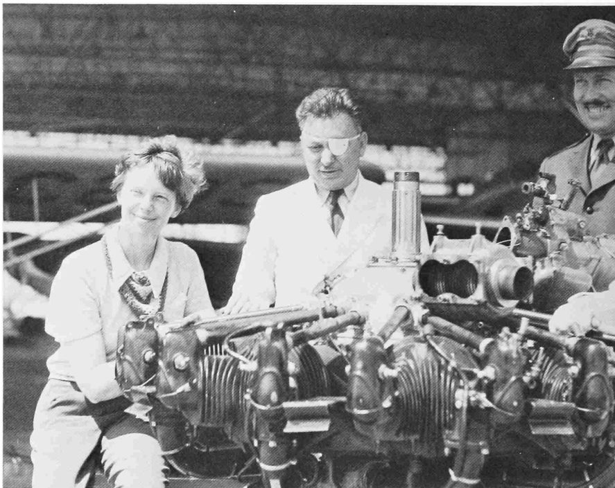
FIGURE 114.—Amelia Earhart, Wiley Post, and Roscoe Turner examine the Winnie Mae's Wasp engine during its overhaul, following the sabotage-forced landing at Muroc. On the engine in front of Turner is the carburetor and an associated heat-exchanger accessory, which enabled exhaust heat to warm the air entering the carburetor. On April 19, 1935, Amelia Earhart flew her Vega, Number NR 965 Y, from Burbank to Mexico City, in preparation for a record long-distance return flight to the United States. (Courtesy Lockheed Aircraft.)
