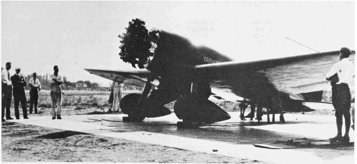
FIGURE 120.—The “Yankee Doodle,” a specially constructed Lockheed Explorer, is tested on June 3, 1930, at Los Angeles, California, during preparations for a planned Paris-to-New York, nonstop flight. Arthur Goebel hoped to fly the aircraft in the east-to-west direction, to be the first to do so. This airplane, license number NR 101 W, had a gasoline capacity of 800 gallons. Goebel did not take the plane but the Pure Oil Company did, and it set a nonstop record from New York to the Canal Zone. On November 21, 1930, the airplane was damaged in an accident at the Canal Zone and the wing was salvaged by Charles Babb. This wing was used with an Orion fuselage and became the hybrid aircraft that Post and Rogers flew to Alaska. (Courtesy Pacific and Atlantic Photos.)
