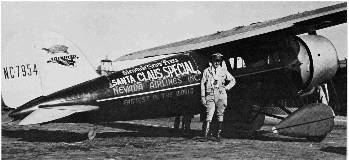
FIGURE 14.—In 1929 F. C. Hall sold the first Winnie Mae (NC 7954) back to Lockheed, who in turn sold the aircraft to Nevada Airlines. The Vega was equipped with a N.A.C.A. cowling and wheel pants, and was renamed “Sirius.” “Captain” Roscoe Turner (later “Colonel”) flew the aircraft in the 1929 air races, coming in third in the free-for-all speed contest, at an average speed of 163.44 miles-per-hour (mph), behind Doug Davis, first, (194.90 mph in a Travel Air) and R. G. Breen, second, (186.84 mph in a Curtiss P-3-A). (Courtesy Lockheed Aircraft Company.)
