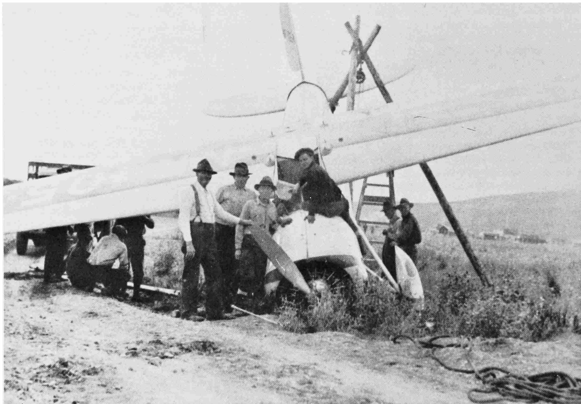
FIGURE 60.—The Winnie Mae has nosed over on July 20, 1933, Flat, Alaska, after a long nonstop leg from Khabarovsk, Siberia. A block and tackle was erected to lower the tail. (Courtesy Stephen E. Mills.)
