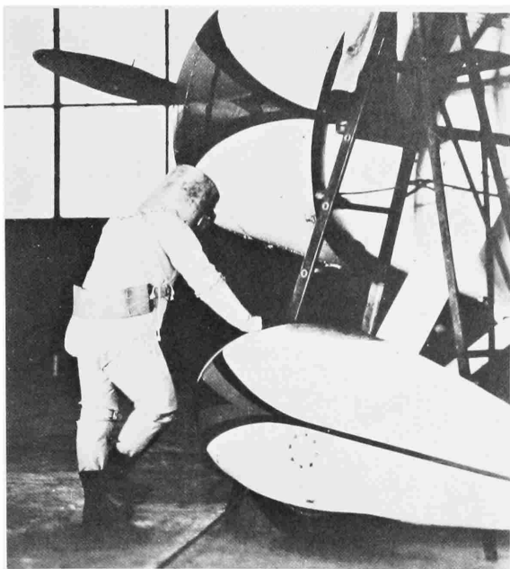
FIGURE 83.—Post prepares to climb ladder to enter Winnie Mae . Note the broad-banded strap which Post sat on. The strap, through its connections with criss-crossing cords to the helmet, kept the helmet from rising excessively during inflation. (Courtesy Phillips Petroleum.)
