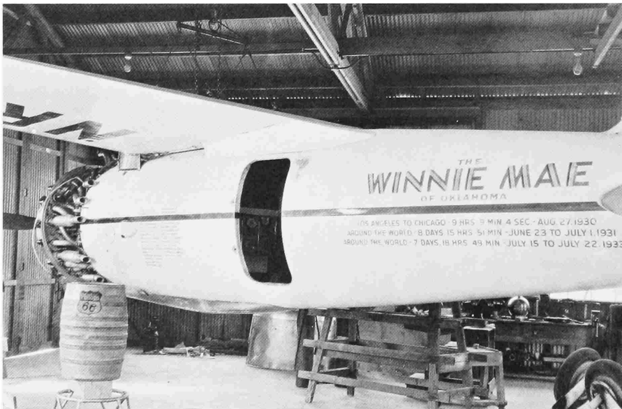
FIGURE 96. —The Winnie Mae is shown being prepared for a transcontinental stratosphere flight. This photograph was made in January 1935 at the original Lockheed hangar in Burbank. This hangar had been a "glass factory" prior to its use by Lockheed. The cowling has been removed and cleaned of paint (seen on floor behind fuselage). The aircraft is suspended by pullies from a ceiling beam by utilizing the hoist eye hooks on the upper wing. The belly-landing skid made of spruce has been glued in place and is now metal clad. Under the rear fuselage in the background on the workbench is the spherical container for the liquid oxygen. (Courtesy Phillips Petroleum.)
