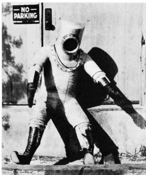
FIGURE 113.—A static pressure test is accomplished with Post's perfected flight-pressure suit after the Muroc forced landing, February 1935. Note the seat-belt marks above the thigh area and the outlet for the headset wire, just beneath the left, lower visor. (Courtesy Edwin O. Cooper.)
